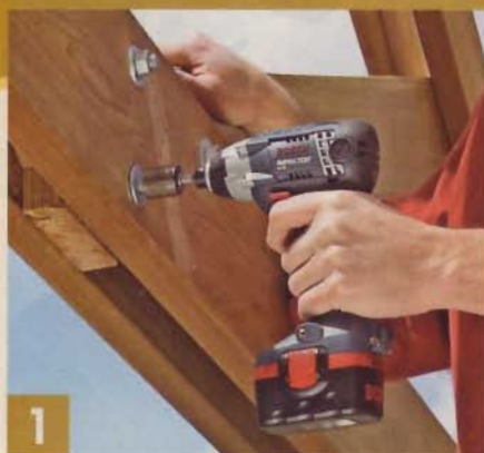
▲ The high torque generated by an impact driver is great for big fasteners, such as lag screws and bolts.
