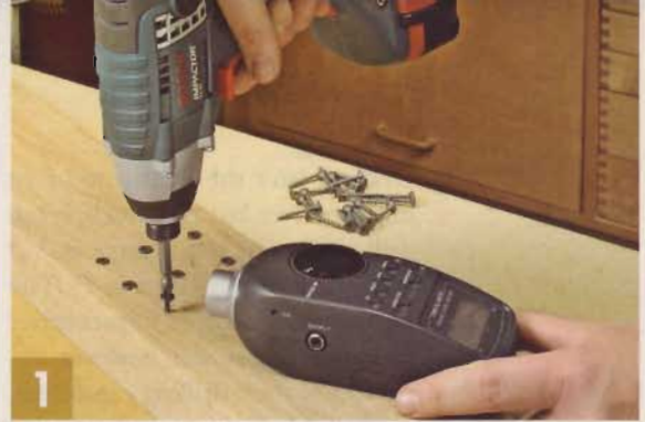
▲ The ratcheting action that helps an impact driver create high torque also makes it very noisy. We used a decibel meter to see just how noisy each tool was.
