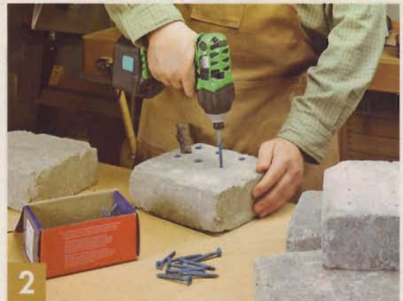
▲ Driving masonry screws into concrete is just one of many applications at which an impact driver excels. We drove a bunch to see which drivers were fastest.
