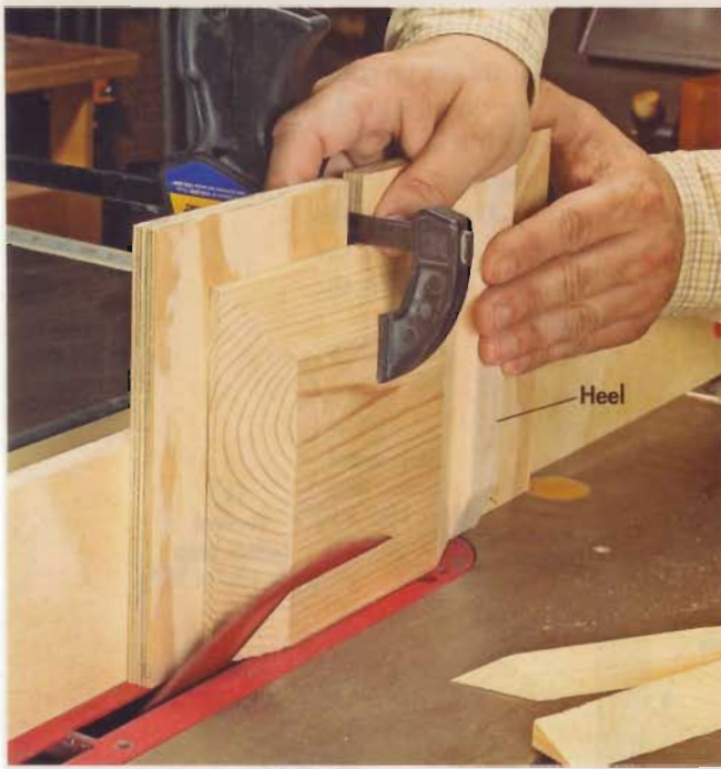
▲ A simple jig makes beveling the post cap tops easy. It's just a piece of 1/2" plywood with a "heel" attached. A tall auxiliary fence supports the jig.
