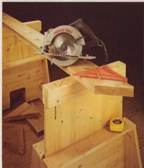
▲ The tops of sawhorses always get chewed up when sawing boards. But replaceable "saddles" protect the adjustable panels on these horses.
