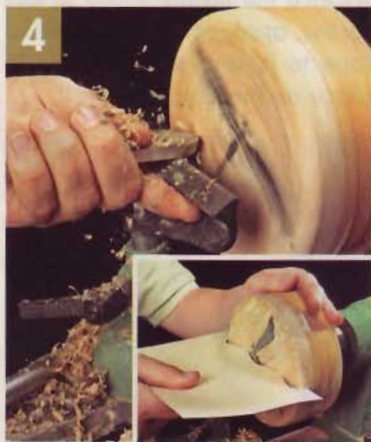
▲ A round-nose scraper makes quick work of the lid profile. Work from the outside in, and check your work with a cardboard template.
