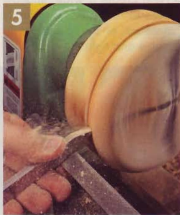
▲ Use a parting tool to cut a 1/4" x 1/4" rabbet along the bottom edge of the lid. This rabbet forms a lip that fits in the top of the box.
