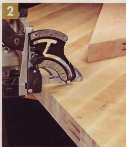
▲ Two rows of #20 biscuits help align the mating edges of the tops. Cut slots for the biscuits \frac{1}{2} " from each face and between the fastener locations.
