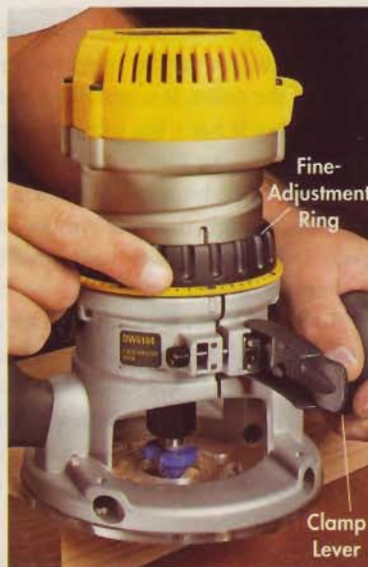
Rotating Ring. Turning this large ring allows fine adjustment. A scale on the base shows the resulting depth change.
