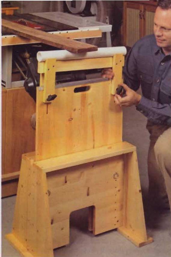
▲The outfeed support lends a helping hand when working with long stock. It mounts to the adjustable panel and can be set to the exact height you need.
