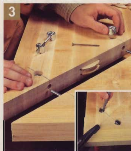
▲ After boring holes for the fasteners, dry-fit the slabs to make sure they draw together tightly. A large nail or nail set is used to tighten the fasteners ( Inset ).
