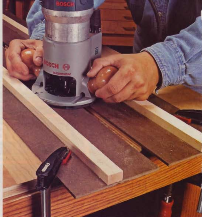
▲ These edge guides make it easy to rout tight-fitting dados for plywood using a standard straight bit.
