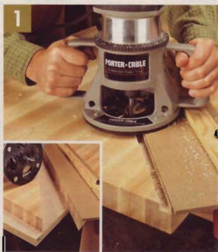
▲ After laying out the miter angle, clamp an edge guide in place to guide the router. Make \frac{1}{4} " deep passes, holding the router tightly against the guide fence.
