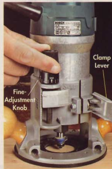
Micro-Adjust Knob. A threaded rod connected to this small knob rotates to make small depth adjustments.
