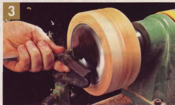
▲ To remove the paper and epoxy residue, as well as flatten the lid, move the tool rest to the front, and work your way from the outside to the center, making cuts along the piece with a square-end scraper.
