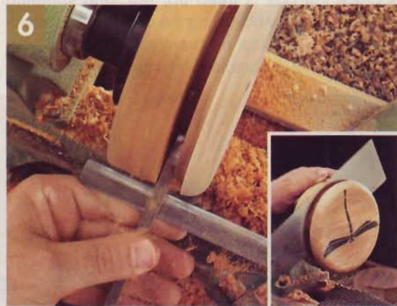
▲ To separate the lid blank from the glue block, use a parting tool to cut down the "glue block" side of the joint line. Cut into the block until the lid is almost separated, then use a handsaw to complete the job.
