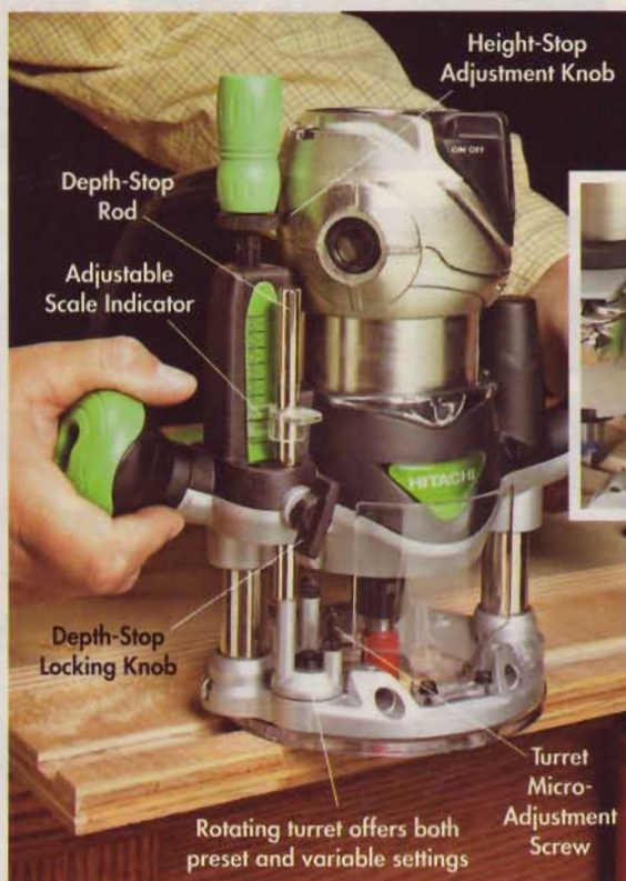
Multiple Stops. The depth stops on a plunge router make it easy to set cutting depth exactly. And they offer repeatability from cut to cut and workpiece to workpiece.
