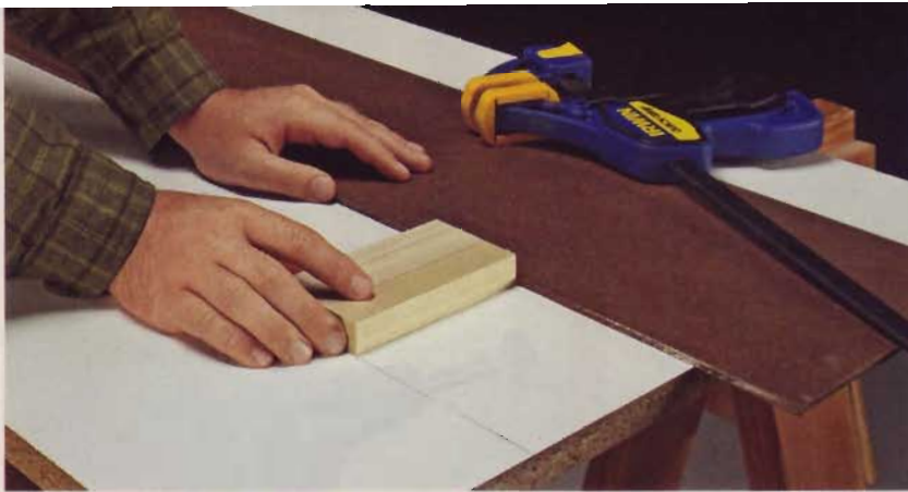
To make straight cuts, guide the circular saw with a straightedge. A setup block makes it simple to position your straightedge the proper distance from the cutline.
