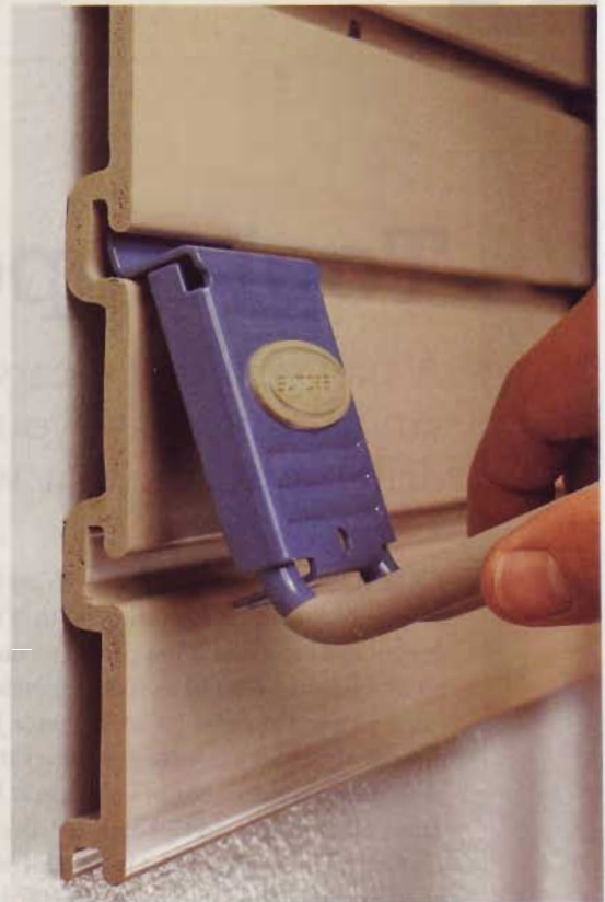
To install an accessory, slide it along a groove until you find the right position. Lock it in place with tabs that engage two of the grooves.
