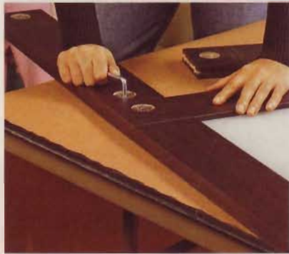
2] Apply glue to the door joint, slide the stile into place, and then use a wrench (included with the kit) to tighten the cams.
