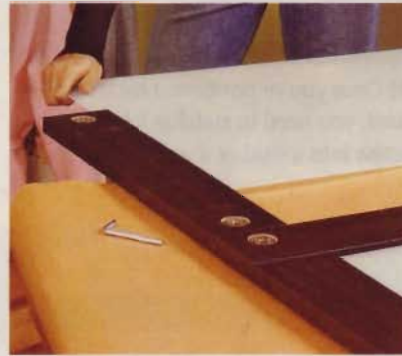
3] Slide the glass panel into the grooves in the stiles, and then attach the last panel to complete each door.
