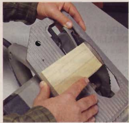
The setup block matches the distance from the blade to the edge of the base.
