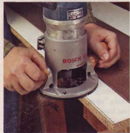
Nothing can produce a smoother, cleaner edge on a sheet of melamine than a router and a straight bit.
