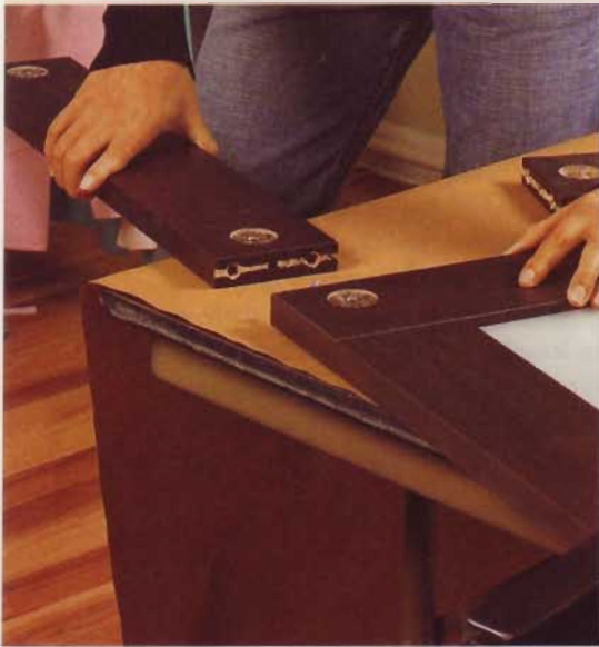
1] To attach the stiles, insert locking cams in the pre-drilled holes. Then slide the stile into position to test the fit.
