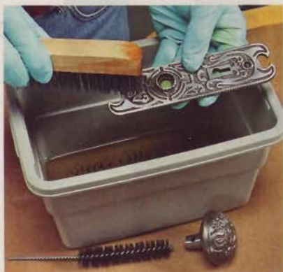
1] To get the powder to adhere properly, scrub all the finish off the hardware using lacquer thinner and a wire brush.
