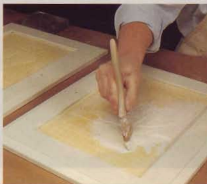
8] With the design complete, coat it with the same paint used for the base coat. A brush helps fill small cracks and crevices.
