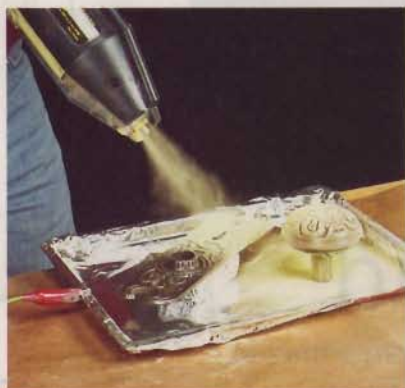
3] After charging the tray, spray the powder across the pieces until they're completely covered.
