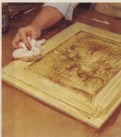
10] Wad up a ball of cheesecloth, and dab the glaze lightly to remove brush strokes and create a mottled appearance.
