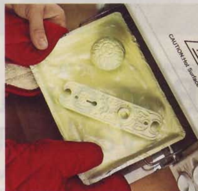
4] Bake the hardware at the desired time and temperature to get the powder to melt and fuse to the metal.
