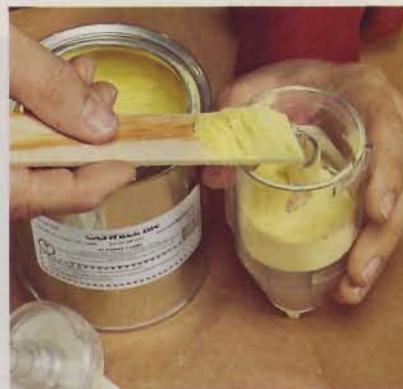
2] Remove the cartridge from the tool, and load it with the colored powder. Any powder that's not used is reusable.
