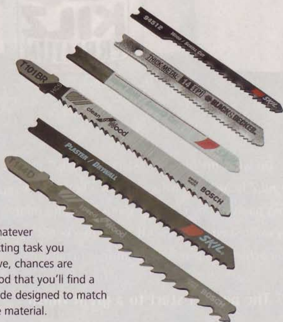
When selecting jig saw blades, pay attention to how many teeth per inch (tpi) the blade has. A low tpi yields a rough but fast cut. A high tpi produces a smooth, slow cut.
