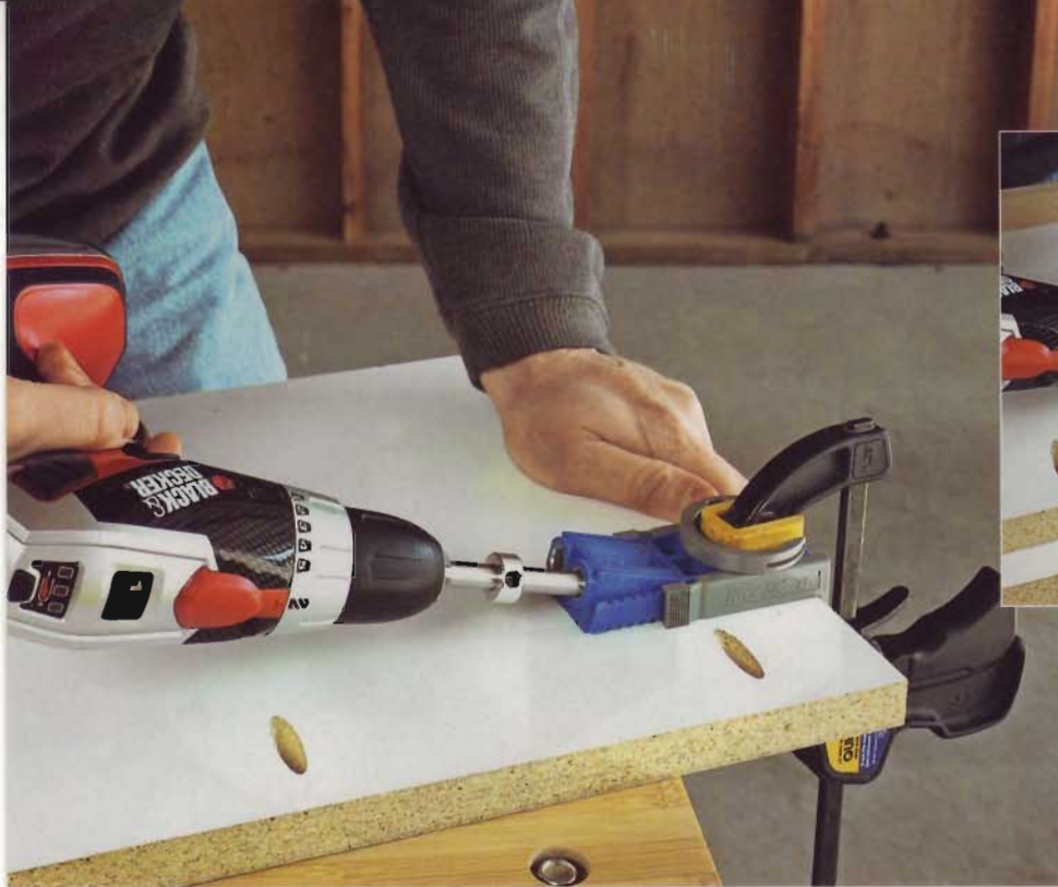
Use a pocket-hole jig to bore holes in the underside of the tray bottom (above). Then position the tray bottom using a spacer, and drive screws to attach the sides (Inset).
