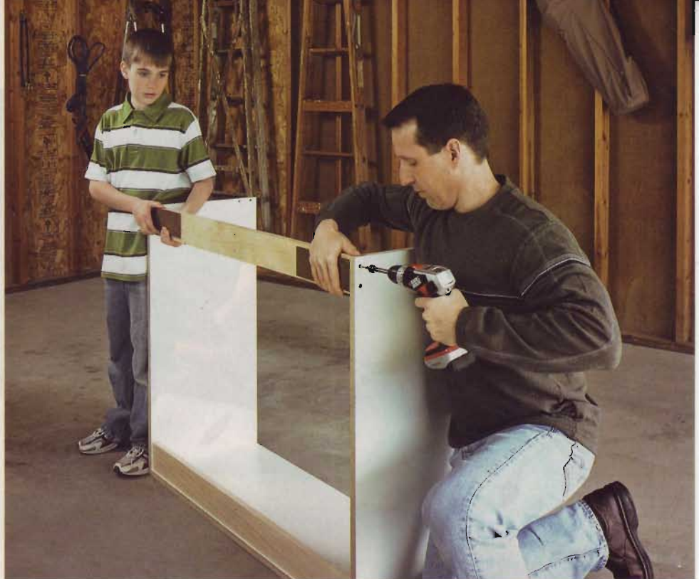
Use spacers to position the upper rear stretcher, and have your helper hold one end of the stretcher in place as you align the other end and drill screw holes.
