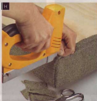
Trim, fold, tuck, and staple the fabric so the opening faces the side of the cushion.
