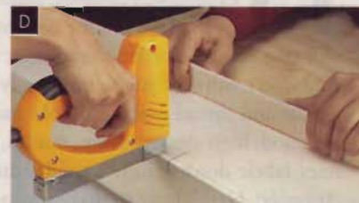
Fold excess muslin around a ruler, have a helper pull to apply tension, align a pencil line with the layout line, and staple.
