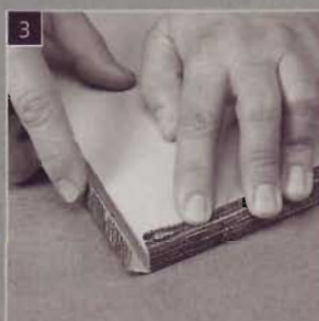
3 After attaching the grasscloth to the MDF panels, carefully wrap the edges.
