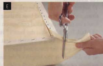
Cut off some of the excess muslin to remove material that would create a bulge in the finished corners.
