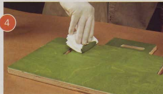
4 Remove the excess stain using a clean, soft cloth lightly dampened with stain. Wipe in the direction of the wood grain, and use light to medium pressure for even color.
