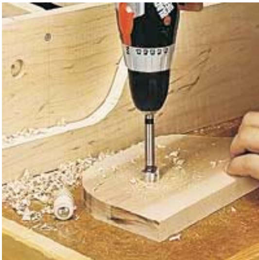
FIGURE 3 Remove the pivoting arm. Now drill a countersink on the outside of the case at the location you just drilled the \frac{1}{16} " hole. Drill the matching countersink in the pivoting arm. The countersinks need to be \frac{3}{4} " diameter and \frac{9}{16} " deep. Glue the hinge into the counterbores.
