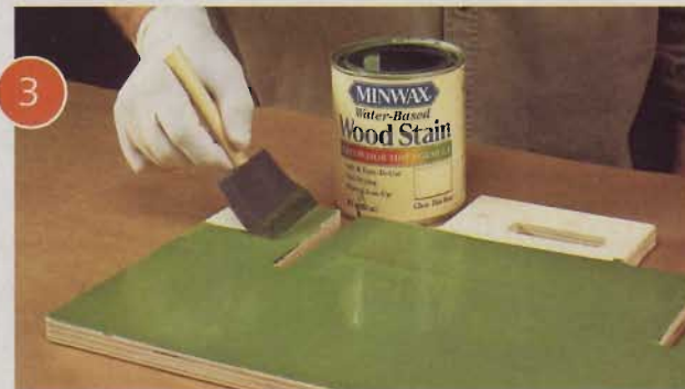
3 Use a foam brush, staining pad, or synthetic bristle brush to apply the stain in the direction of the wood grain. Don't let the stain penetrate longer than 3 minutes.
