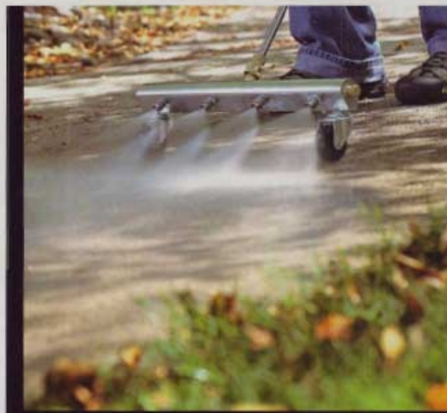
Rinse a big area quickly by attaching a water broom to your pressure washer.
