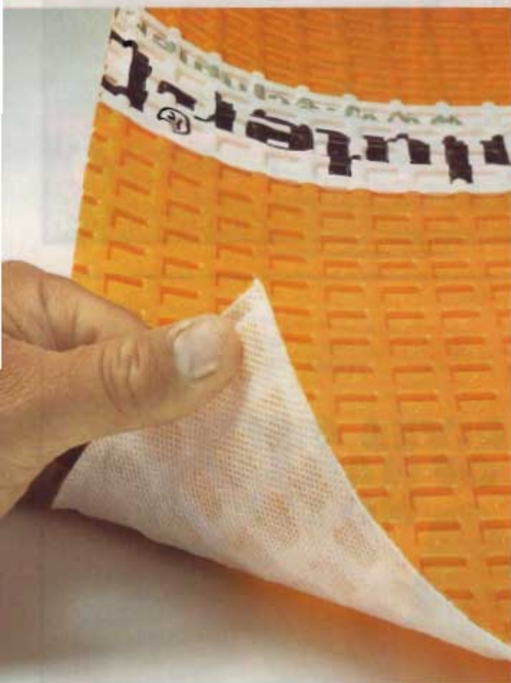
Fleece on the underside of Ditra wicks away moisture. A waffle pattern on top holds mortar to create a solid structure.
