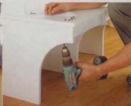
2] With the base sitting away from the wall, set the locker unit on the base. Align the seat panel, making sure that it sits flush or overhangs where necessary (left). Then drive pocket screws that secure the locker unit to the base (right).
