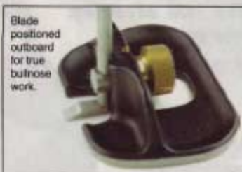
Base registers easily off end of workpiece.
