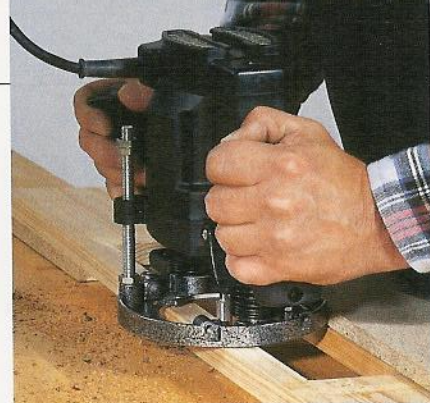
Scrap wood clamped to the workpiece serves as a straightedge guide for the router to follow. This router's base plate has one flat edge to help guide.
