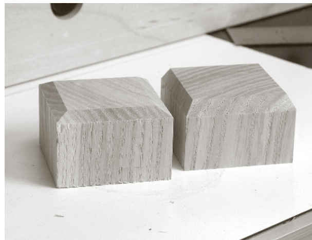
Profiles of chamfers made using router bit angles other than 45° differ depending on whether the leg stock is run vertical or flat to the table. Here you can see the different chamfers that were cut with a 30° chamfer bit.
