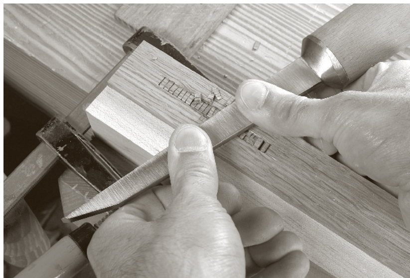
This through-mortise on the lower leg of a Gustav Stickley rocker would not pass modern muster. The ends of the mortise were left round and the tenon was square. On other joints in this chair you can see tearing left from the boring machine.
