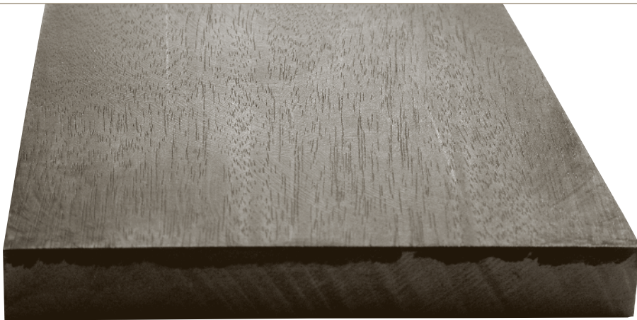
Water-based filler dries very quickly. Here you can see swirls from the application of the product. Make sure to wipe excess water-based filler from the project while moving with the direction of the grain.
