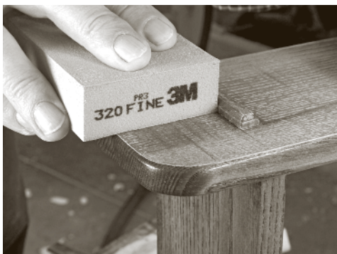
Sponges are also good for getting at both sides of an inside corner.
