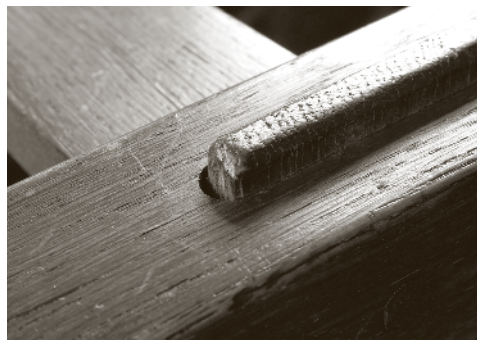
This through-mortise on the lower leg of a Gustav Stickley rocker would not pass modern muster. The ends of the mortise were left round and the tenon was square. On other joints in this chair you can see tearing left from the boring machine.
