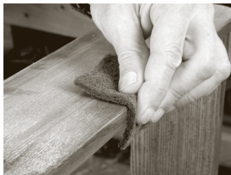
A nylon pad and a gentle touch can sand an outside corner without going too far.
