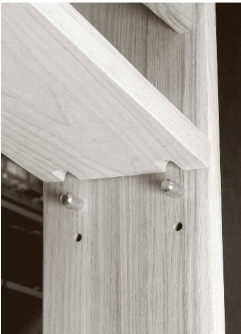
Stopped grooves made at the router table with a core box bit hold the shelves securely and conceal the shelf pins.
