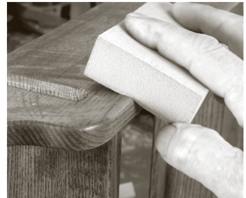
Sanding sponges are an excellent balance of a flat surface that gives enough to gently handle corners and edges.
