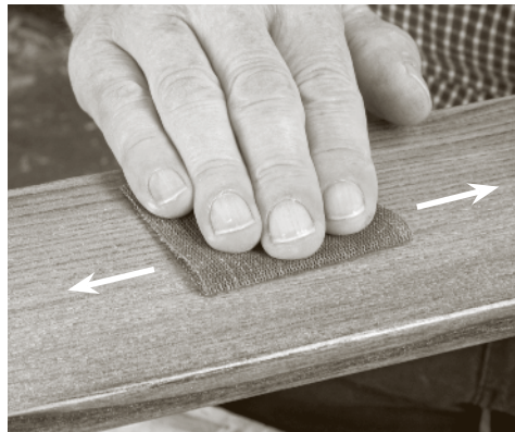
On flat surfaces, grain direction does not matter, but it is important to move at a right angle to the direction of your fingers. Going the same way can produce grooves in the surface.
