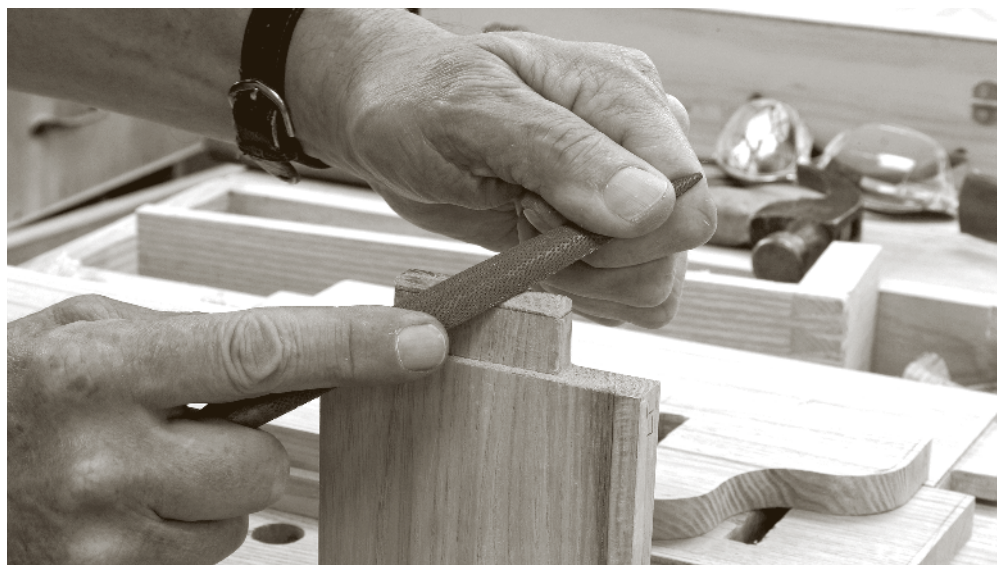
Holding the rasp at a 45° angle quickly brings the chamfered ends down to the layout line.
