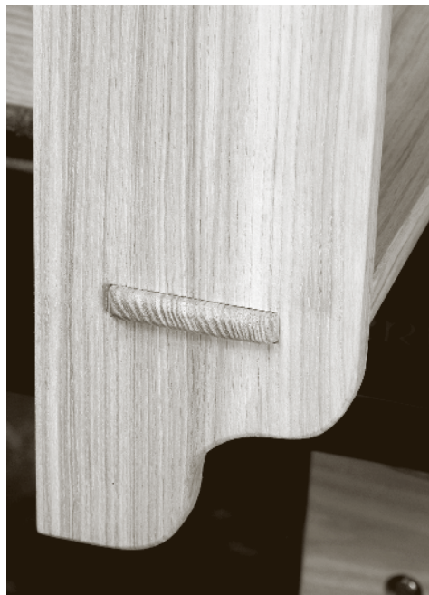
The completed through mortise-and-tenon joint is incredibly strong, and it adds a decorative accent to a simple project.
