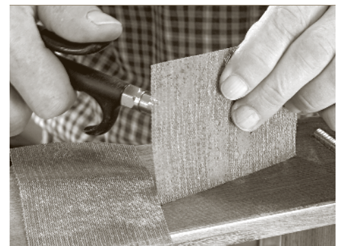
Abranet is mesh, so dust has a place to go. If it clogs, it can be cleaned with a blast of air.
