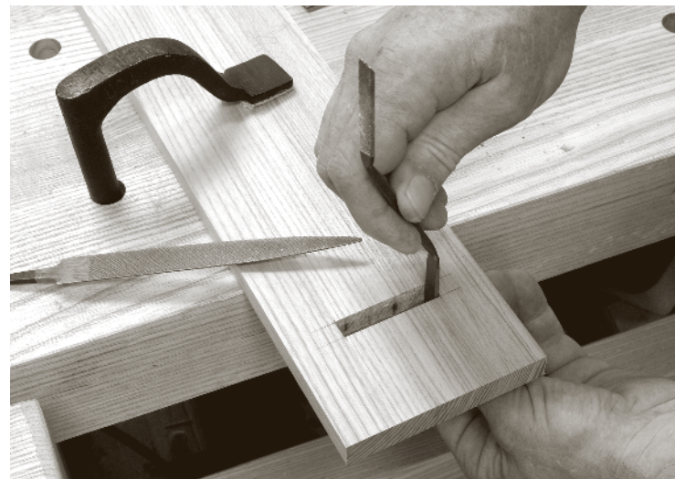
A small flat file is ideal for perfecting the ends of through-mortises.
