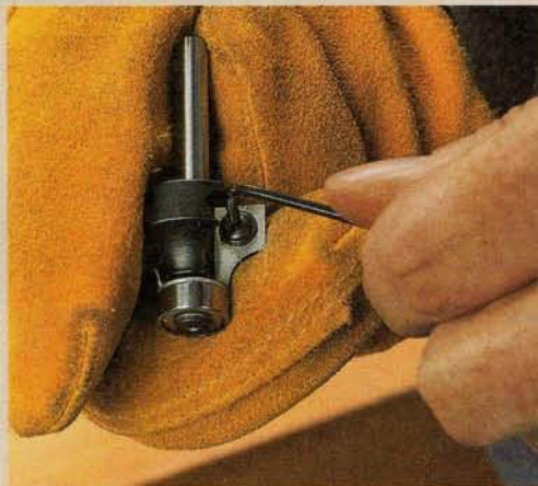
▲ To protect your fingers, it's a good idea to wear a leather glove while rotating or replacing the carbide cutters.
