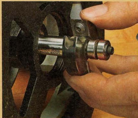
▲ The 1/2"-shank bits offer the convenience of replaceable inserts but with heavier-duty construction.
