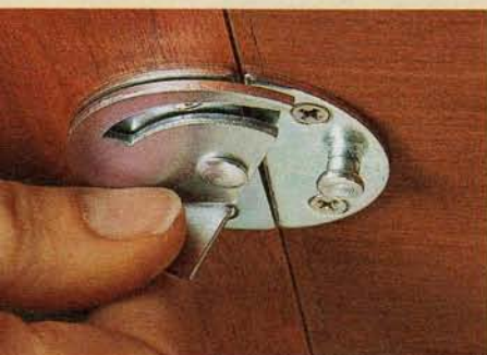
▲ Installing locks between the top and the leaves keeps them from separating when in use.
