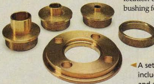
▲ A guide bushing attached to the baseplate follows the fingers of the template in a dovetail jig for perfect dovetails every time.
