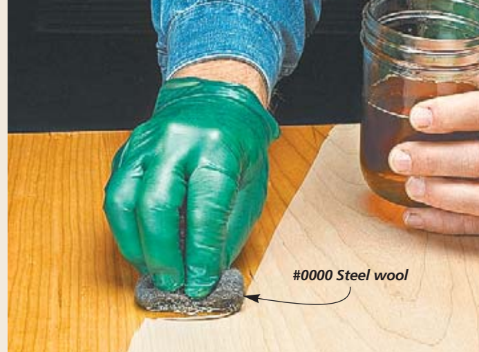
▲ A jar of oil and a pad of steel wool are all you need to get started. Wipe on a heavy coat and let it soak in.
