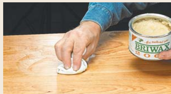
▲ A light coat of paste wax goes on over the third coat of oil. A soft cloth and a circular motion do the job.
