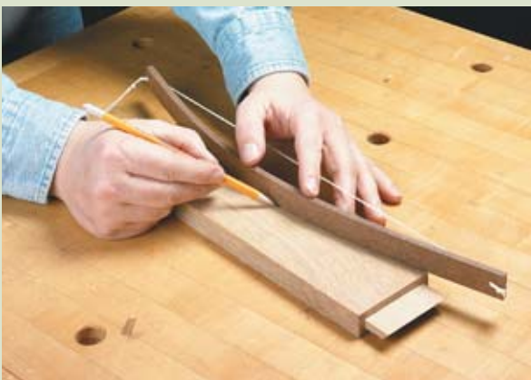
▲ A notched scrap of hardboard and a short length of string is all you need to lay out a smooth, consistent curve. A series of knots tied in one end of the string allows you to easily adjust the amount of "bow."
