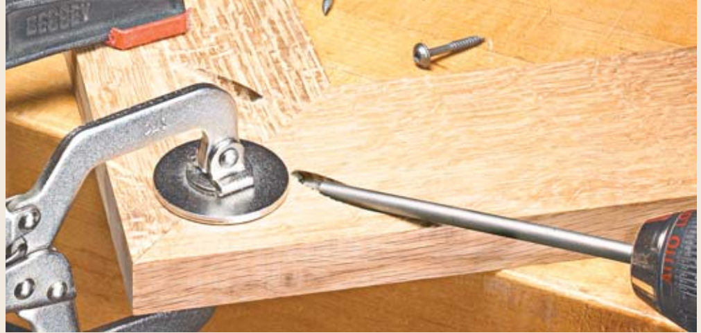
▲ Two pocket holes square to the miter joint and opposite one another allows pocket hole screws to secure the miter joint. A face frame clamp makes it easy to hold the joint in position while the screws are inserted.
