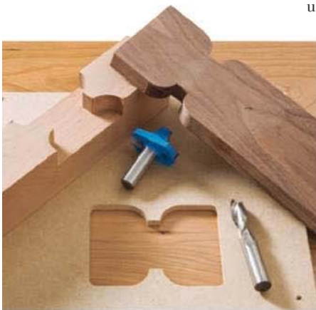
Supplies for Scott's Butterfly Joint: 1/2" straight spiral bit, 5/8" roundover and Scott's template.
