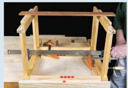
The second jig has buttresses positioned to hold the end frames and the top rail. To prevent the frames from falling over during clamping, a brace with retaining blocks is placed across the top of the subassembly.
