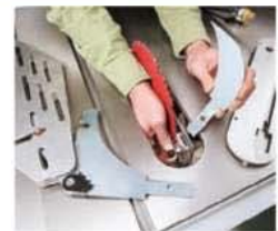
You can just about split hairs with the T-square style rip fences on these big saws, making ripping extremely precise (top right photo). A quick-release knob simplifies changeovers on General's riving knife and guard system (right).
