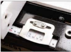
Grizzly's hairline fence cursor (left) makes it easier to read rip fence settings without parallax discrepancies. A handy cleanout door around the dust port (inset) simplifies cleanout chores.
