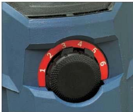
The rpm control dial is located on the front of the router and is very easy to read. It would be great if Bosch would provide a chart relating numbers to rpm.
