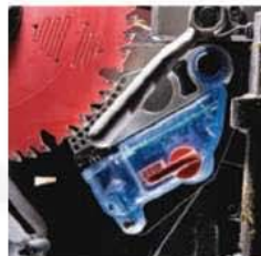
SawStop's revolutionary blade brake (inset) offers industry-leading safety, and the dust-collecting guard (left) promotes cleaner sawing in general.
