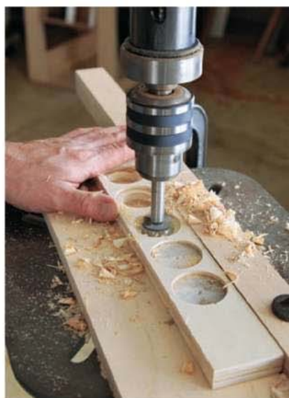
Drilling the two-step borings in the top pieces of the tool holders is most easily completed on a drill press. It can be done with a handheld drill, but it's just a bit trickier.
