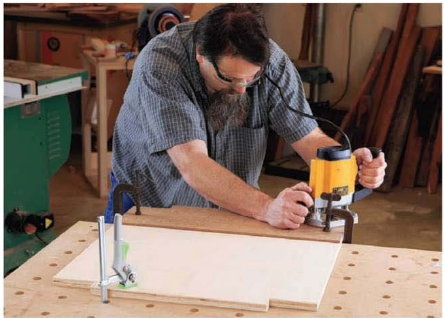
After roughing out the notches on the inner panels, the author pattern-routed the final shape with a 1/2"-diameter pattern routing bit. Its radius perfectly matched the 1/4" roundover bit used on the legs.
