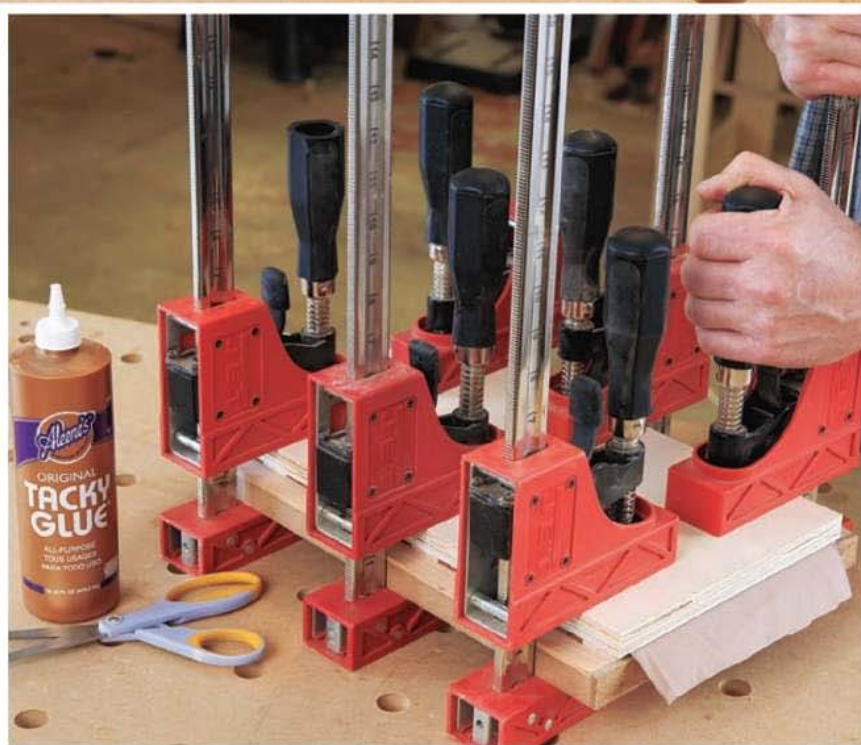
Once the pieces are lined up in the jig, the author draws a line along each edge (top photo). Both the canvas and glue are kept well out of that area (where the door rides in its grooves). The canvas is then applied (bottom photo) with the help of a flat board, wax paper (not seen) and plenty of clamps.
