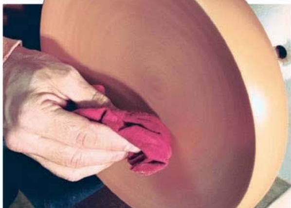
The author applies his liquid friction polish to a spinning maple bowl. As the friction spreads and polishes the product, a smooth, shiny finish begins to appear.
