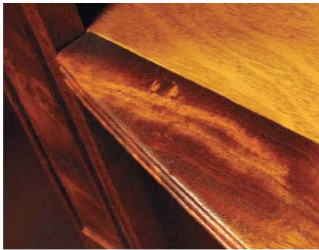
The hardwood on the face of this bookcase is mahogany. So is the plywood shelf to which it is glued. They're stained with the same product, but the look is dramatically different.
