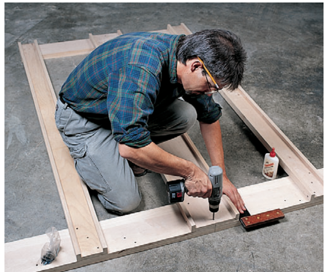
Figure 1: When working on larger assemblies like this panel saw, keep an accurate square handy as you glue and screw each piece together.
