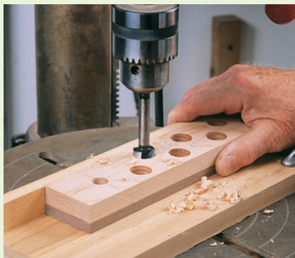
Step 1: Glue up two pieces of 5/8" maple for the jaw tops and a piece of 5/8" maple and 3/8" walnut for the bottoms. Use the full size pattern on the Pinup Shop Drawings to lay out holes for the magnets and spindle nuts, and a Forstner bit to complete the drilling.
