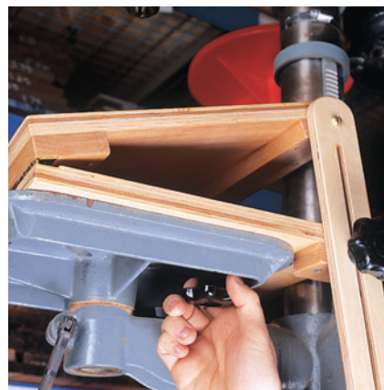
Step 6: Bolt the adjusters to the upper plate assembly and clamp them to the screw blocks with knobs. Use the remaining two knobs to secure the jig to your drill press table.
