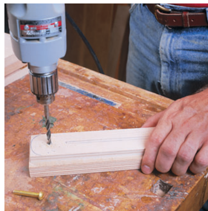
Step 3: Cut plywood for the adjusters and lay out the pivot hole and slot on each one. Drill the 1/4" pivot holes.
