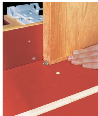
Figure 3: Rout the grooves in the drawer sides after the units are assembled. Be sure to stop the grooves 1/2" from the face of the drawers.
