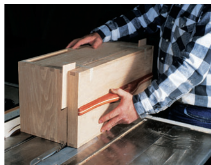
Figure 2: Cut three sides of the box to separate the lid, then slip 1/8" thick shims into the kerfs, holding them in position with masking tape to make the final pass.
