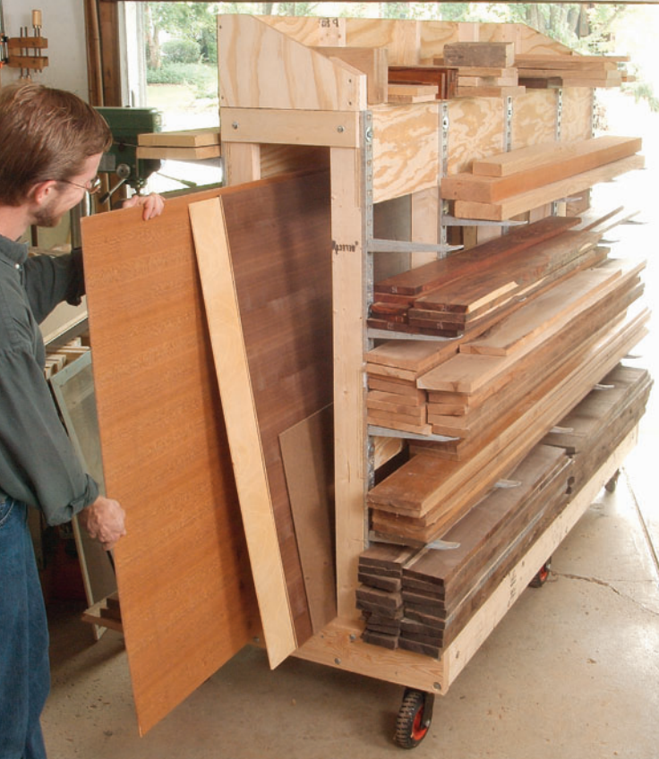
The author maximizes floor space in his cramped garage shop with the help of a two-sided, rolling lumber cart that also stores sheet goods and shorter offcuts in separate bins.
