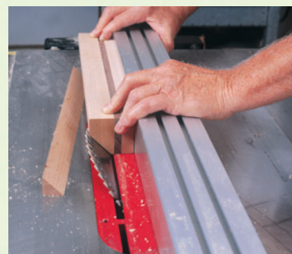
Step 4: Transfer the end view of each jaw to your workpiece and cut the 45° angles on the tops with the magnets riding along the rip fence. Switch to a router with a 1/2" roundover bit to soften the top edges and ends of each of the jaws.
