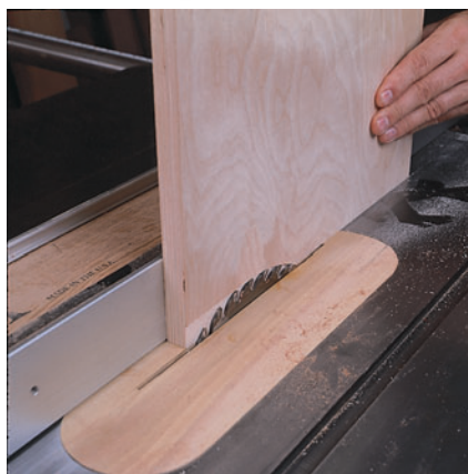
Step 1: Cut stock to size and rabbet the lower plate and one strip to accommodate the hinges (see Hinge Detail ). Fasten the hardwood to the plates and install the hinges.
