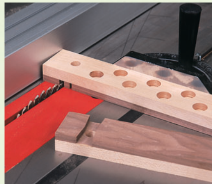
Step 2: Set the miter fence to about 5° when defining the walls of the spindle tracks (see full size pattern). This shape will keep the track a little wider at the edges than in the middle and help to prevent binding during use.
