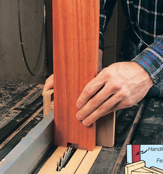
Figure 1: Make the jig at right to wrap your table saw fence and stabilize the tall handle blank during the joint-cutting operation. To limit the chance of making a mistake during cutting, shade in the waste area first with a pencil.
