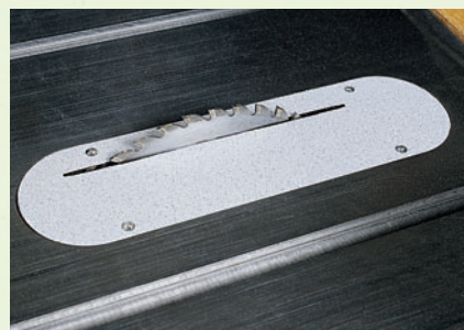
A zero-clearance insert is the real key to creating clean, chip-free edges when cutting melamine-coated materials on a table saw.
