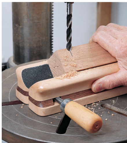
Drilling into edges and corners is easy with this magnetic V-block jig. The jaws can be opened to suit tapered or parallel edges, and no-skid paper holds spindles firmly in place.
