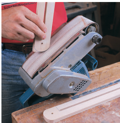
Step 5: Secure your belt sander in a vise and shape the ends of the adjusters. Use a palm sander to smooth the jig's surfaces and ease all the corners. Apply a coat of sanding sealer.
