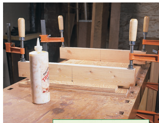
Figure 1: Batten boards, which feature a curve of about 1/8 inch on their bottom edge, are used to apply pressure at the middle of a wide panel assembly during glue-up to hold it flat.
