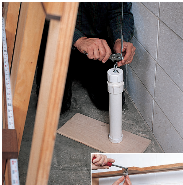
Figure 4: After installing the pulley (inset), set the counterweight on a spacer and, with the saw at its highest position, attach the cable. Adjust the counterweight to equal the weight of the saw and carriage.
