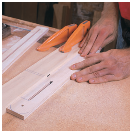
Step 4: Rout the slots in shallow passes with a 1/4" straight bit after marking the bit's cutting area on the fence. Use the marks as guides for starting and stopping the cuts.
