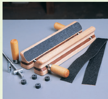
Step 6: Glue the biscuits in place and insert the two nuts. Apply the no-skid tape and trim the excess. Sand thoroughly and apply a few coats of finish over everything, including the tape. Wrap up by inserting the spindles and the two handles.
