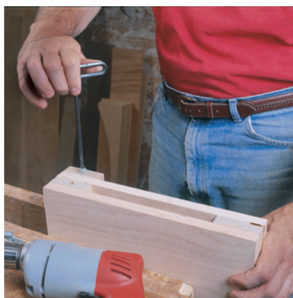
Step 2: Drill pilot holes for the threaded inserts in the ends of the strips and screw blocks, and in the bottom plate. Wax the inserts and install them with a hex driver.
