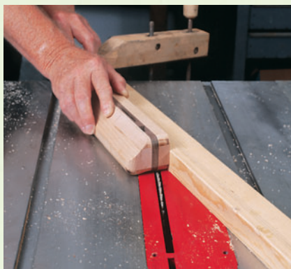
Step 5: Clamp an auxiliary fence at an angle to the table saw top and use scrap wood to establish the angle for the cove cut before cutting your project parts. To determine the exact fence angle, try raising the blade and sighting down the end of the blocks.
