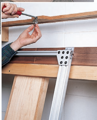
Figure 4: After installing the pulley (inset), set the counterweight on a spacer and, with the saw at its highest position, attach the cable. Adjust the counterweight to equal the weight of the saw and carriage.
