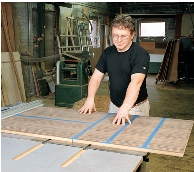
In the busy shop of contributing editor Mike McGlynn, sheet goods get knocked down to size using a commercial panel saw and the table saw soon after entering the shop. Smaller panels are easier for him to manage alone, which saves effort and leads to more efficient work.
