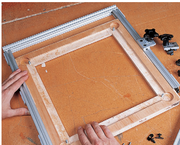
Figure 3: The plywood carriage insert fits a traveling aluminum frame. In turn, the saw is mounted to a Plexiglas plate, which is attached to the insert with threaded knobs.
