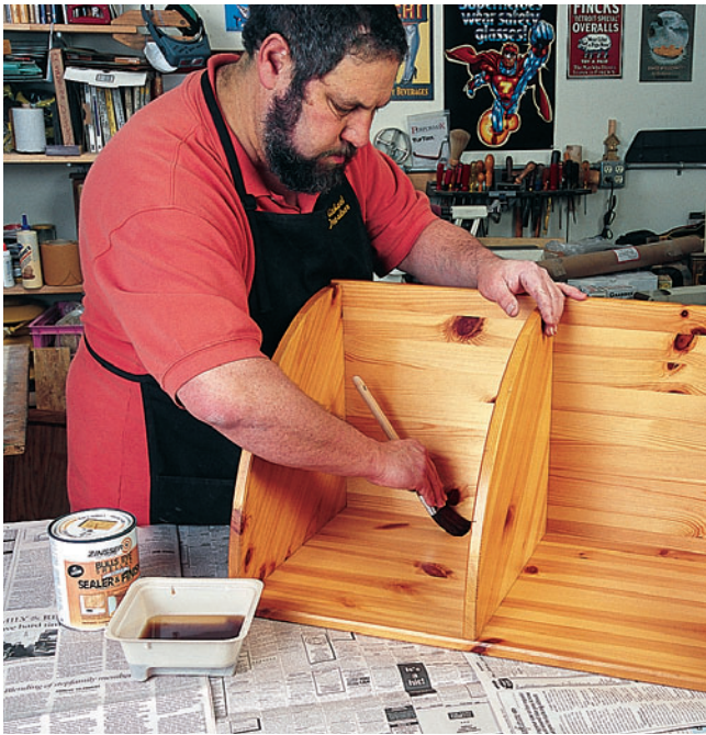
Finishing guru Michael Dresdner maintains a separate clean area of his shop for applying finish. Not only does he get dust-free results this way, but it also allows him to keep finishing supplies, applicators and other cleaning solvents all within easy reach of the bench.
