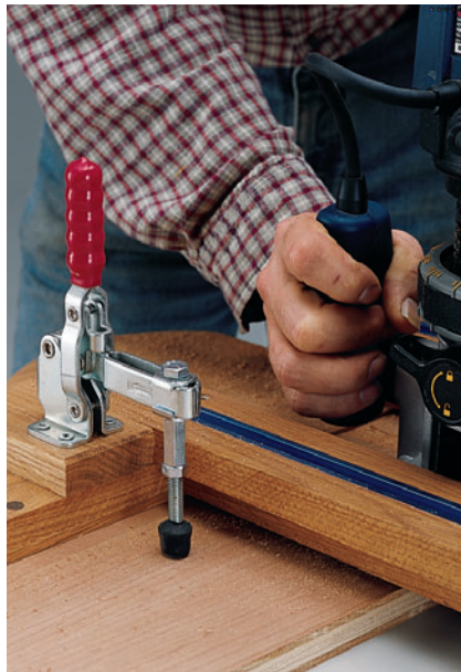
Figure 3: The hold-down clamp is mounted on a spacer block and modified with a 1"-long hex head bolt and a connector nut.
