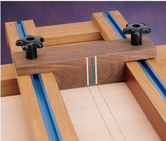
Figure 2: Attach the rails to the melamine deck with screws and glue. Cover the exposed screw holes with walnut plugs.
