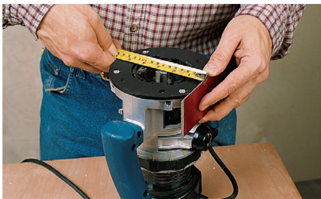
Figure 1: Determining the space required for your router is critical to the success of this jig. Measure your router and the two pieces of laminate to get the exact dimension.
