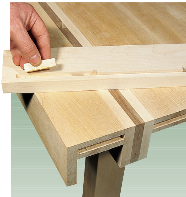
Figure 1: The spline grooves on the endcap are stopped, while those on the ends of the top are through cuts. After routing the grooves in the top, a three-inch-wide strip is ripped off. This piece sits outside of the liners and spacers.
