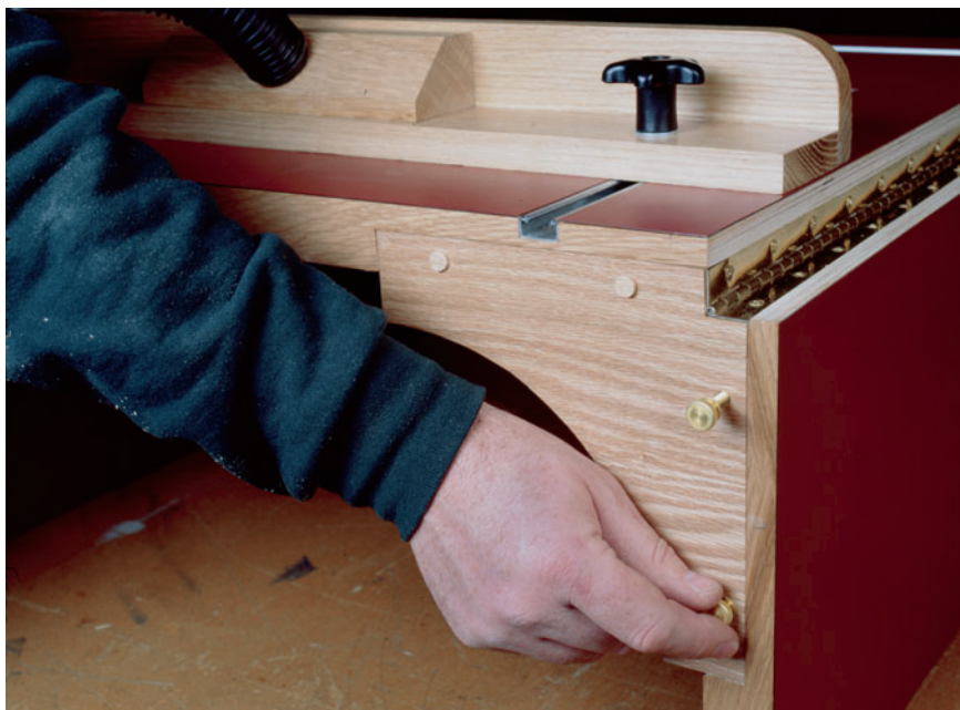
Figure 2: Gussets that are mortised into the back of the tabletop allow the top to be converted into a portable benchtop unit.
