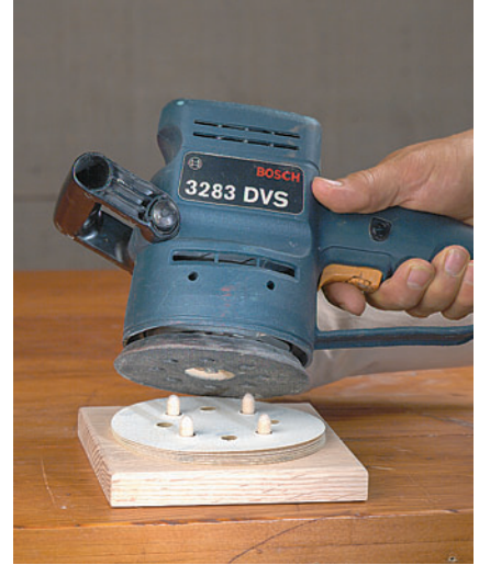
The alignment blocks don't just store the disks, they make it easy to center them on your orbital sander: just press down. The dust extraction holes line up every time.
