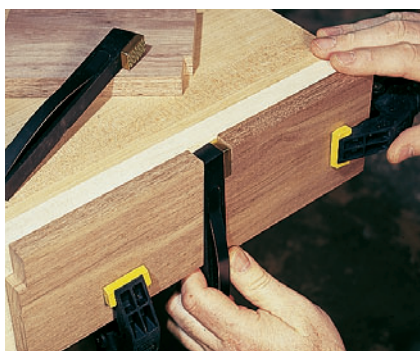
Figure 2: Dry-fit the bench dogs and spacers, leaving gaps that are the size recommended by the dogs' manufacturer. When everything fits, trim the final spacer to length.
