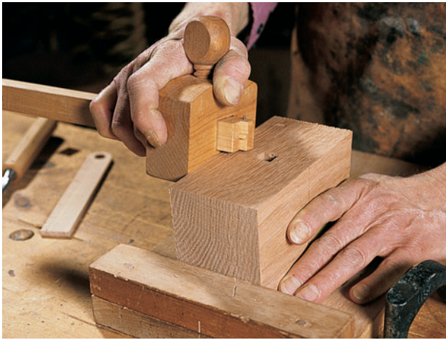
Step 2: The dovetails are half as deep at the top of the mallet head as they are at the bottom (where the handle enters). Scribe the depths with a marking gauge.
