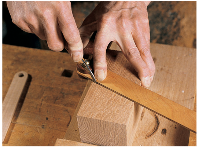
Step 3: Connect the scribe marks with a reliable straightedge and a sharp marking knife to ensure precise layout lines.
