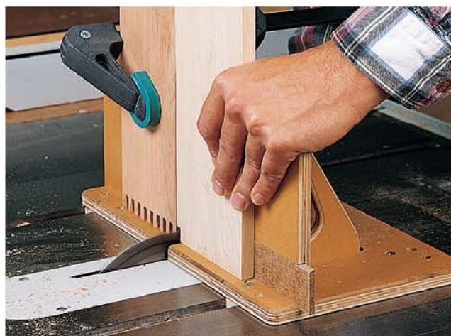
Jigs can serve a transformational purpose for shop machines. Equipped with a finger joint jig and dado blade, a table saw becomes a precise and efficient joint-making machine.
