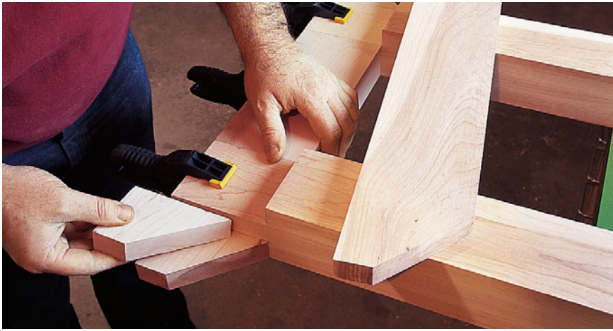
Figure 4: Dry-fit the legset parts together, then use this as a template to determine the shape of the foot and top inserts.
