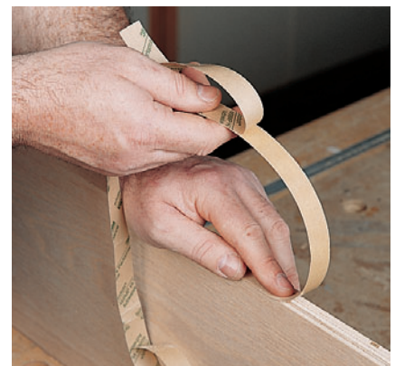
Figure 3: Apply pressure sensitive hardwood tape to all four edges of the base unit's plywood doors, then sand the tape flush. Sand carefully to keep from sanding off the plywood surface veneer.
