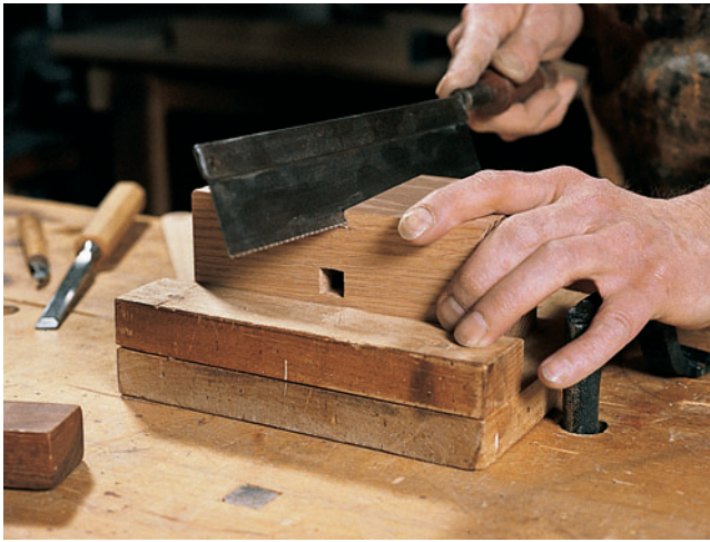
Step 4: Saw the sides of the dovetail slots with a backsaw. Slice kerfs in the slot's middle to help you gauge the depth when paring.
