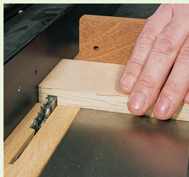
Step 2: Without moving the rip fence, switch to the miter fence to form matching dados in the drawer sides.
