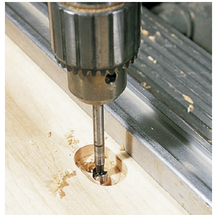
Figure 3: Use your drill press to bore two-step slotted holes in the endcaps: these will allow the benchtop to adjust to various levels of moisture in the workshop.
