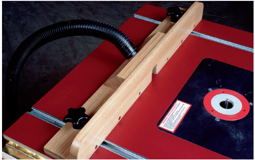
Figure 4: The router table's fence incorporates a dust collection port. Your shop vac hose should friction-fit to this hole.
