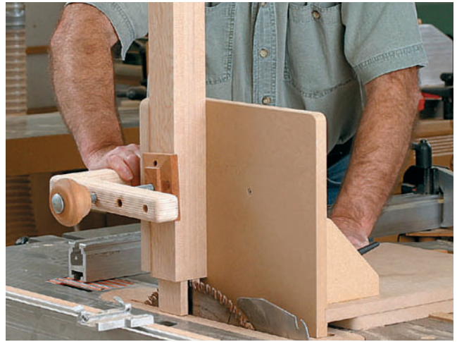
A shop-made tenoning jig offers multiple advantages: it stabilizes end cuts on long workpieces, improves accuracy and keeps your hands out of harm's way. Nothing makes tenon-cutting easier.
