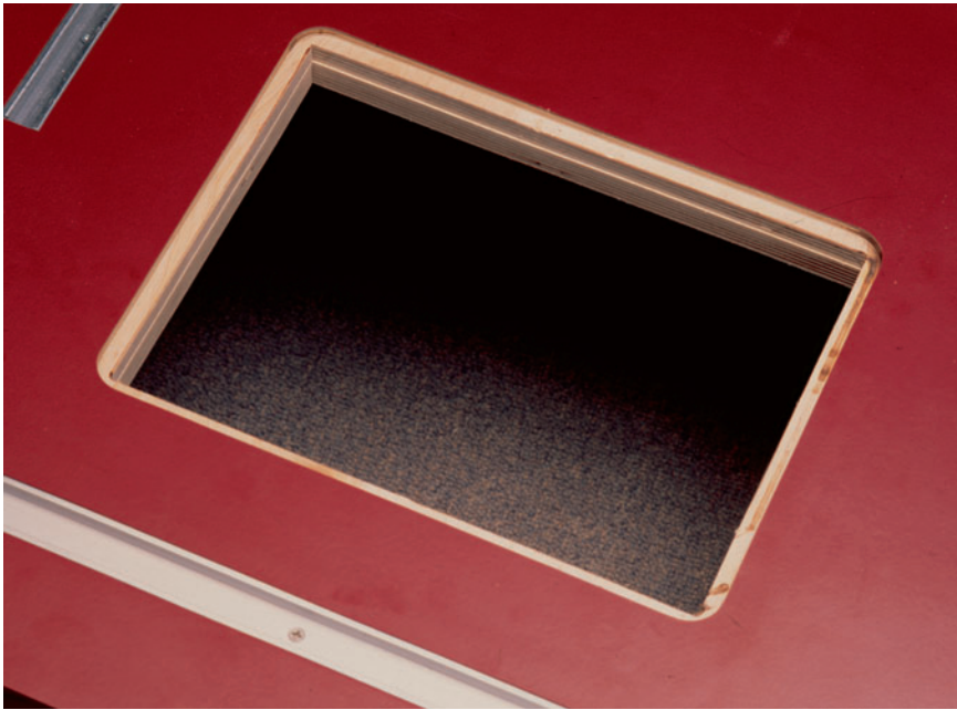
Figure 1: The router table insert rests on a rabbet that holds it flush with the tabletop. Follow the instructions that come with your plate for cutting this opening and rabbet.
