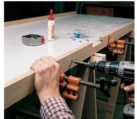
Figure 2: Attach the rails to the melamine deck with screws and glue. Cover the exposed screw holes with walnut plugs.
