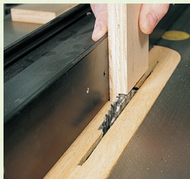
Step 1: Install a 3/8" dado head and a zero-clearance insert in the saw and cut a rabbet at the end of each drawer front and back.
