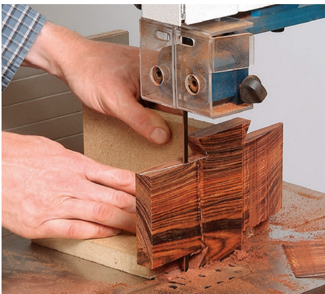
A jig doesn't have to be complex to be effective. Two scraps held together with hot-melt glue and stuck to a workpiece form an effective and safe way to secure odd-shaped stock for deep bandsaw cuts.
