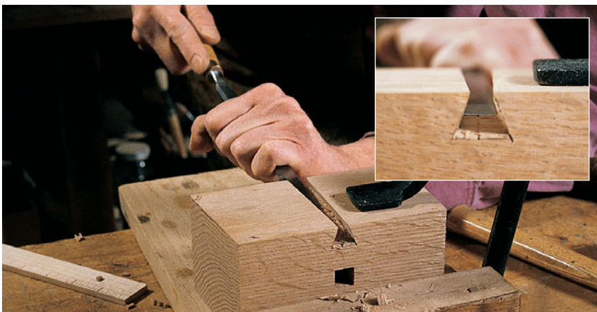
Step 6: Clean up the slots with a sharp paring chisel. Note the gradual slope of the opening, top to bottom.
