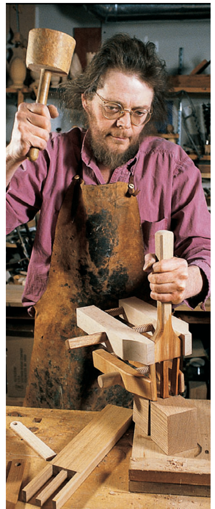
After soaking the pins in boiling water to make them pliable, clamp the ends together until they line up with the oversized dovetail slots. The second clamp keeps the handle from splitting at the base.
