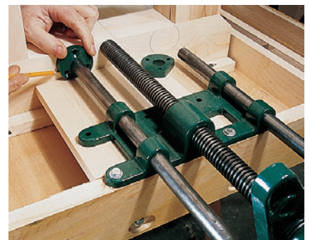
Figure 5: The vise attaches to both the endcap and vise support. With two screws holding the unit in place, establish the locations for the guide rod and center screw holes in the legs.
