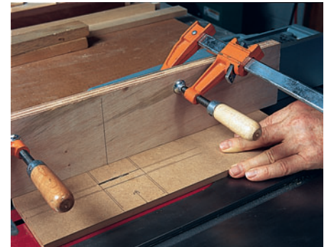
Raise the saw blade through the baseplate (securely fastened by a hold-down clamped to the fence). The center line across the width of the aperture is aligned with the vertical line on the fence.
