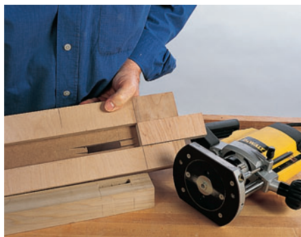
A finely-cut mortise — the first result of careful jig assembly and machine technique.
