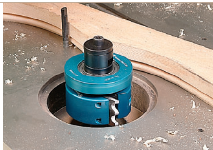
A rub collar and starter pin can shape curves. (Guard removed here for clarity.)
