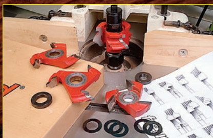
Multi-profile cutters (left) produce many shapes, while rail and stile cutters (right) assist in cope-and-stick joinery.
