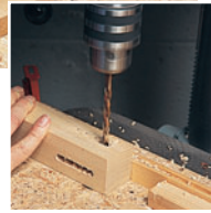
(Above) Drill setup for the first mortise. (Right) Drilling the adjacent mortise.
