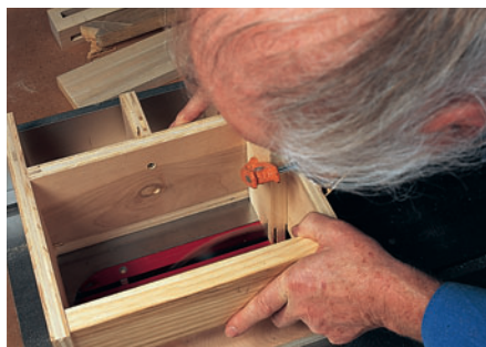
Saw the tenon width and saw the cosmetic shoulder using the same blade height.
