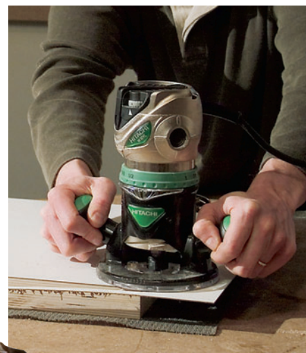
The author trims the laminate flush with a piloted flush trim bit, holding the workpiece in place on an anti-slip mat.
