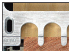
Board alignment lines
