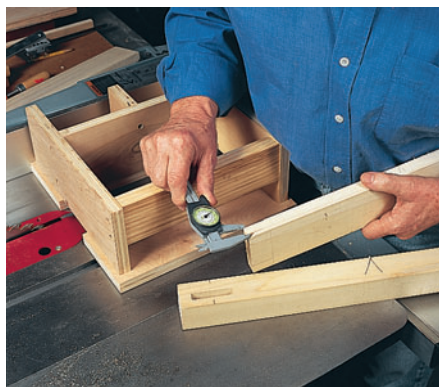
Position the jig for the second face cut, using the spare rail. Make a test cut and check with a vernier caliper to confirm tenon thickness is correct.
