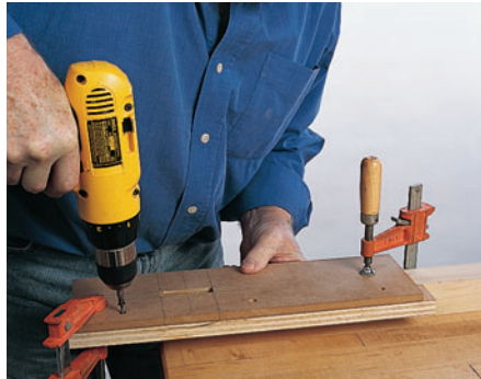
With the baseplate opening milled, attach the first base block and then add the second, using the leg as a spacer.
