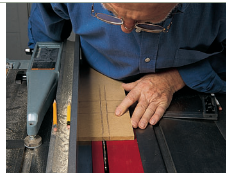
Set the first cut on the baseplate of your jig by aligning the outside of the saw blade with the aperture guideline.
