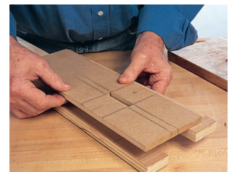
Here are the finished baseplate and two guide blocks, separated by the mortise workpiece.
