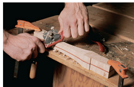
A comfortable handle is the key to a successful mallet. To reduce tearout while spokeshaving, work from the high points to the low.
