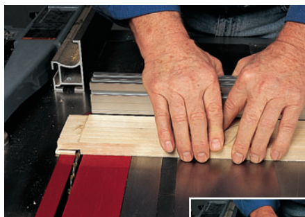
Saw all four shoulders with the miter fence.
