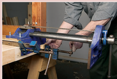
Hang the vise with the top turned upside-down. (The mounting bolts are on an older bench, before I began using lag screws.)
