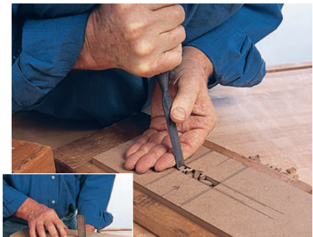
Remove the waste at each end of the aperture by vertical paring with a bench chisel. Now check for square.
