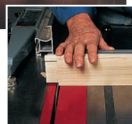
Saw all four shoulders with the miter fence.
