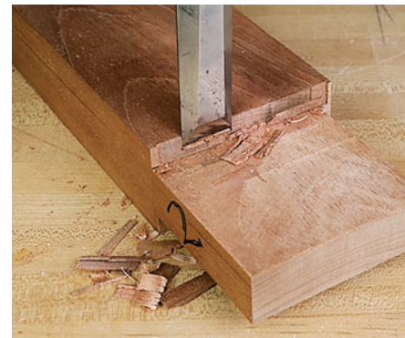
Slower is surer: knife the shoulder lines and clean up with a wide and sharp chisel.
