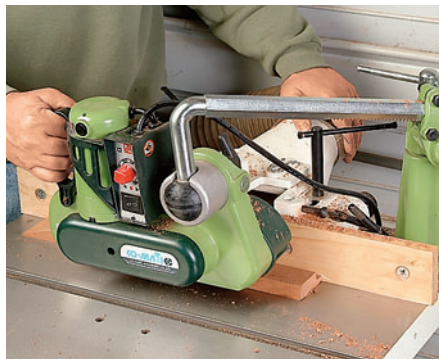
A power feeder lets you "climb cut" stock — which you can't do by hand feeding.
