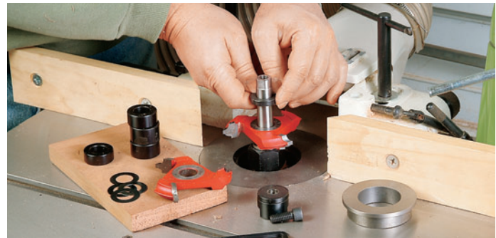
Metal spacers help set up cutters correctly on the spindle, while a variety of throat plates accommodate the different diameter cutters.
