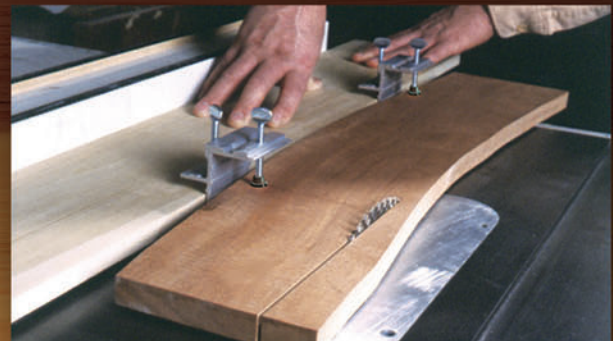
Straighten crooked boards in two passes
