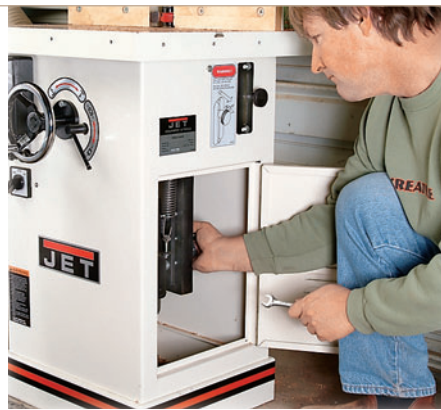
The hand wheel changes a shaper's spindle height, while controls inside the base change motor speed.
