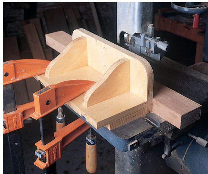
A point fence, like the adjustable shop-made version above, is the key to being able to adjust for blade drift as you resaw. This example fits into the saw table miter slot.
