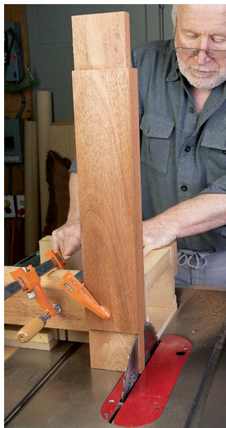
A block clamped in place on the front of the jig positions the rail to cut the cosmetic shoulder and avoids sawing into the jig.
