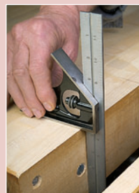
Make the fixed cheek square with the benchtop (left). A clamped workpiece should be square (center) with the top and vise cheeks parallel (right).
