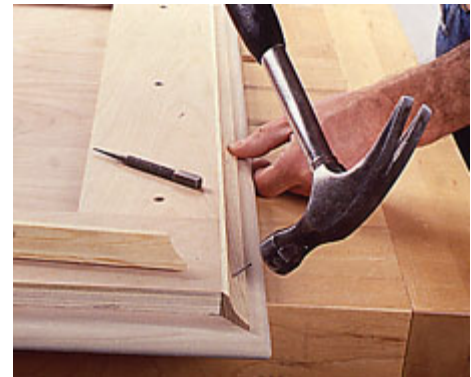
12--After the support strips have been installed on the bottom of the top, miter and nail cove molding to edges of strips.
