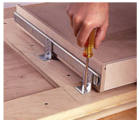
16--Attach slides to pencil drawer and plane on bottom side of top. Drive mounting screws through slotted holes.
