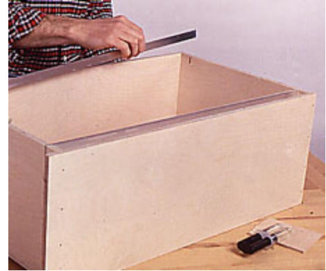
17--Cut aluminum bars for hanging files to length. Then, apply a dab of epoxy to the support slots and push the bars in place.
