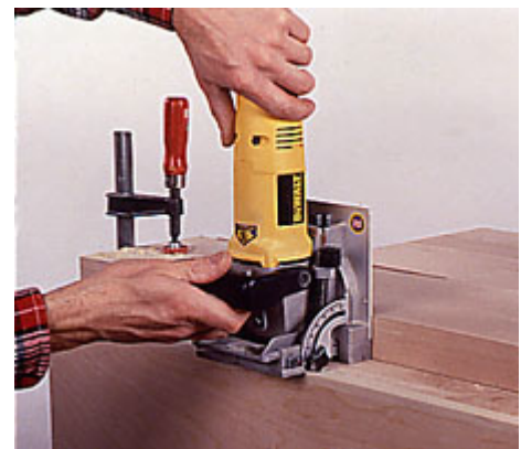
7--Clamp a straightedge to the case side to guide the joiner. Then, cut slots for the plates used to attach the modesty panel.
