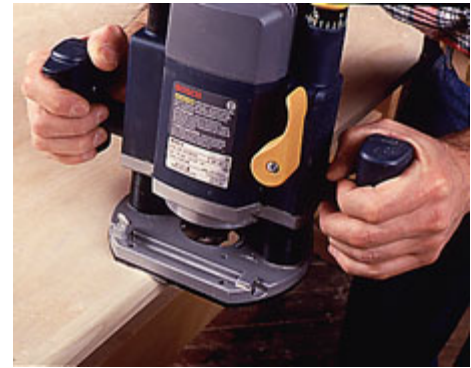
11--Glue and clamp the edge banding in place and, when glue is dry, route the top edge with a 3e8-in.-rad. rounding-over bit.
