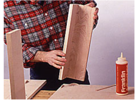
5--Begin assembly with one side on the bench. Apply glue to plates, slots and edges, then push the second side in place.
