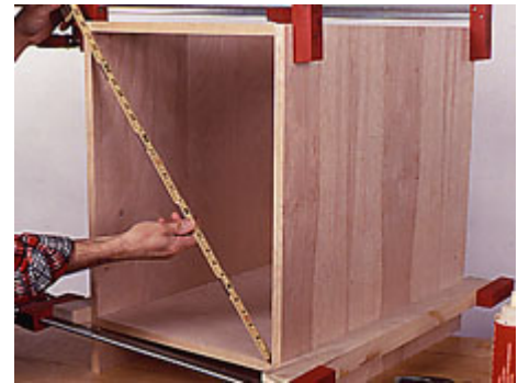
6--Draw all joints tight with clamps, then check the case for square by comparing opposite diagonal measurements.
