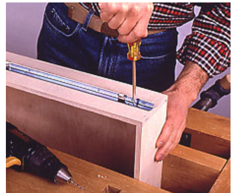
18--Install the slides on the other drawer assemblies. Again, use the slotted holes so you can easily adjust the parts later.
