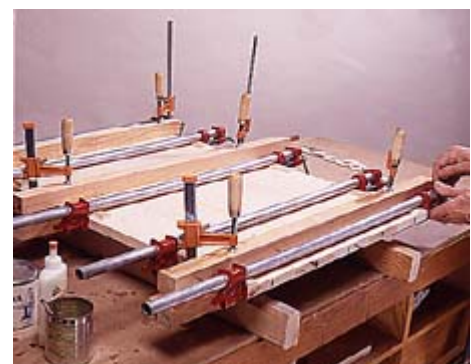
2--Save glue application time by pregluing the joining plates in their slots. A small-nozzle bottle is handy here.
