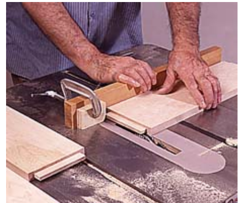
7--Use a stopblock clamped to the miter gauge and a dado blade in the table saw to cut the apron tenons.
