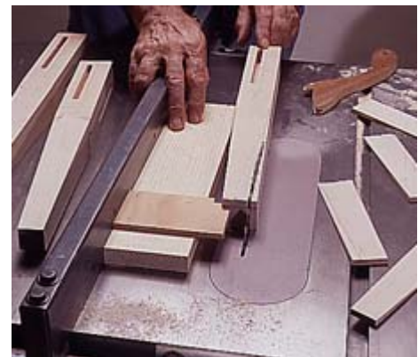
5--Use a stepped jig on the table saw to cut the leg tapers. Each step positions the leg to cut two tapers.
