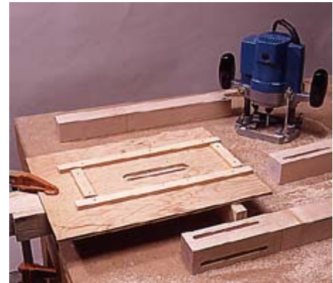
4--Use a jig and a plunge router to cut the leg mortises. The stops are positioned to suit the router's base.
