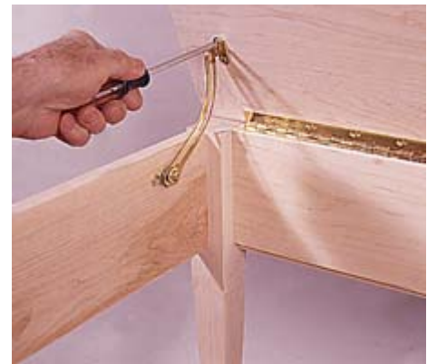
10--Sequence is important when attaching the top's support hardware. Attach it to the apron first, then the top.
