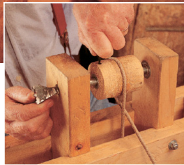
The drive center is shown here being formed, with the jigsaw crankshaft lying next to it. After rough shaping, the center is filed and ultimately takes on its spade-bit shape. The center is then mounted in the drive pulley by tightening the stop collars.
