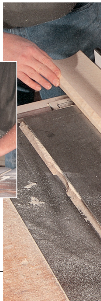
After the cove cut is made, cut the bevels on the front face of the moulding. Set your saw blade to cut a 45-degree bevel and rip the edges.
