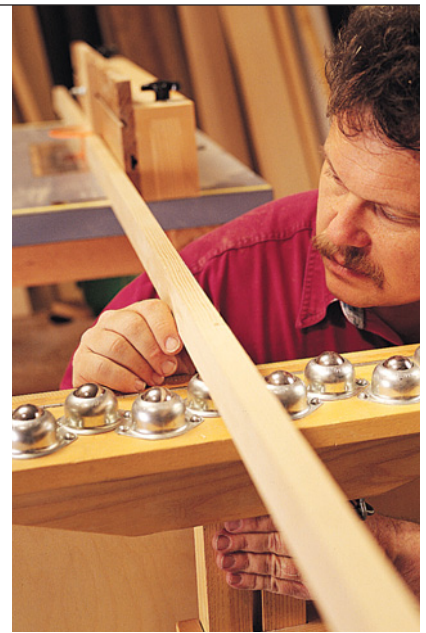
To use the roller stand alone, simply swing the extension table down out of the way.
