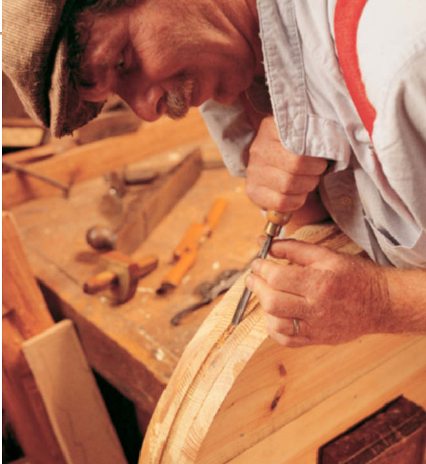
Carving the groove in the flywheel for the rope takes a little time, but the changes in end-grain direction makes carving easier than turning.
