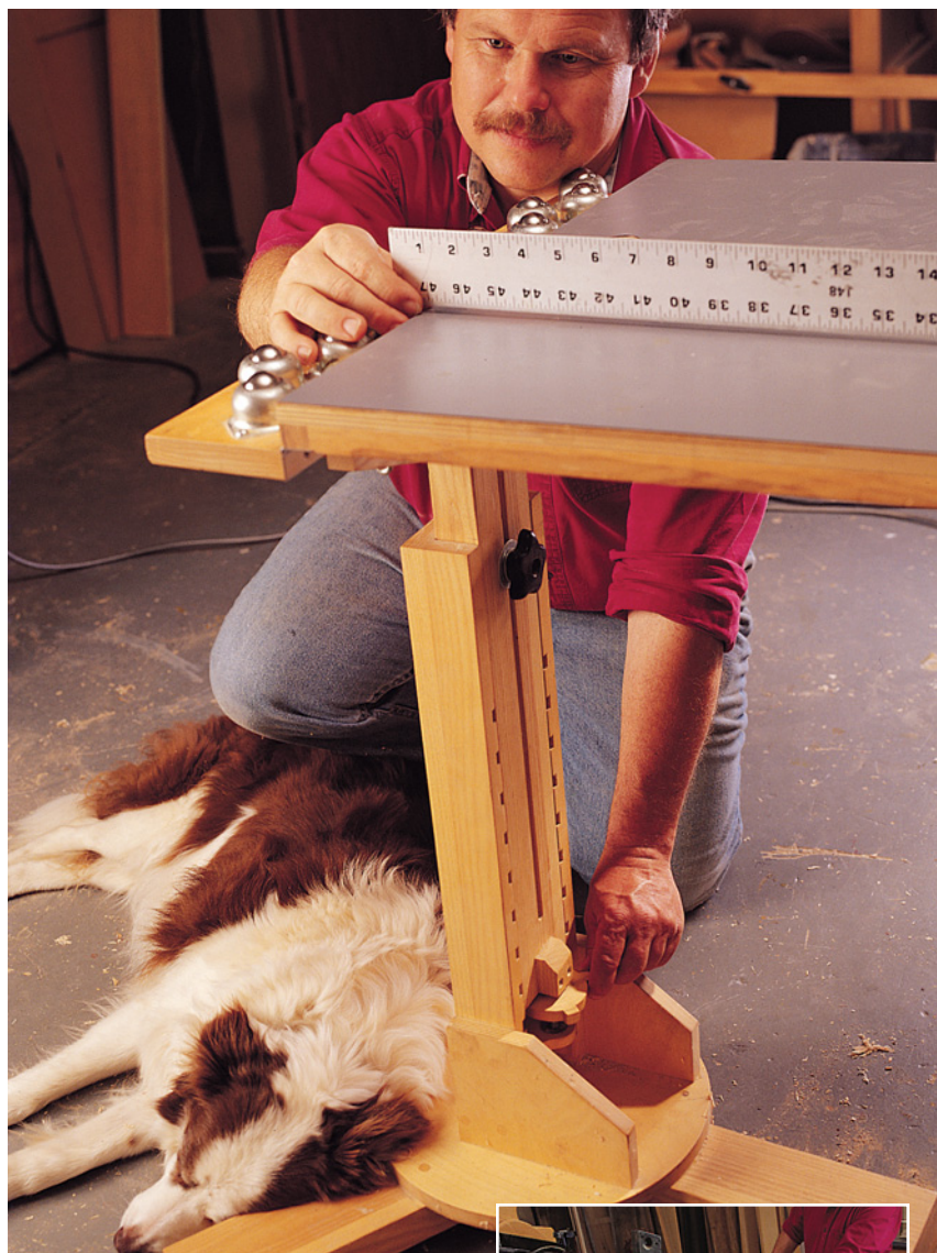
To adjust the extension table level with the tool, lay a straightedge across them. Loosen the locking knob and raise the roller head. It’s so easy, you’re guaranteed not to curse and wake Fluffy.
