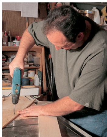
I screw my fence in place. If you don't want to poke holes in your tableboard, C-clamps will do just as well.
