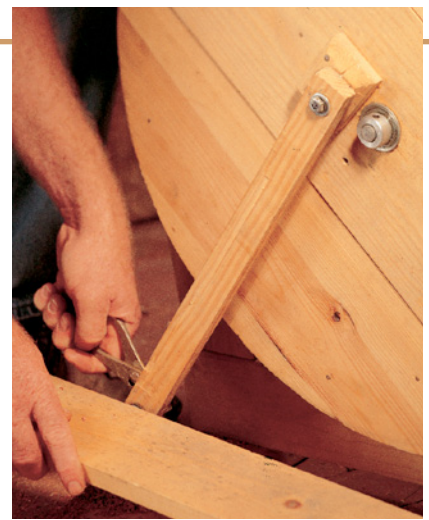
The connecting rod is attached to the treadle by a lag bolt screwed into the treadle side. The opposite end of the connecting rod rides on a \frac{3}{8} " lag bolt screwed through a small block (to allow clearance over the stop collar) into the flywheel.
