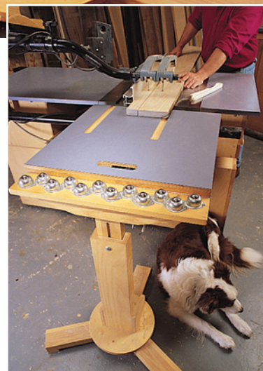
To adjust the extension table level with the tool, lay a straightedge across them. Loosen the locking knob and raise the roller head. It’s so easy, you’re guaranteed not to curse and wake Fluffy.
