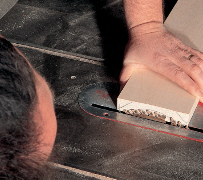
First set your blade to the finished height of the cove cut using the drawing on the end of a piece of stock.
