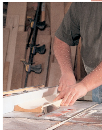
After the cove cut is made, cut the bevels on the front face of the moulding. Set your saw blade to cut a 45-degree bevel and rip the edges.
