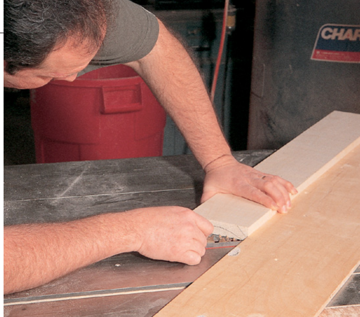
Place the auxiliary fence on the top of the saw's table and line up the teeth with the arc drawn on the end of your stock.
