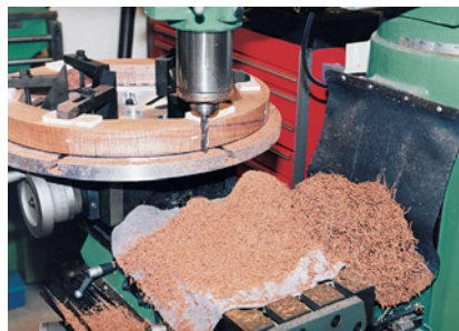
Milling machines excel at dealing with round shapes. Clockmakers will be amazed at what this machine could do for their woodworking.
