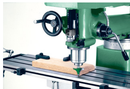
The table travels left to right 18½" and forward and back 10¾".
