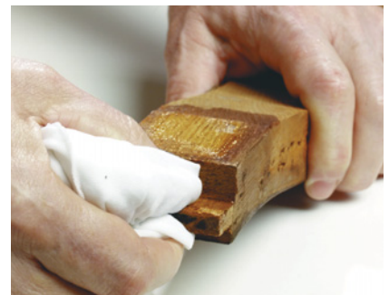
You can easily dissolve and wash off old hide glue with hot water or vinegar. If the glue is stubborn, scrub it with a stainless-steel kitchen scrubber or coarse Scotch-Brite pad and hot water.
