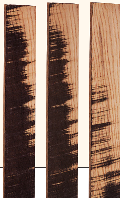
These boards were painted black to better show progressive passes on the jointer with the left photo the first pass. Even though some black or rough-sawn areas remain by the third pass, it is ready for planing, starting on the opposite face.
