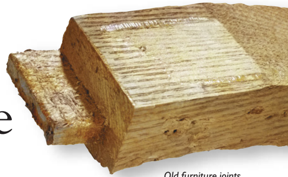
Old furniture joints were glued with animal hide glue, which must be removed before regluing with any glue other than hot hide glue so the new glue can bond to the wood.
