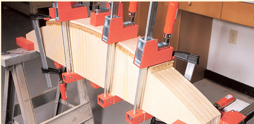
In gluing up the laminations, I use a brush to cover every square inch of the wood face. I thin the glue with a little water to make it easier to spread. Thinning will not affect the holding power of the glue. The glue run out on the sides is a good sign that all surfaces are bonding.
