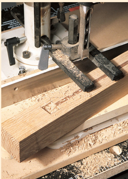
The square ends of the inlays can be done with a mortiser, as shown here, or you can use a router with a template and use a chisel to square out the corners.
