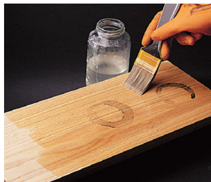
Brush on the oxalic acid solution over the entire board. The dark marks will begin to fade immediately, though it might take 15 minutes or longer for them to disappear completely.
