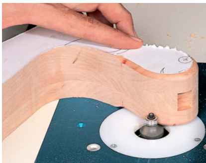
Here you can see the \frac{1}{4} " roundover bit at work on the head area. Be sure to roundover just the head on the "A" and "B" assembly.
