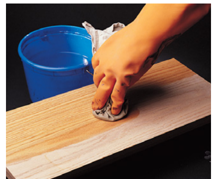
After the board has dried, remove the crystals using a wet rag or a hose. Never brush the crystals off the surface.
