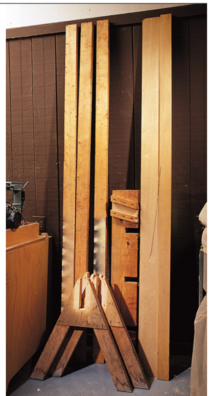
The cutting grid breaks down when you're not using it and stores against a wall, along with the circular saw guide. The grid is so useful however, that mine is set up more often than not.
