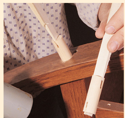
A \frac{3}{4} " dowel with slots and wedges will hold the rockers in place for many years to come.
