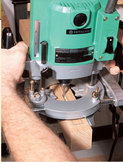
Start the inlay work on the four legs by using a router with an edge guide to rout the 1/4"-wide channels for the inlay.
