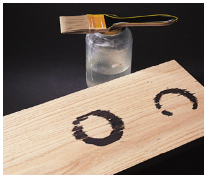
To remove dark water stains, you'll usually have to first remove the finish from the piece. Oxalic acid crystals can be bought at better hardware and paint stores. Sometimes it's labeled "wood bleach."
