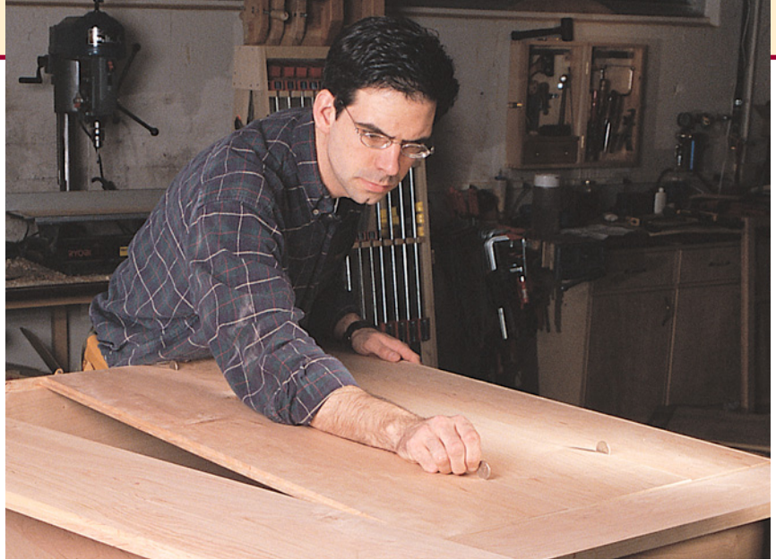
Get a pocketful of quarters when putting the back in place. You want the back to expand and contract with the seasons, and the thickness of a quarter is just about right.
