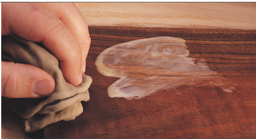
To find glue splotches before you stain, wet the surface with paint thinner or water. The glue will show up a lighter color.
