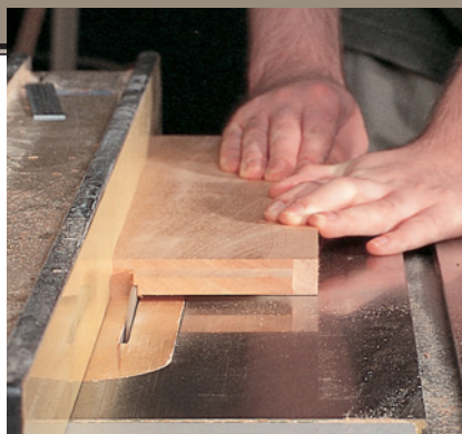
You will need to fasten the tabletop using tabletop fasteners, which requires making a kerf in the aprons. I made this kerf on the table saw \frac{1}{16} " from the edge and \frac{1}{4} " deep.
