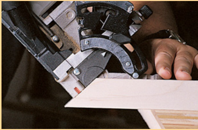
If your fence is adjustable only between 0° and 90°, you can cut the joint on the inside of the miter. Just be careful when positioning your tool.
