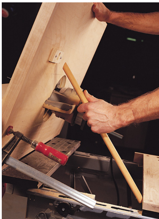
Once the tabletop is hinged to the Workmate's front board, it's easy to locate the positions for the prop stick and stick bracket. Note the shop-made replacement board for the Workmate top.
