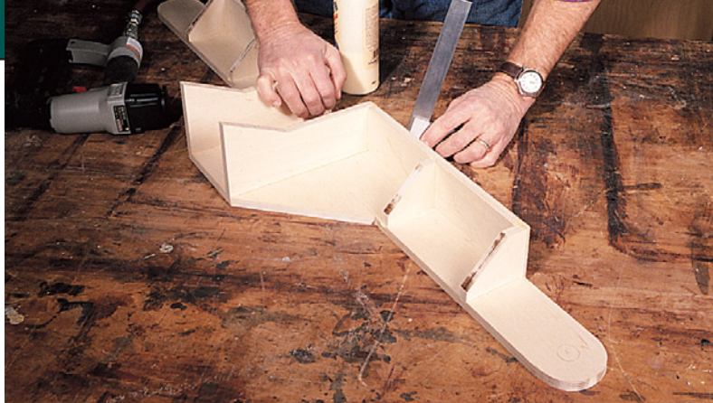
As you assemble the fence, make sure it is square along its length. Be sure and check it again after it is clamped up.
