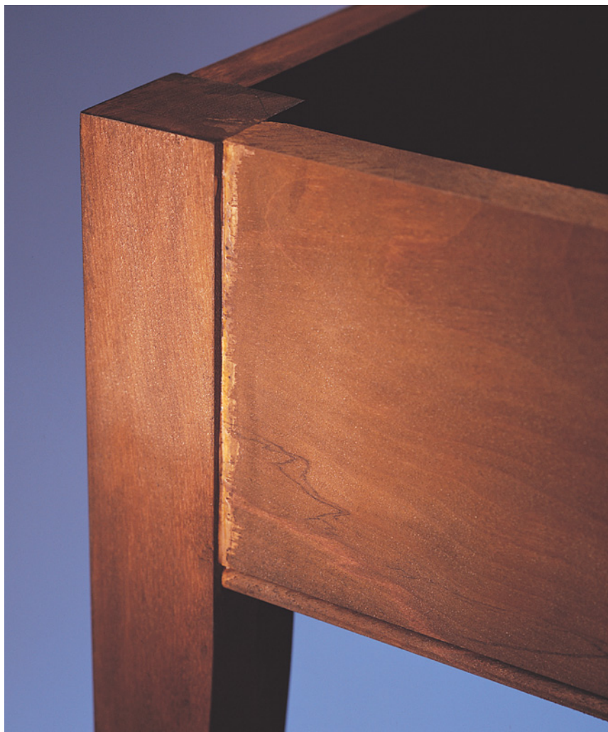
Glue squeeze-out is a particularly thorny problem when a joint meets at a 90° angle, such as a table leg to an apron. And because the apron is set back, it's easy to miss the squeeze-out during sanding.
