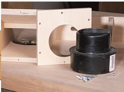
Inside view of the dust chute from the rear including the plastic 4" to 3" dust collection hose adapter. Rout the 3" hole for the adapter with the circle-cutting jig or use a "fly cutter" in your drill press.
