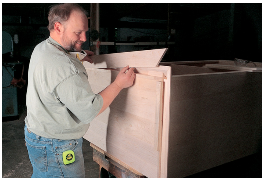
The last step on the crown is to attach the cap to the crown and cabinet. Notice the glue blocks behind the crown moulding to support the crown and add stability.
