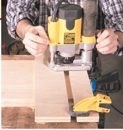
This plywood jig cuts the dados in the sides that hold the top and bottom pieces. Here I'm cutting the dado for the bottom. Note how the edge of the jig is flush to the bottom of the case.
