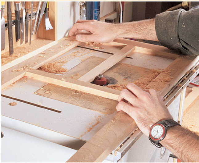
Cut the rabbet for the glass using a rabbeting bit in your router table. After the rabbet is cut, you'll need to square the edges with a chisel. Because this work is delicate, make sure your chisel is super sharp.
