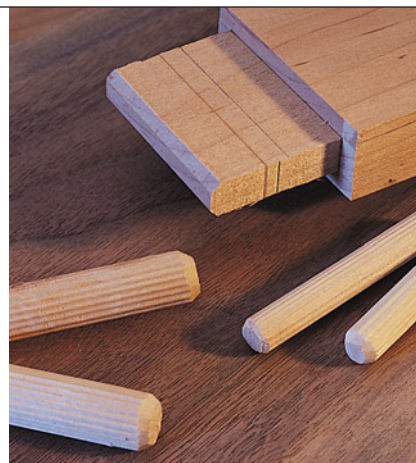
One way to avoid squeeze-out is to design your joints so that excess glue has a place to collect. Chamfering the ends of your tenons or using dowels with chamfered ends will help.
