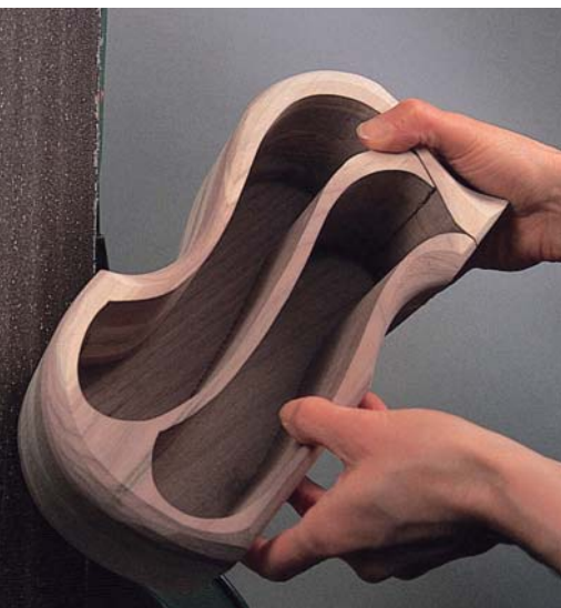
When shaping the box edges, feed the wood into the belt with an upward motion. In general, take more wood off on the thicker edges, and less where it's thin.
