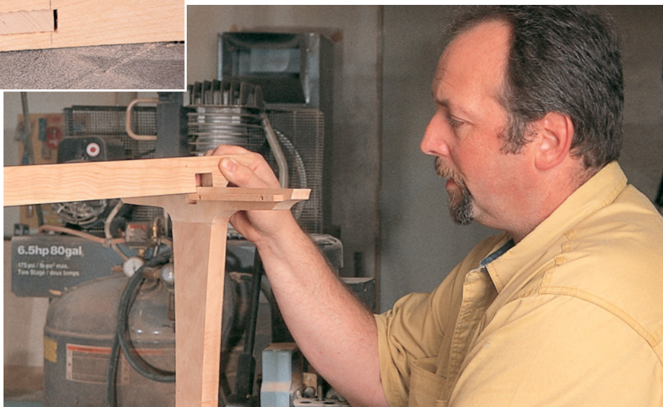
The legs and stretcher are held together with an edge-lap joint. The legs are notched through the mortise-and-tenon joint (above), and a mating notch is cut in the stretcher (right).
