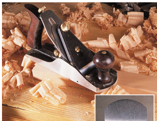
At the mouth of the plane you can see how the frog extends all the way to the sole. The design is supposed to reduce blade chatter.
