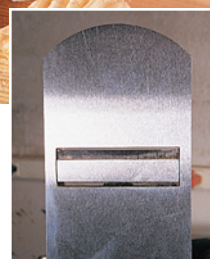
At the mouth of the plane you can see how the frog extends all the way to the sole. The design is supposed to reduce blade chatter.
