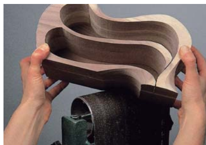
A little twist of the wrist over the top cylinder can create some interesting effects in your box's inner curves.
