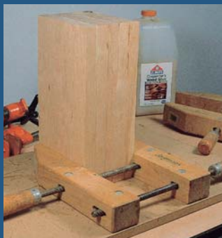
The bar on a handscrew clamp helps keep the pieces in line while clamping a block.
