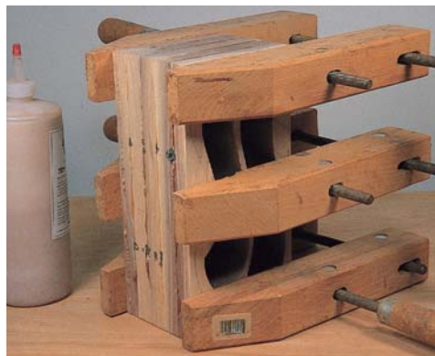
Glue and clamp the back slice on, making sure all surfaces are contacted. Go lightly on the glue close to the inside backs of the drawer cavities to prevent too much excess glue from squeezing into the box innards.
