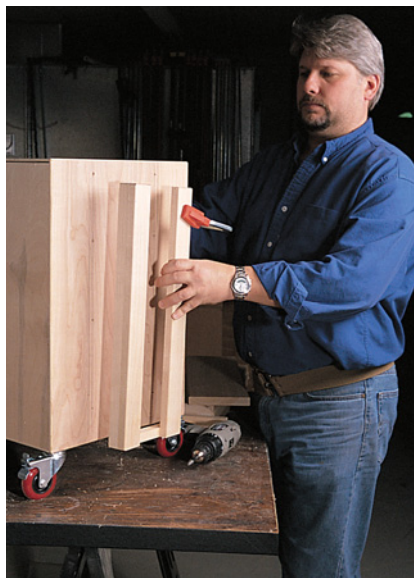
After drilling the clearance holes in the cabinet sides, I used a clamp to hold the channel assembly in place while pilot drilling, then screwing the channels in place from the inside of the cabinet.
