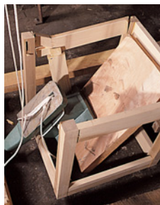
The mortise-and-tenon cube after the second hit.
