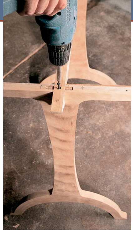
The edge lap joint isn't the strongest in the world, so I decided to add a screw to help out a little bit.
