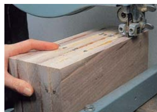
Feed the block slowly into this small blade. Forcing it will only give you a rough cut and possibly cause the blade to bow to one side.
