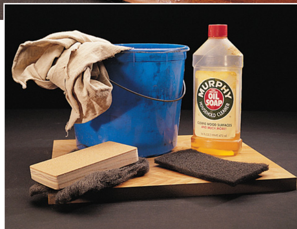
You also can merely abrade the finish, which is not as effective as sanding. Steel wool (or gray Scotch-Brite pads) and a lubricant such as Murphy Oil Soap dissolved in water is all you need.
