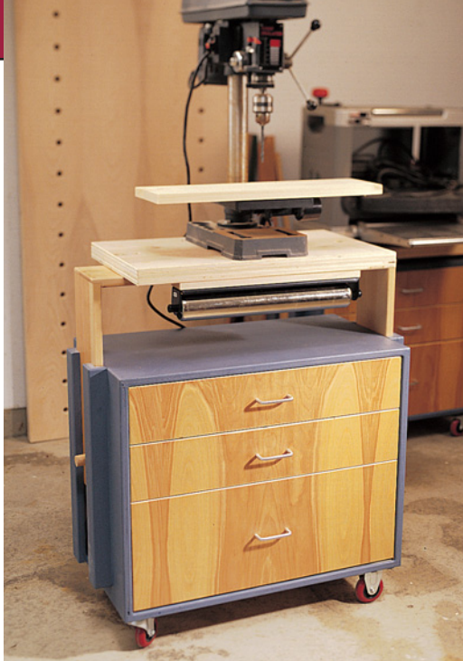
By adding smaller tops to the individual cabinets, each makes a fine tool stand with lots of storage beneath. Note the roller stand mounted on the underside of the top. Flip the top over and you've created an outfeed table for any machine.
