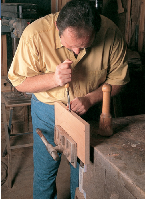
After drilling out the mortises in the feet using my drill press, I cleaned up the mortise and squared the corners with a chisel. I'm glad they shot this picture because I don't use hand tools too often.
