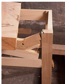
The mortise-and-tenon cube after the first hit.
