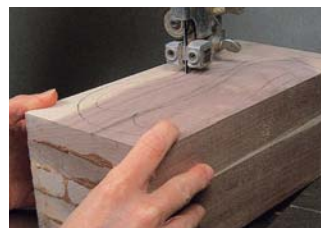
Smooth pattern cuts are accomplished by keeping the blade guide close to your work. Feed slowly to prevent straying from the lines.
