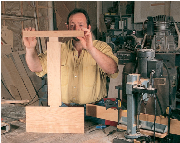
With the mortise-and-tenon joints complete, I transferred the shape of the legs from the template to the pieces. Band saw the shape, then sand the edges smooth. You might note that the grain orientation on the feet isn't really the best, as it makes a weak support. But when making a reproduction...
