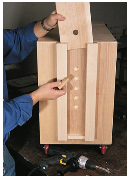
A 1" dowel is a simple and secure way to hold the support arms at the proper height. The five hole locations (and the all-the-way-down position) give you a variety of working heights.
