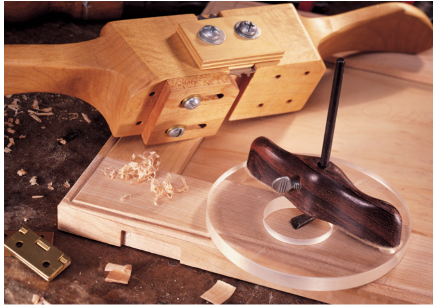
A beader (above) is a great tool for hand detailing furniture and is easier and safer than an electric router in some cases. A hand router excels at cutting hinge mortises and cleaning out grooves.
