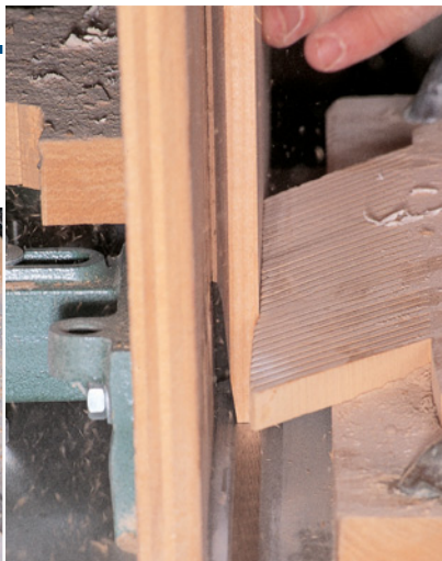
I like to cut most of the bevel on the raised panel on my table saw (left). Then I use a vertical raised panel bit in my 1½ hp shaper to cut the profile in one pass (above).
