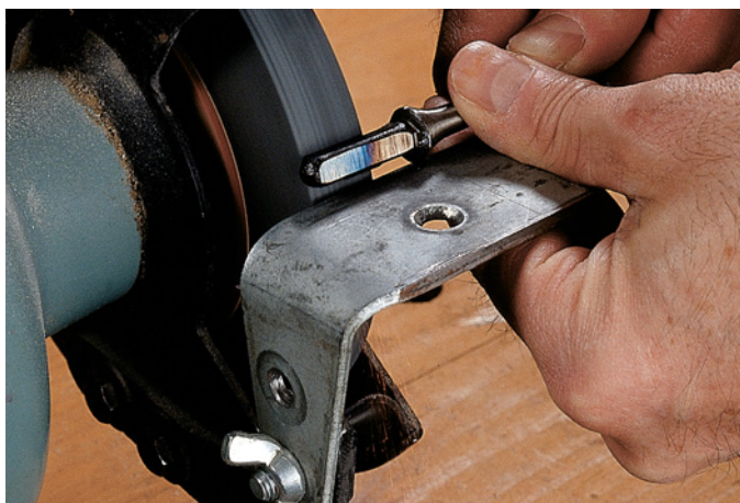
Grind flat facets on a round cast tang made for a composite handle to ensure a tight fit in the new wooden handle.
