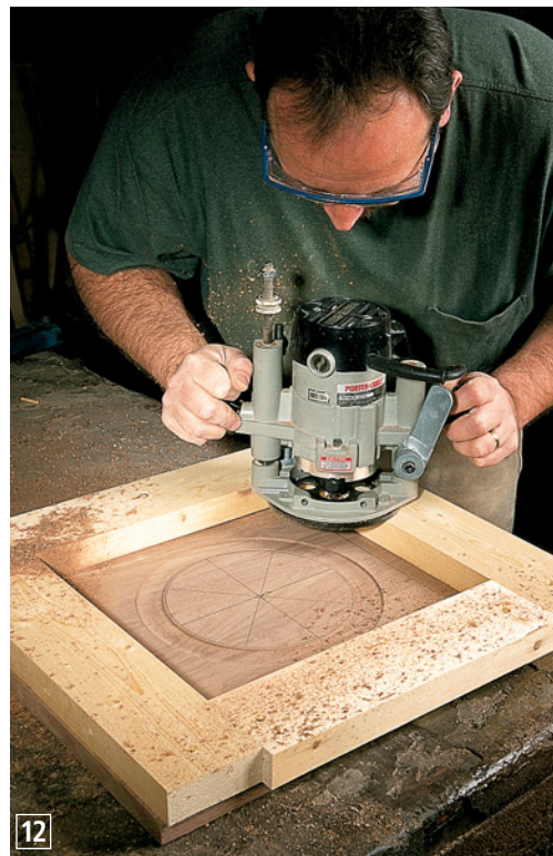
For the next step I chose to make a simple 2x4 frame and used a bit with a top-mounted bearing to create the outer border recess. This ensures that the corners will meet accurately. I used a 3/4"-wide straight bit to make the cut with a single pass. After the cut, use a chisel to square out the corners.
