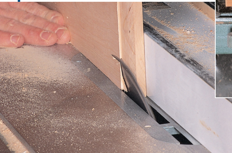
I like to cut most of the bevel on the raised panel on my table saw (left). Then I use a vertical raised panel bit in my 1½ hp shaper to cut the profile in one pass (above).
