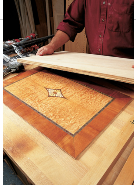
For the crowned bars to work properly, the assembly must rest on a flat, rigid surface such as a workbench. Be careful not to over-tighten the clamps. If the middle of a bar lifts off the assembly, the clamps are too tight.
