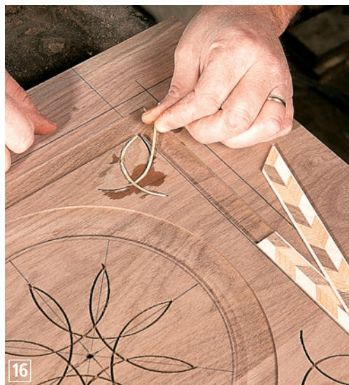
To make the banding for the corner arcs, set your table saw to once again slice 1/16" strips from a larger piece. Then carefully slice the strip to a little over 1/8" thick. A straight edge and utility knife will serve well here. Then add a little glue and press them into the recess. Make some extra strips in case some snap. I used tiger maple, which is pretty brittle. Holly would have been easier to work with.
