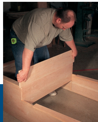
To save time and effort, I glue up the panel for the countertop from two boards so it will fit perfectly into the dados in the sides.
