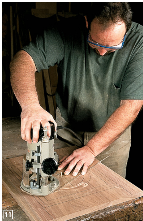
With the inlays made, lay out the pattern on the door front. The first step is to cut the circle pattern. I used a shop-made circle-cutting jig (though you can also purchase one), making the 1"-wide recess 1/8" deep in two overlapping passes using a 3/4" straight bit. Start with the outside dimension, then adjust the jig inward to the inner diameter.
