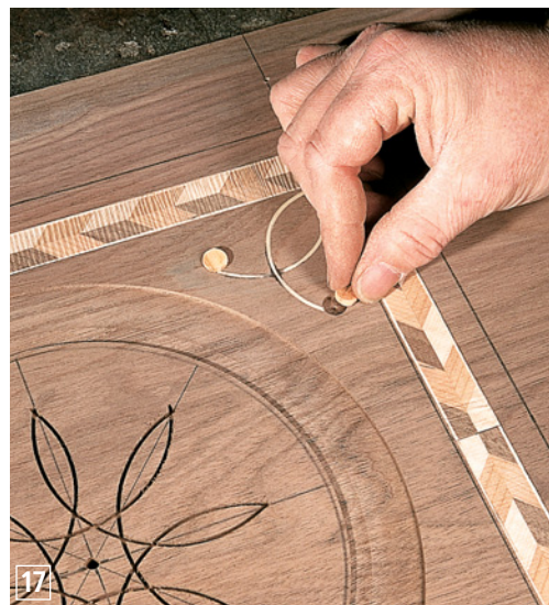
For the "berry" designs, I used a 3/8" plug cutter to make a number of 1/8"-thick dots. Carefully glue these in place. The berries in the center of the pattern are created in the same way.
