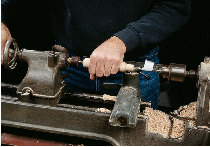
Bore the tang pilot hole on the lathe using a machinist's drill mounted in a chuck on the head stock. Feed the handle into the spinning bit with the feed wheel on the tail stock.
