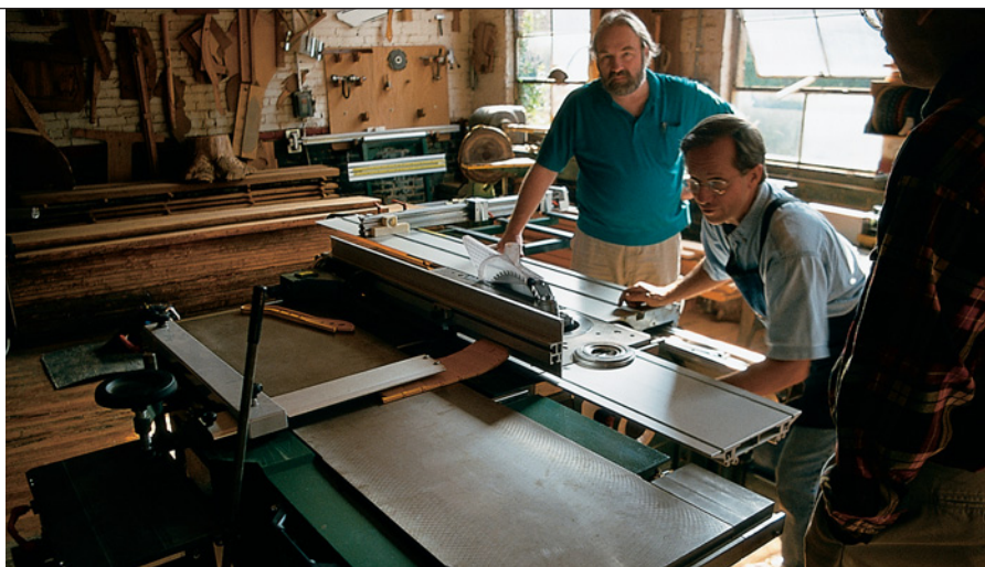
Mehler (center) demonstrates his Felder combination machine. It's amazing how the splitter moves up and down with the blade. Why can't we have this on all U.S.- and Taiwanese-made saws?
