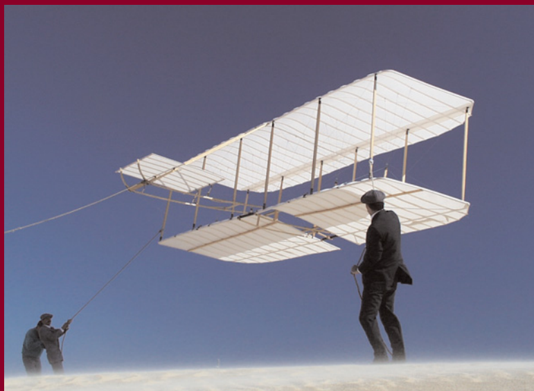
Tom Cherry and David Thompson measure the lift of the 1901 Wright Glider, recreating one of the Wright brothers' experiments.
