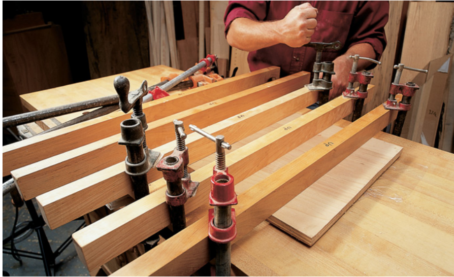
For the crowned bars to work properly, the assembly must rest on a flat, rigid surface such as a workbench. Be careful not to over-tighten the clamps. If the middle of a bar lifts off the assembly, the clamps are too tight.
