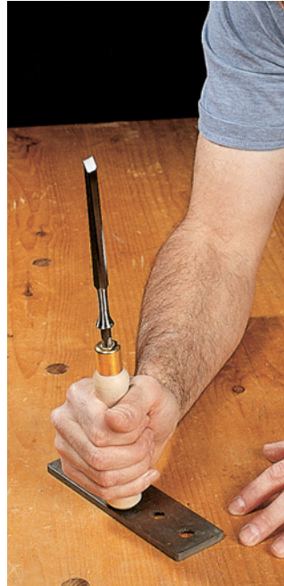
Seat the tang in the handle by repeatedly striking the end of the handle against an iron plate or machine table.
