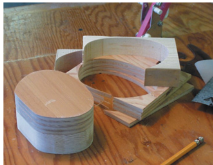
Here you can see parts B, C, D, E and F after they’ve been cut out using the band saw.
