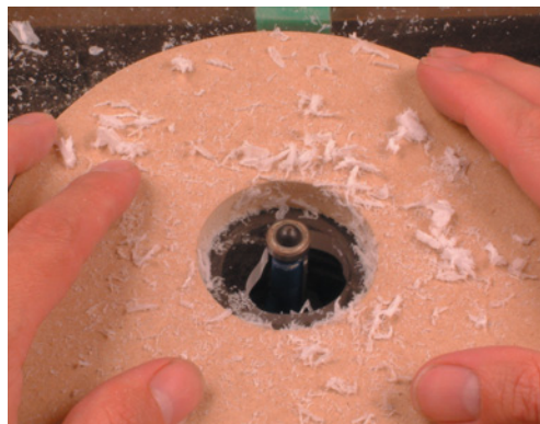
After cutting an adequately sized starter hole with a drill bit, a bearing-guided flush-cutting bit does a nice job of shaping the interior holes to match the template.
