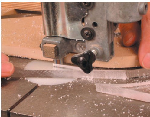
With the template carefully attached to the acrylic, use your band saw to rough-out the shape of the jig itself. Leave a little extra, but don't leave so much that the router won't be able to clean it up easily.
