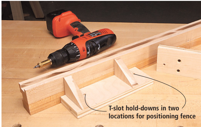
The fence is supported by two simple brackets screwed to the rear of the fence. The location of the triangular braces is important to the track orientation, so follow the diagrams carefully for location.
