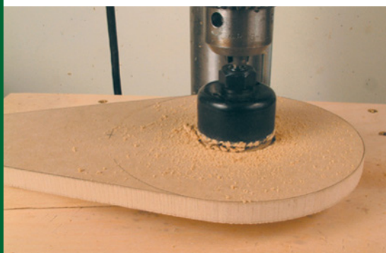
For the interior holes in the template, hole cutting saws, Forstner bits or spade bits will do the job. Make sure you back up the template to avoid blowout on the backside of the workpiece.
