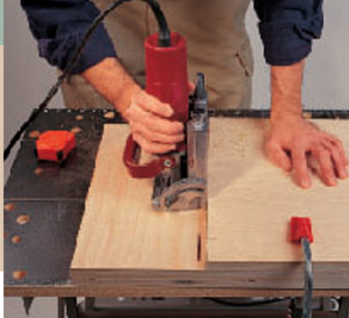
Using the lines you marked on the partition, cut the slots in the cabinet side using the partition as a fence.
