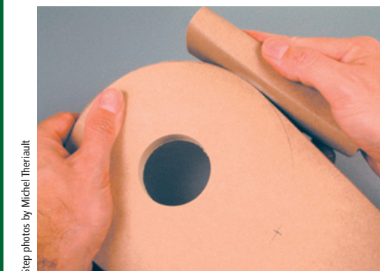
With everything cut, holed and sized appropriately, the last step is to clean up the edge so that it's smooth. A block and sandpaper can do most of the work, but an edge sander (if available) will be much quicker.
