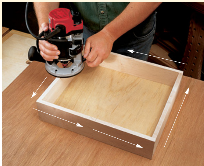
For most routing operation, counterclockwise is the correct direction. As shown here, that is with the bit on the outside of the box, following the arrows around the box. If this were a solid door or panel, instead of a drawer, the motion would still be the same - counterclockwise.
