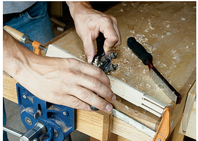
You can shape the handle with a spokeshave in less time than it takes to read this article. By clamping the handle as shown, you can spin the handle to quickly round over all four edges.
