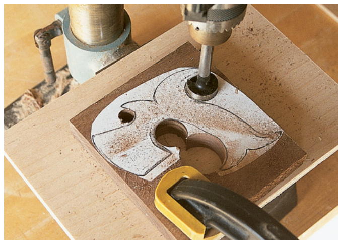
Use Forstner bits to make perfectly radiused curves. Connect the holes using your band saw, and you are halfway there.
