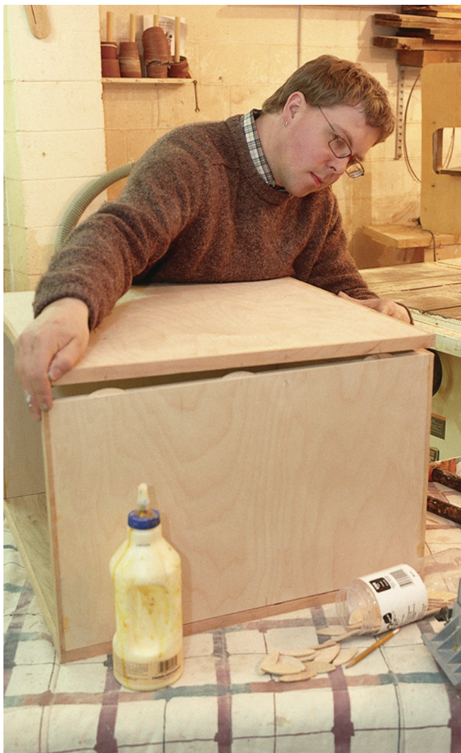
During the second stage of cabinet assembly, laying the cabinet on its side keeps you from fighting with gravity. The cabinet comes together relatively easily, and the alignment is a snap thanks to the biscuits.
