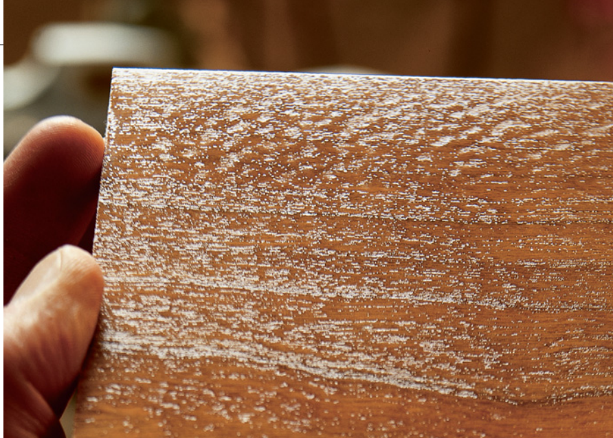
Orange peel, a problem that occurs with spray systems, can be reduced by thinning and by adjusting the gun. This piece of closed-grain birch should have a flat, nearly flawless finish.
