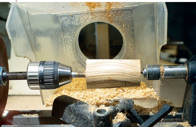
After sanding down the corners, mount the blank on the bolt and use the tailstock of your lathe for support.
