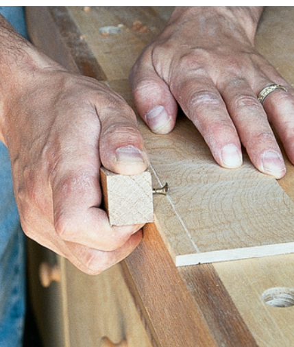
To make a quick-and-dirty scratch stock, sharpen the head of screw with a file. Apply light pressure, keep the stock against the blade and let the screw do the work.
