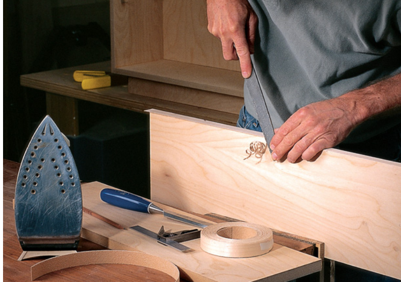
Apply a hot iron to hot-melt-glue backed edge veneer, then file off any veneer overhang using the teeth on your file's edge. It works just like a saw.
