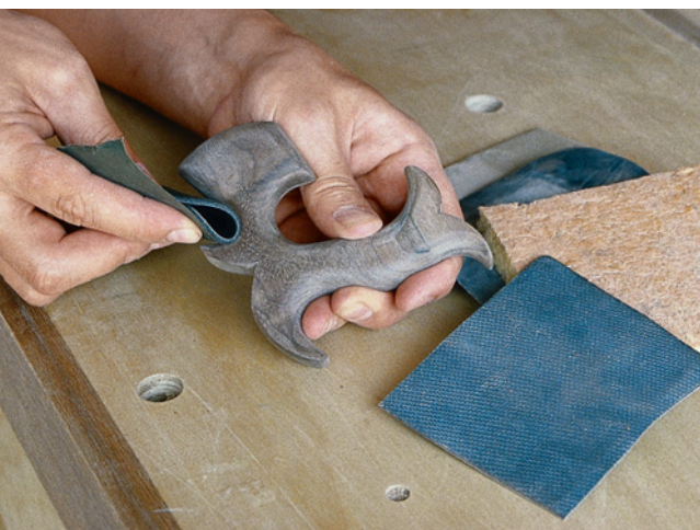
Back your sandpaper to smooth the curves. Old mouse pads and carpet padding make excellent custom sanding pads.
