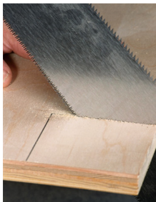
Before assembly, handsaw 3" x 3 3/4" notches in the sides at the bottom corners to make the toe kick space.
