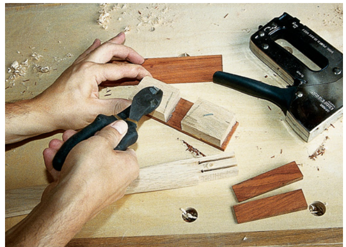
Clip the heads off of staples to prevent the laminations from slipping during glue-up.
