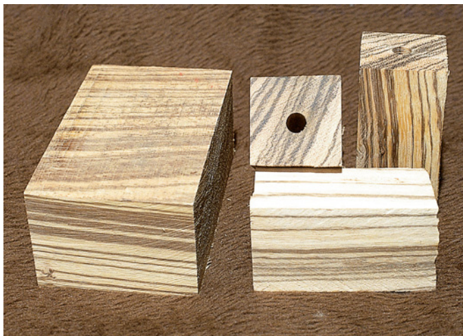
Here you can see the three bottle stopper blanks and the piece for the stand. The hole drilled in the center of each blank is \frac{23}{64} " in diameter and 1" deep.
