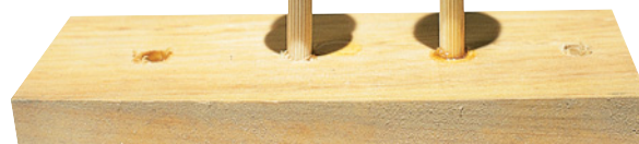
After applying the finish to the stoppers, the best way to let them dry is to make a small rack that holds the stoppers' mounting dowels.
