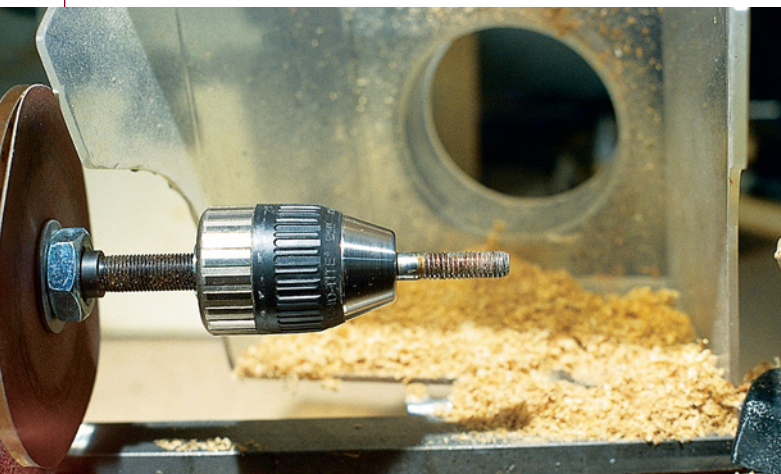
I've found the best way to turn these stoppers is to screw them onto a bolt (that has had the head cut off) that's chucked into my lathe.
