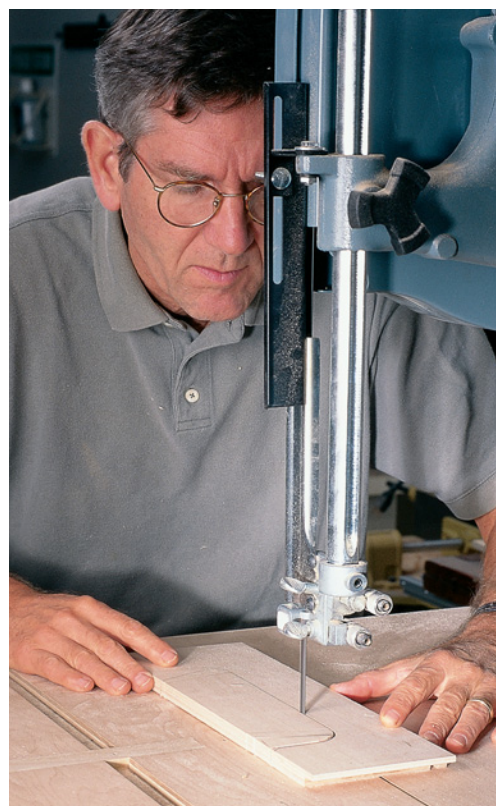
Mark the cutout on the fronts of the pull-out trays and then band saw to the line and sand. Then go ahead and assemble the trays.
