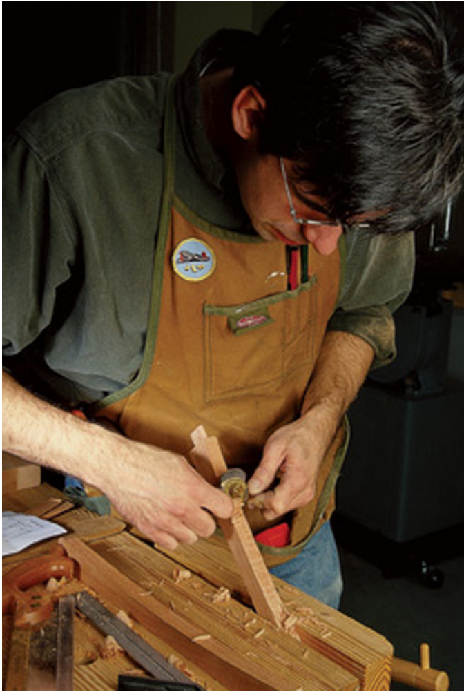
A spokeshave cleans up your saw cuts on the top rails quickly. After working with the fancy Leigh jig, it's a relief to pick up a tool that's simpler than I am.
