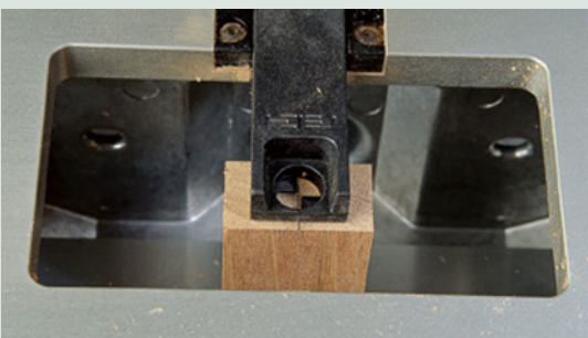
Center the table over your tenon using the slide-out window. Lock the table in place and put the router up on the jig.
