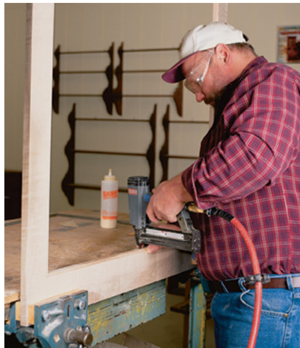
Some people like to make the beading part of their face frame. I find that it's easier to cut a \frac{5}{16} "-wide piece of bead moulding to size and then attach it to the frame. Here you can see I'm attaching my face-frame bead with a brad nailer.
