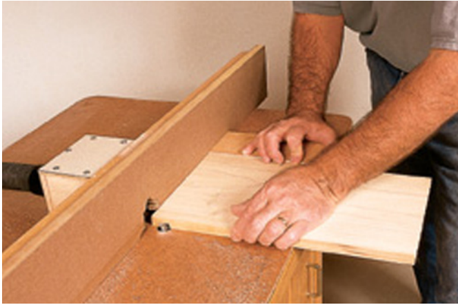
The typical router table setup works for dadoing parts like drawer sides. A push block – just a square scrap – stabilizes the work and backs up the cut, preventing tearout as the bit emerges from the cut.
