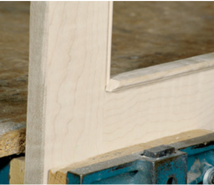
This is what the face-frame bead looks like before I nail it in place. No one would ever know that I made the beading separate from the frame.
