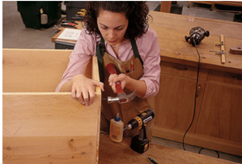
The rear rabbet joint is a better joint than a butt joint for stability, but some glue and a few nails make it an even better joint. To make the nails more attractive, we used antique-looking cut nails.
