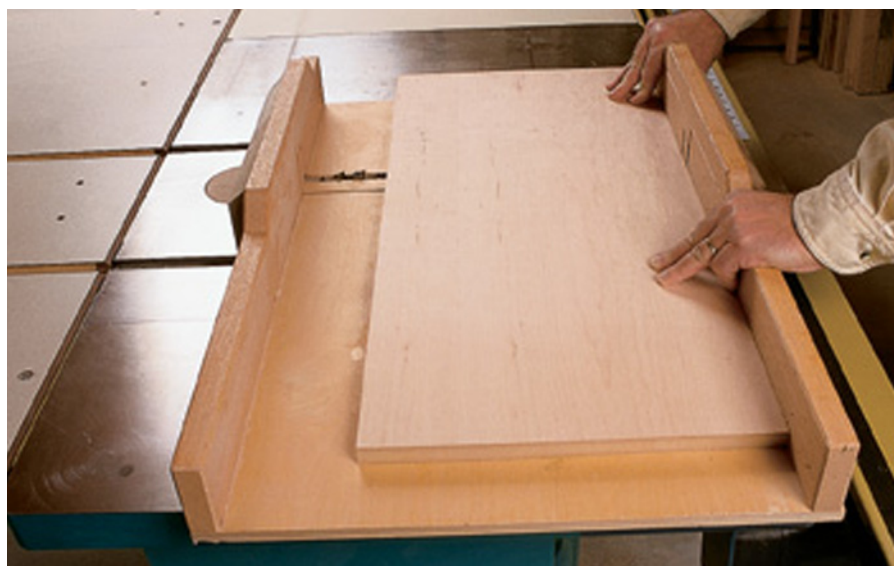
An accurate, shop-made cutoff box is the best guide accessory to use for dadoing on the table saw. Set the cutoff box on the sled base, tight against the fence. The work won’t shimmy or shift out of position as you slide the box across the dado cutter.
