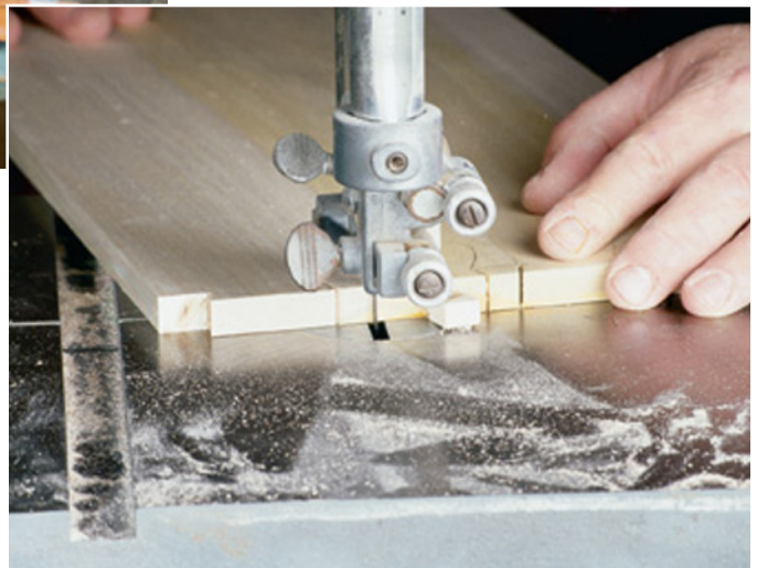
After I lay out the tails on the drawers' sides, I cut them out using my band saw.
