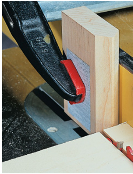
This simple jig can be used as a stop anywhere you have a fence. And you can micro-adjust the stop using the machine screw (top). On a table saw, this jig is great for stop-cuts (above). On the drill press, repetitive operations (such as drilling mortises) are easier with this handy shop helper (right).
