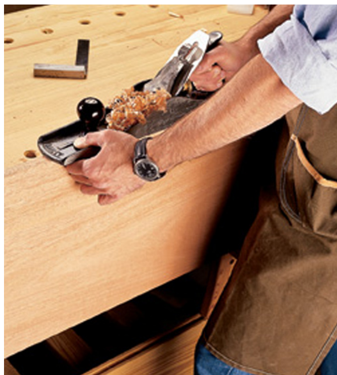
If you don't own a jointer, a jointer plane, such as this #7, can joint a perfect edge. It takes a bit of practice, but is not as difficult as you might think.
