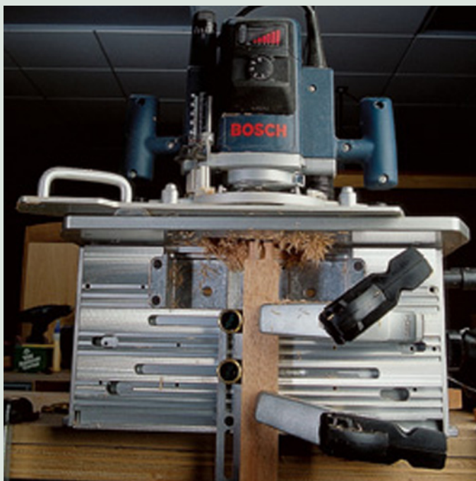
With the assistance of your plunge router, you can cut almost any mortise-and-tenon joint with this new jig from Leigh Industries.
