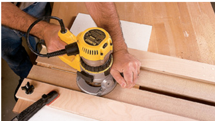
The gap between the fence bases on my dadoing jig represents the cut width. Pinch scraps of the work material between them to set the jig.
