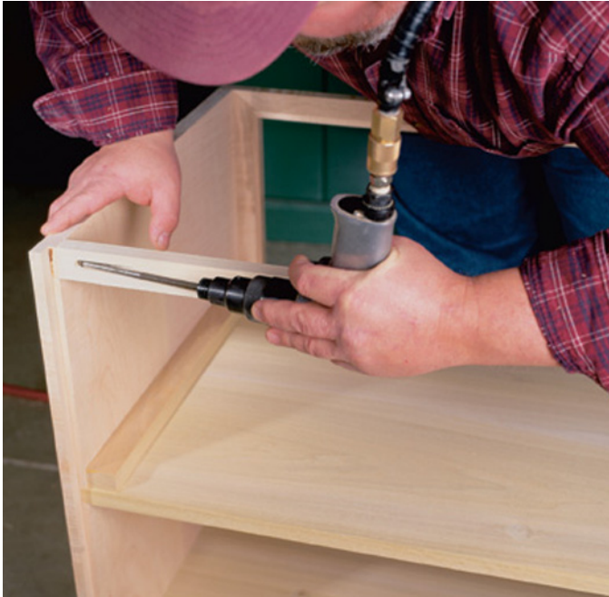
The bottom case uses a screw board to help support the top case and hold the back in place. Here I'm screwing the screw board to one of the bottom case's sides, flush to the inside edge of the rabbet.
