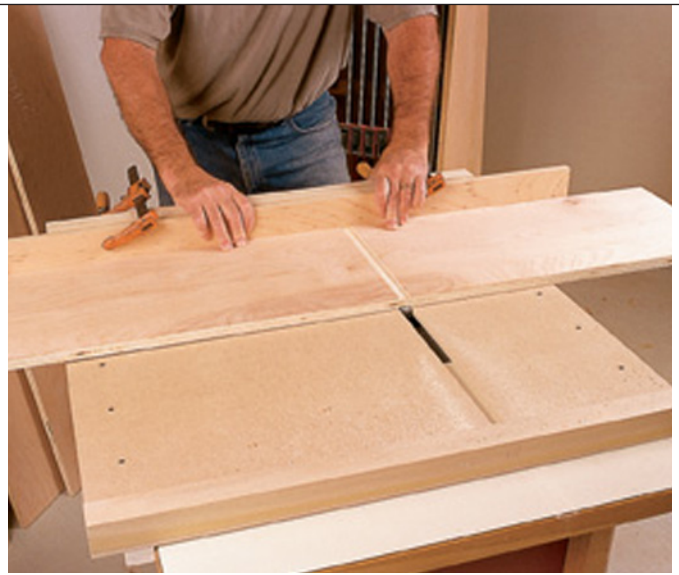
Dado large workpieces on a router table with a cutoff-box-like sled. A stop clamped to the sled's fence locates the cut and immobilizes the work. Slides on the underside reference the edges of the tabletop to guide the sled.
