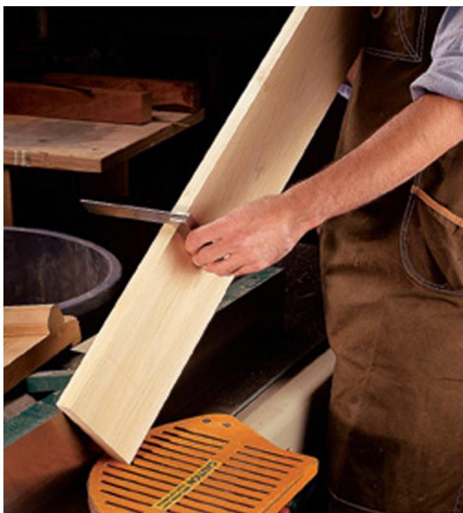
Joint all your edges before gluing up a panel. Some people like to use a "sprung" joint that has a slight bow in the middle. I find it unnecessary.
