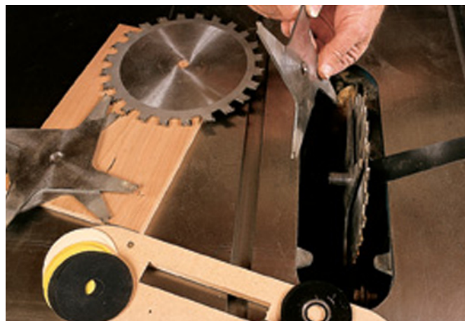
A dado stack set consists of separate blades, chippers and washer-like shims. You fit the elements onto the saw’s arbor, one by one.
