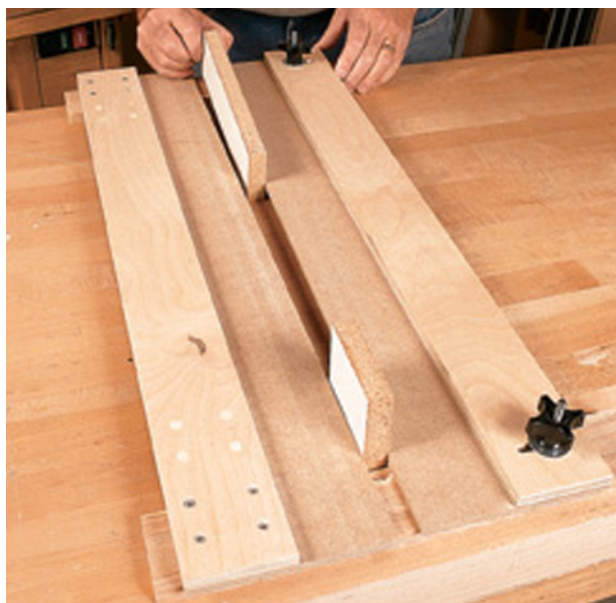
The gap between the fence bases on my dadoing jig represents the cut width. Pinch scraps of the work material between them to set the jig.
