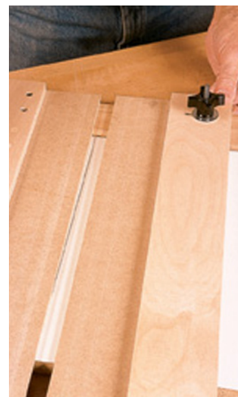
Position the jig by setting the fence base edge directly on your layout line. The crossbars ensure it will be perpendicular to the reference edge.
