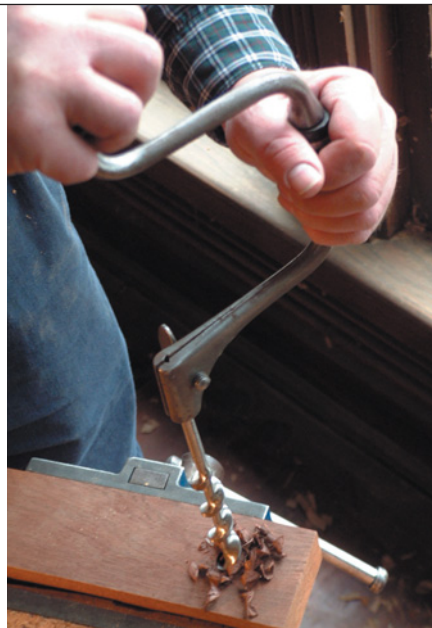
The brace and bit produces immense amounts of torque that your cordless drill could only dream about. Plus, many models (not the one shown here) have a ratcheting feature that allows them to be used in corners and right up against wall moulding.
