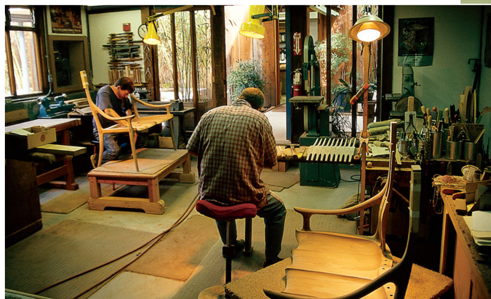
In the fitting room, Johnson (at left) and White use a variety of hand sanding and sculpting tools to final-fit the pieces. A 14" band saw stands handy, and a large and small lathe are available for any turning needs. The photo above shows the lathe tools and some spindles ready to be fit into the back splat.
