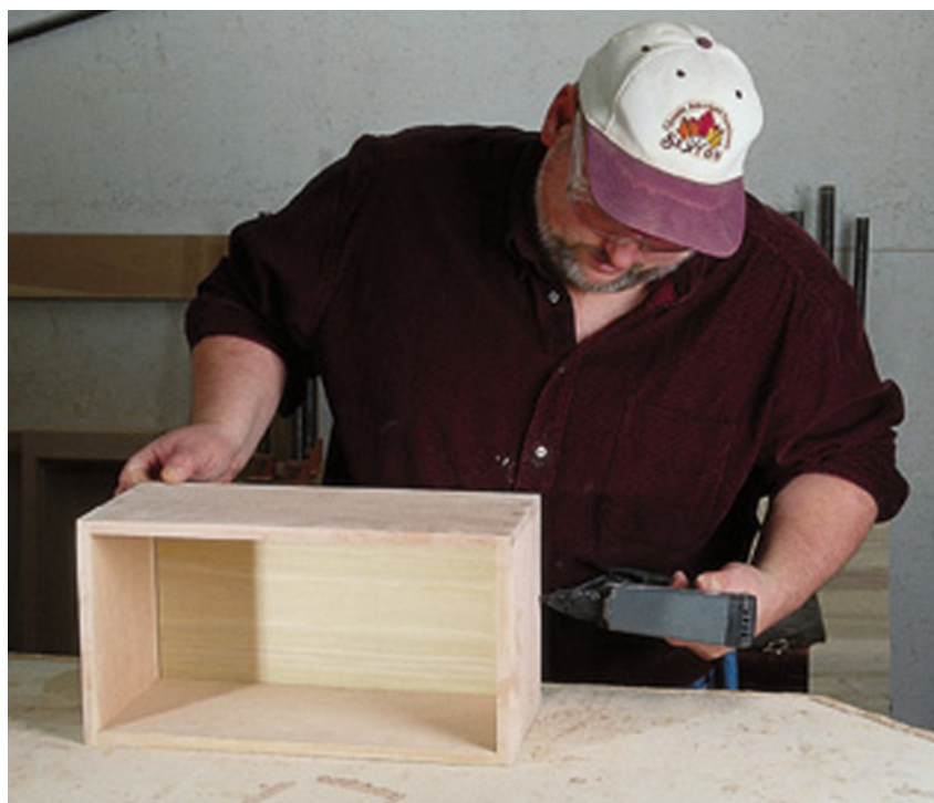
The bottom piece is small enough that wood movement isn't much of an issue. I simply nailed it in place.
