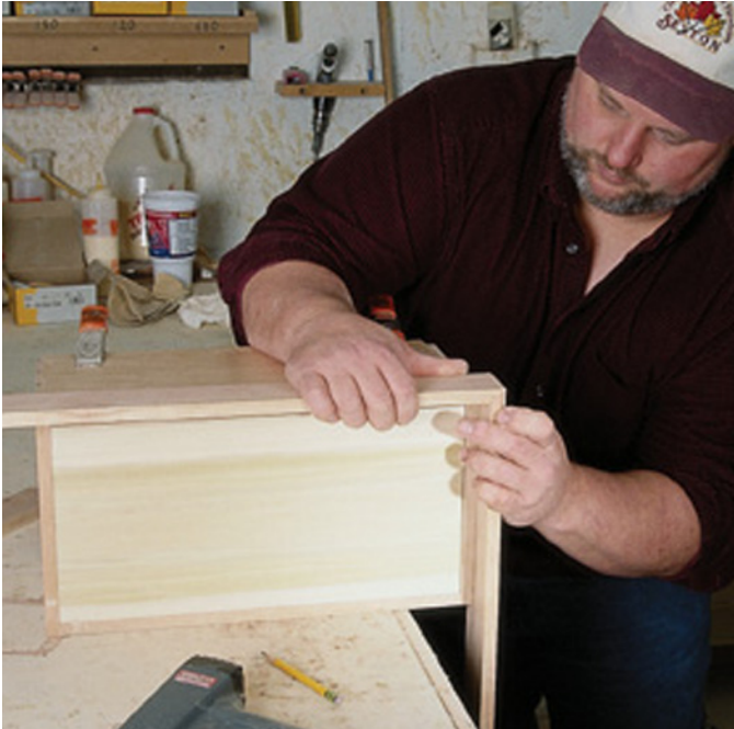
When mitering the base moulding, first cut a couple miters and check to make sure your saw is set for the right angle to make an airtight fit.
