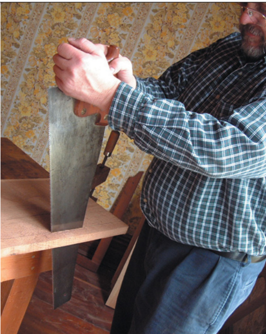
Handsaws might seem like an antiquated way to size lumber, but a straight and sharp saw is highly effective (and a joy to use).
