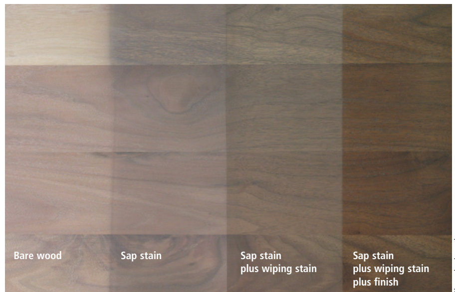
Figure 5: A more effective method of blending sapwood with heartwood is to apply a sap stain (first colored column from the left), then apply a walnut wiping stain and finally apply a finish.
