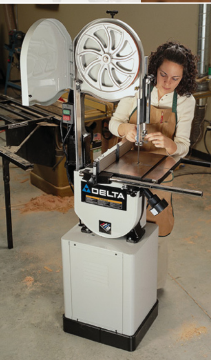
The traditional cast-iron band saw, with riser block.
