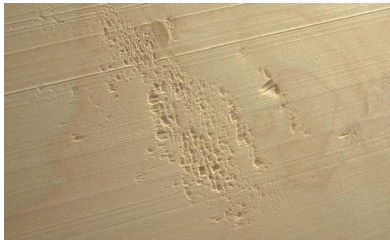
This is what tearout looks like. Avoid it. When a finish is applied, it looks terrible.
