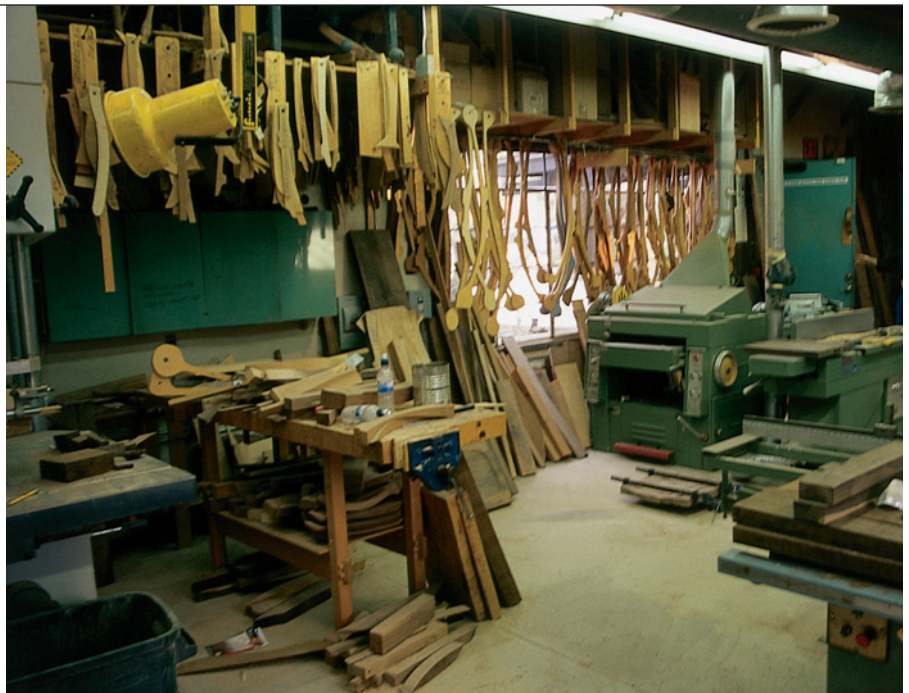
In "Sam's shop" (more accurately the machining room) templates for a dizzying array of chair designs line the wall. Standing at the ready is a 20" planer, 12" jointer and tucked in the left of the photo is a Laguna 20" band saw, one of four band saws currently in the shop.
