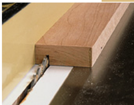
Saw a rabbet on the table saw in two steps. Set the blade elevation and fence position first to cut the shoulder (above) then adjust either or both as necessary to cut the bottom.
