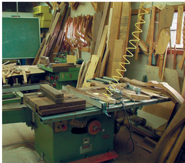
On the opposite side of the room above is a 12" table saw and heavy duty shaper. More templates adorn the walls (they're fixtures in most of the rooms) and a chalkboard and props stand at the ready for weekend lectures where Maloof walks attendees through the construction processes of one of his chairs.
