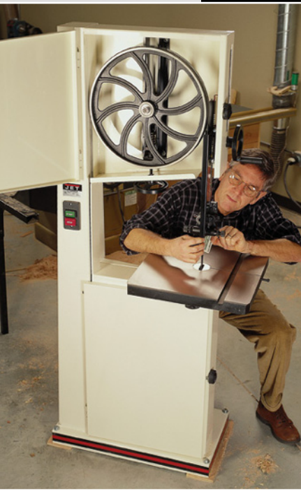
A steel-frame band saw, built for resawing.
