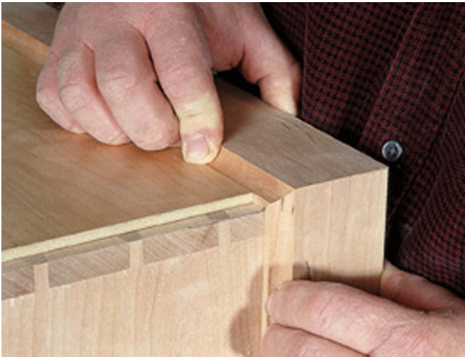
Once your miter is cut, check the fit before adding the glue and nails.
