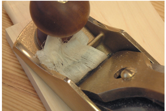
See how the shaving emerges only in the middle of the iron? That's how you know your iron is sharpened and set correctly.
