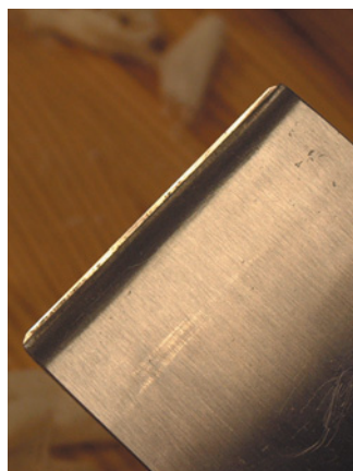
For smoothing work, position your chipbreaker between 1/32" to 3/32" from the cutting edge.
