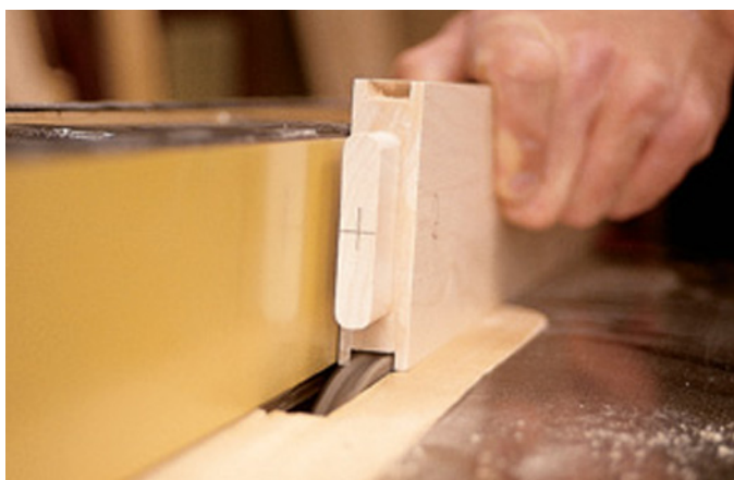
After the tenons and mortises are cut on all your parts, rough out the grooves for the panels using a dado stack in your table saw.
