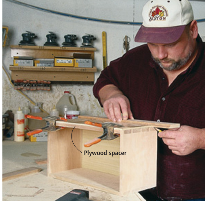
Clamp a plywood spacer to the front that positions the base moulding exactly where you want it. I always find the cut line for my miters by placing the work on the piece and marking from the underside as shown in the photo. This is more accurate than measuring.
