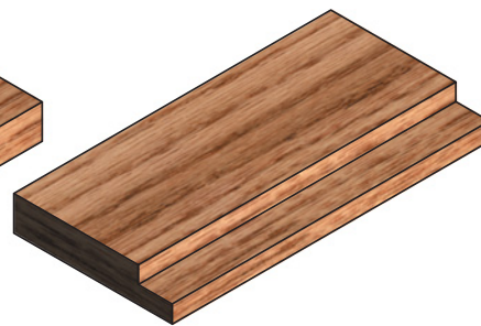
Saw a rabbet on the table saw in two steps. Set the blade elevation and fence position first to cut the shoulder (above) then adjust either or both as necessary to cut the bottom.
