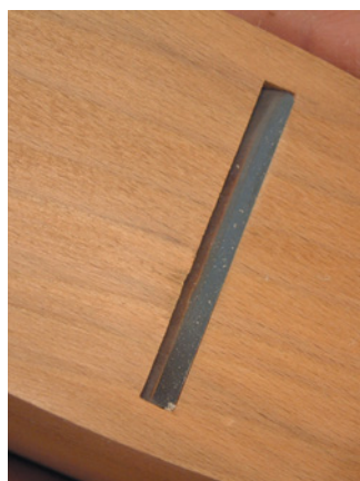
Take a look at the throat on this Clark & Williams coffin smoother. See it? Neither can we. This is a tight mouth.
