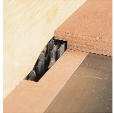
Clamp a sacrificial facing – a strip of luan plywood here – to your table saw fence when cutting rabbets with a dado head. Run the cutter up into the facing, exposing only enough of the cutter to form the rabbet.
