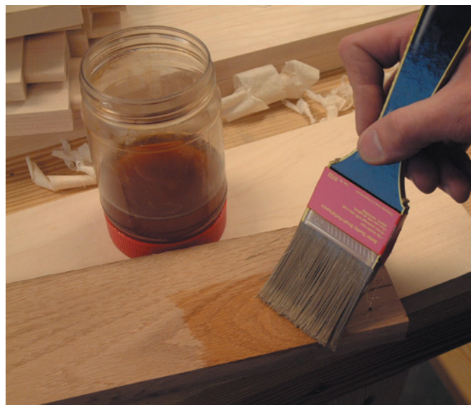
A little shellac on a problem tearout will stiffen the wood fibers and allow them to be sheared cleanly – sometimes.
