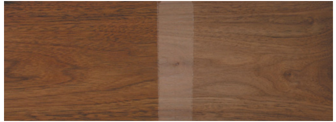
Figure 2: Varnish applied to the left side of this walnut board adds a warmer coloring than does water-based finish applied to the right side.
