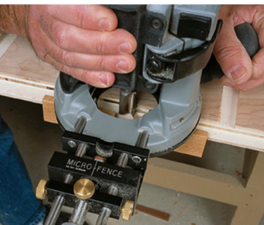
With an edge guide and straight bit, you can customize the rabbet's width, forming it in a series of passes.
