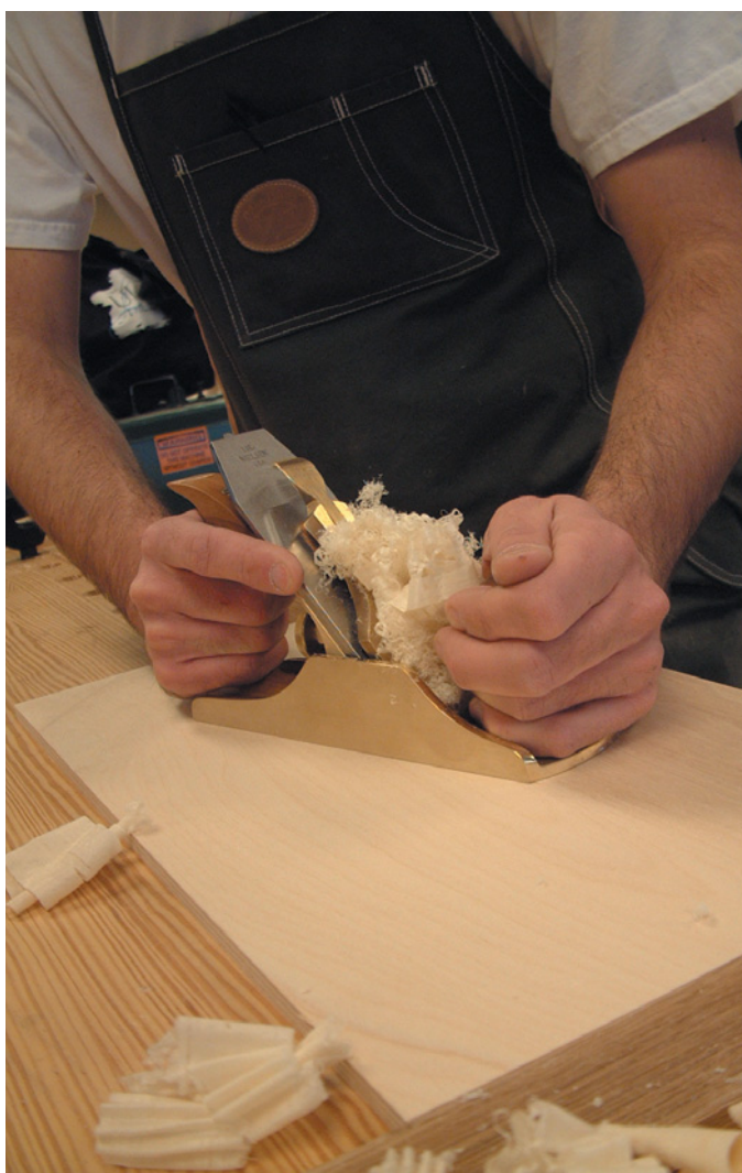
Skewing the plane body during the cut can help in tricky grain situations.
