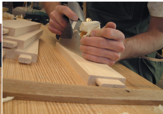
A shop-made planing stop is a simple and effective way to hold your work for smoothing (left). The force you use to push your plane also holds your work down and against the stop (above).
