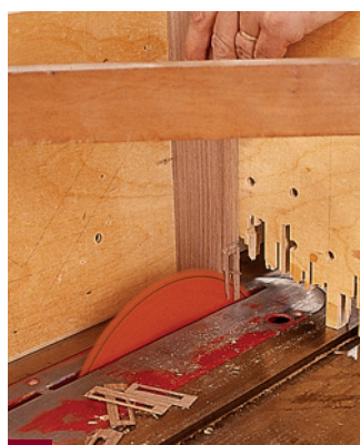
7 Use a tenoning jig to remove the waste material where the top and bottom rails meet the stiles.
