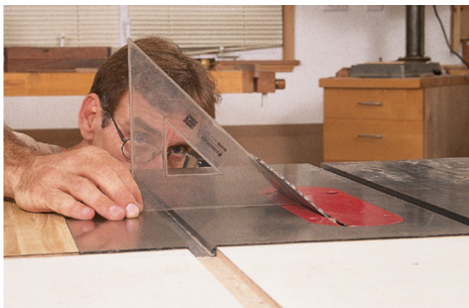
A 45° drafting triangle, which you can find easily and is affordable, is a great tool for adjusting blade tilt stops.
