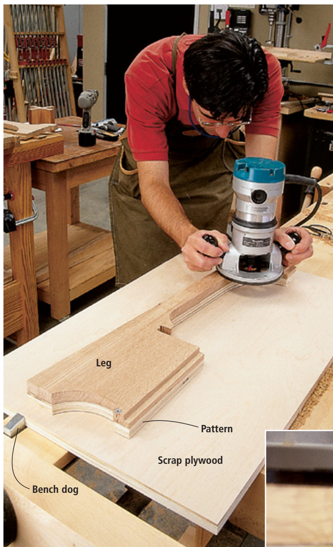
I nailed my pattern to a piece of scrap plywood and clamped that to my bench. This made routing the leg a simple operation that could be done in one pass.
