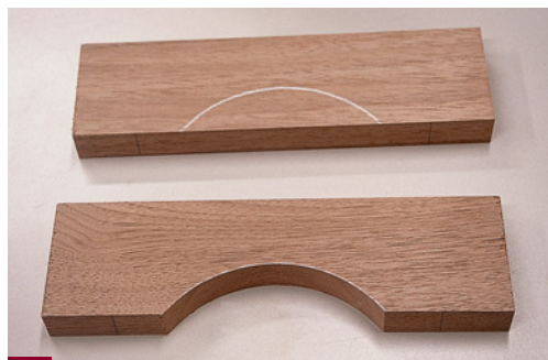
5 Cut the door pieces to size, lay out the radius on the top rail and create the tombstone effect. To do this, you will want to use a \frac{3}{16} " roundover bit on the inside edges of your pieces, making sure to run both edges on the middle rail of each door.
