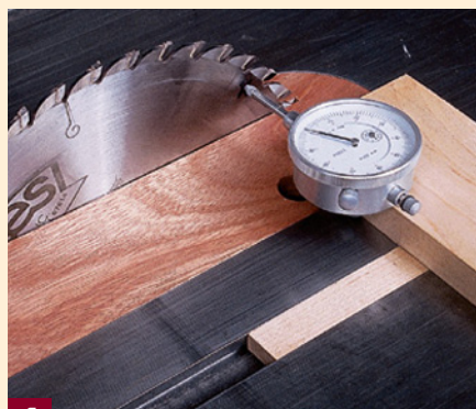
1 Mark the blade and rotate it fully forward to pre-load the dial indicator plunger against it. Then zero out the dial indicator.
