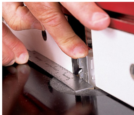
Align the outfeed side of the fence even with the cutting edges of the bit's smallest diameter. Use a straightedge and turn the bit by hand to find the correct alignment.
