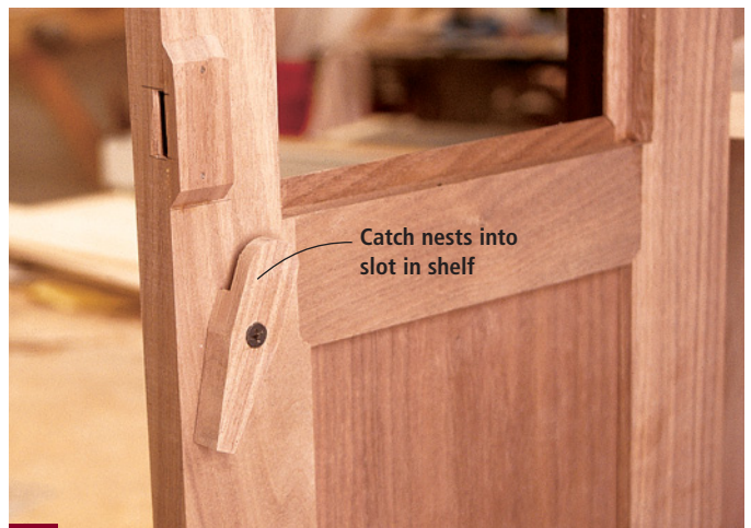
17 Using a biscuit joiner, make a groove in the bottom edge of the shelf, just behind the stile and 1/4" from the shelf front, to accept the door catch. Next, mark the location of the lock strike and create a catch. It is also possible to purchase an angled strike plate from the lock supplier to eliminate this procedure.
