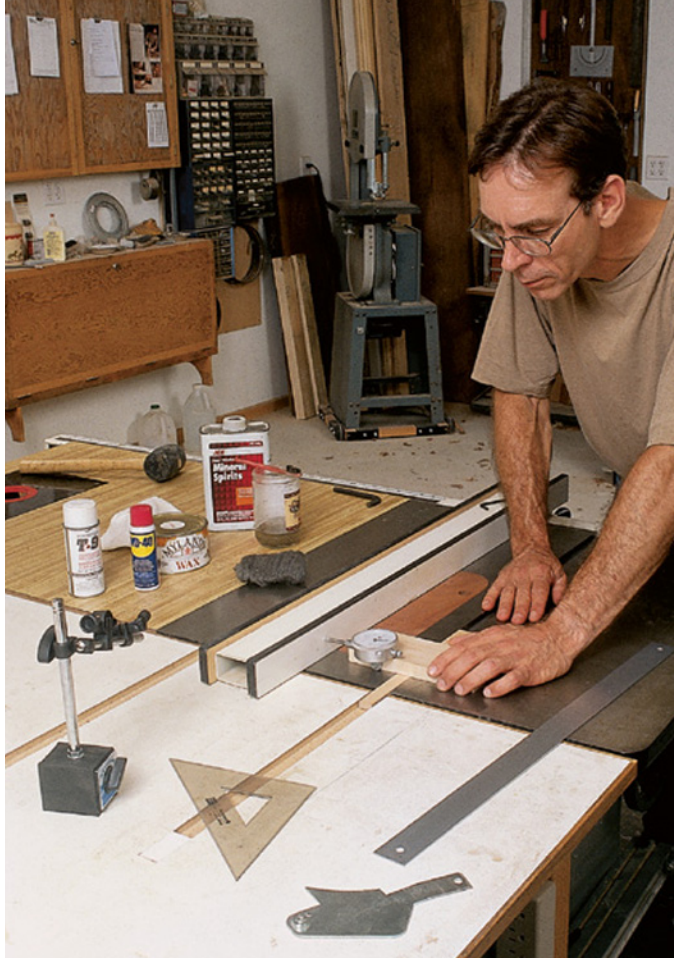
None of the tools needed to tune up your table saw are expensive. Here I'm checking the parallelism of the fence to the miter gauge slots using a $14 dial indicator.
