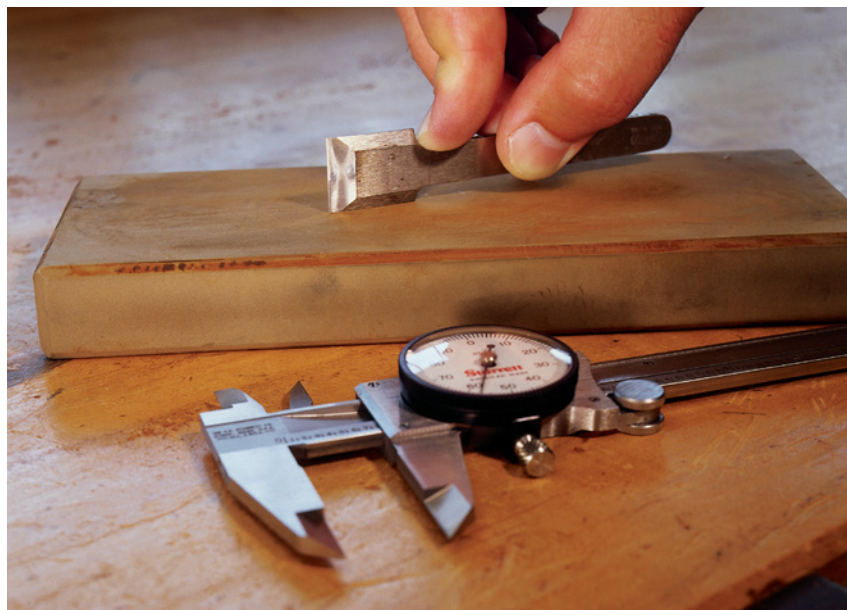
Your iron should be .006" to .010" wider than the sole. To get your iron to this width, carefully work the sides of the iron with a coarse bench stone. Check your progress with a dial caliper.
