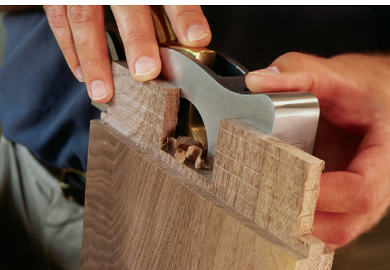
When planing end grain, as I'm doing here, be careful of splintering the grain at the trailing corner of the stock. To avoid this, simply plane from both directions and allow the cuts to meet near the middle.
