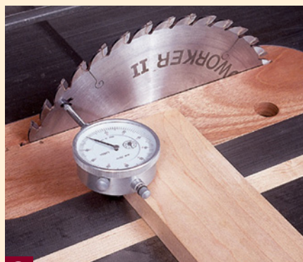
2 Rotate the blade mark to the rear, then slide the dial indicator back until the plunger rests against the mark.
