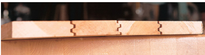
For the routed glue joint, mark the center of the work and align the sweet spot on the glue-joint bit with your mark. It probably won't be perfect, but it'll get the setup process started.
