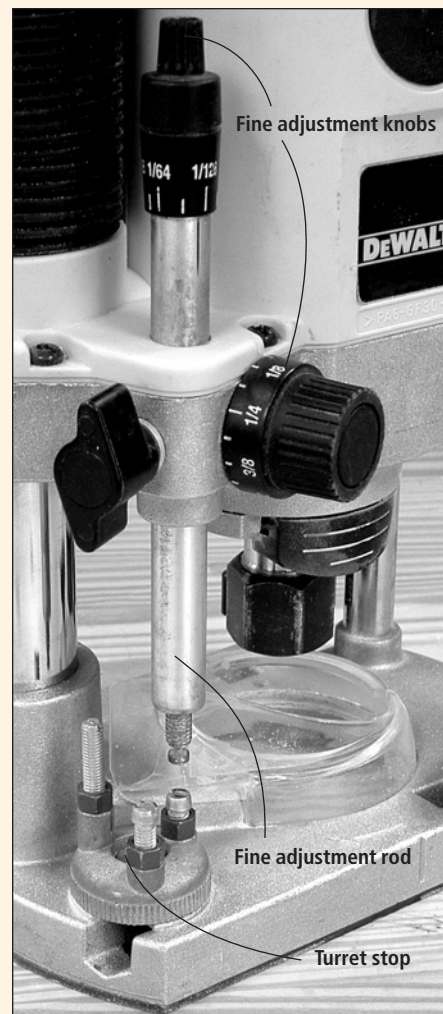
The fine-adjustment knobs make the depth as accurate as possible.
