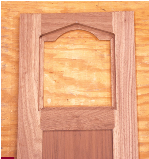
13 This is how the glass area should look after routing.
