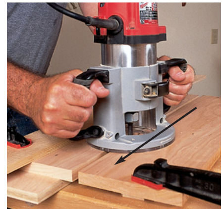
Position the mating board opposite the first, with a gap just smaller than the diameter of the bit between the two workpieces. The feed direction when routing the second edge is left-to-right.
