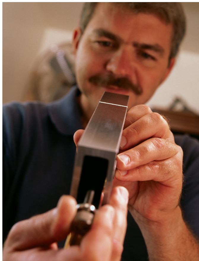
Once your iron is ready for cutting, install it in the plane and adjust it for a very light cut. Simply sight down the plane and slowly advance the iron until you can see just the edge.
