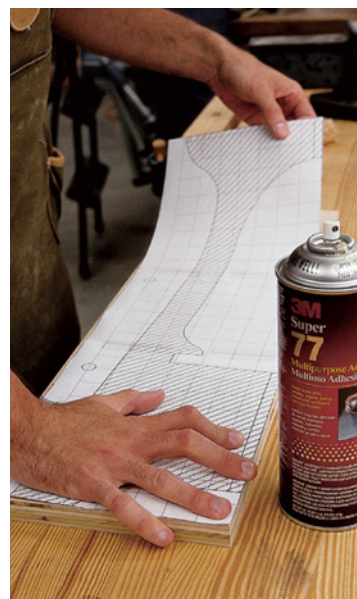
With the patterns taped together, attach it to a piece of plywood using a spray adhesive. This 3M product is available in the glue section of most home-center stores.
