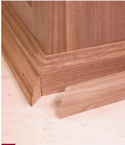
14 Using a 1/2" beading bit to form the edge of the Stage 2 base moulding, create the piece and nail it to the Stage 1 moulding.
