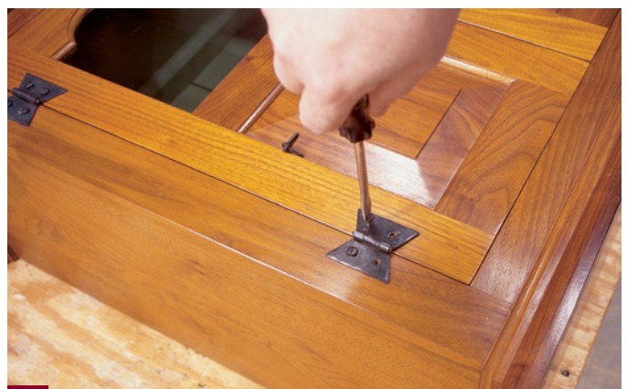
18 Install the glass. Reattach the hinges, reinstall the lock and apply a coat of paste wax. And with that, your cupboard is done.
