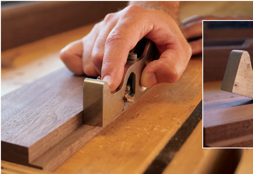
Some shoulder planes, such as the Stanley #92 shown here, feature a removable front piece, which transforms the tool into a chisel plane.
