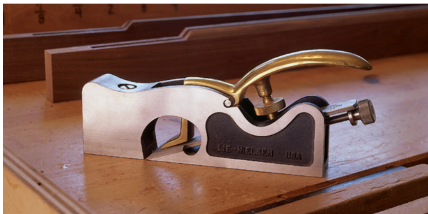
For fine-tuning joints, the versatile shoulder plane is a must-have tool in your shop.
