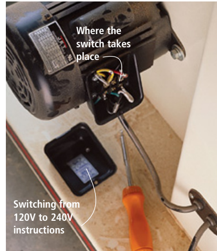
Most motors have a label that shows you how to switch it from 120V to 240V, as shown here.
