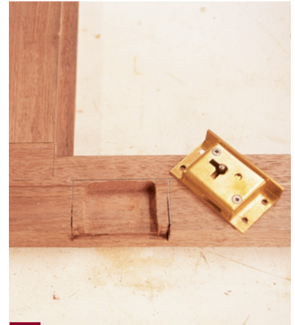
15 Install the lock into your door, then fit both doors into place and install the hinges, making sure to allow equal spacing around the doors.
