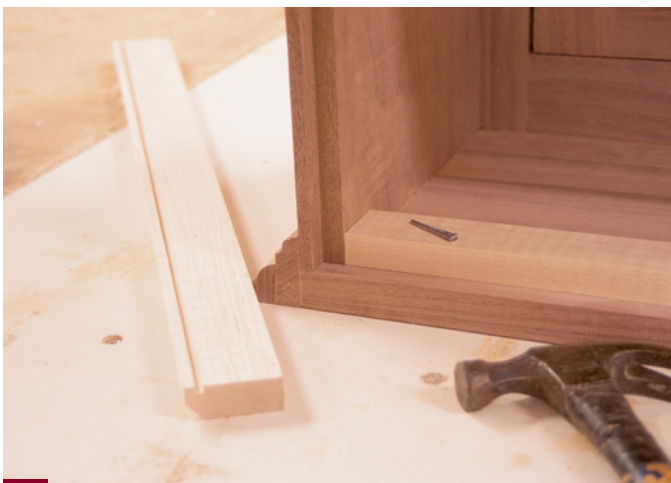
16 The backboard nailers are glued and nailed to the top and bottom of the case. Here you can see a groove cut into the bottom of the nailers, which will make sure to eliminate any glue squeeze-out.
