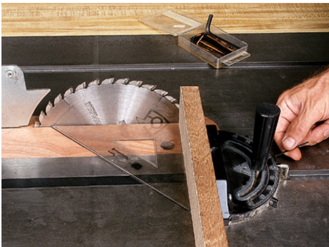
After adjusting the miter gauge square to the blade, set the stop on the gauge for accurate repeatability. A sandpaper-faced auxiliary fence allows for greater control when crosscutting.
