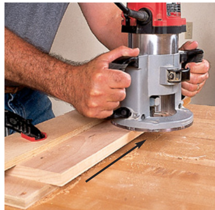
Rout the first half of an edge joint by guiding the router along a fence clamped atop the workpiece. The feed direction here is right-to-left (moving away from the camera).
