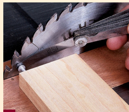
3 As a low-tech alternative to a dial indicator, you can use an automotive feeler gauge to check the gap between the blade and a screw driven into the jig.
