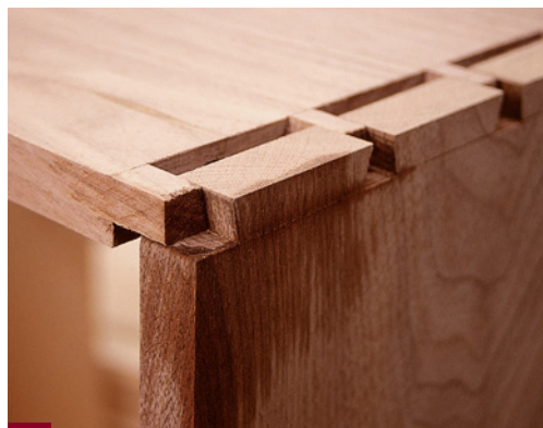
1 Using the pins, lay out and then cut the corresponding tails into the side pieces.
