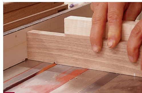
6 Set the saw blade to 45° and cut to the shoulder of the roundover location. There is one cut each for the top and bottom rail and two cuts for the middle rail. The area for the middle rail is nibbled away and cleaned up with a chisel.
