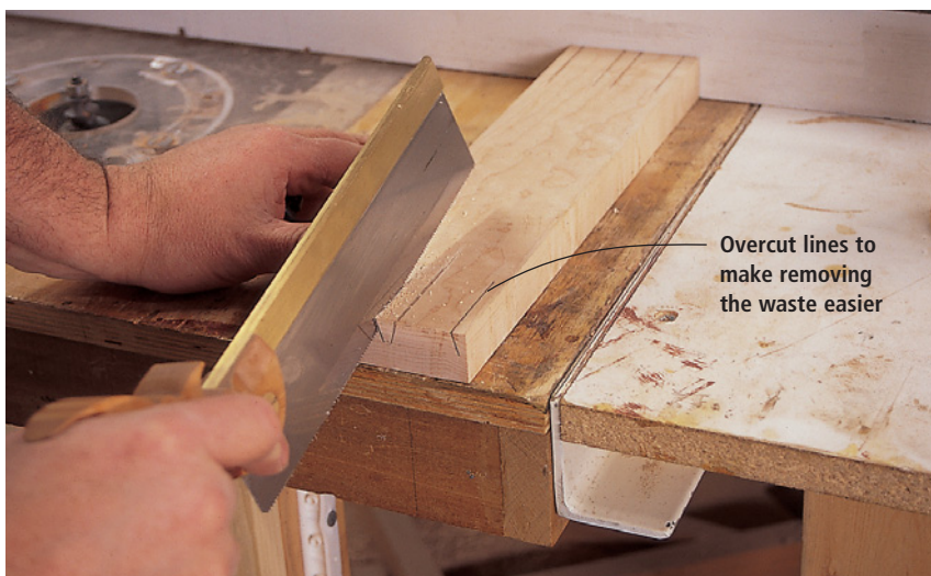
Begin building the drawer by laying out the dovetails on the drawer front. Cut the lines down to a line scribed \frac{1}{16} " from the inside of the drawer front. Overcut toward the center of the interior face of the front. A front this size has two full tails, one pin and two half pins.
