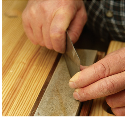
If you stone the edge freehand, bow the tool slightly to keep it flat on the sharpening stone.
