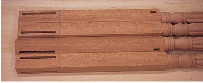
Mark and cut the mortises for all the rails. Also, you can see the finished carving from the previous step.
