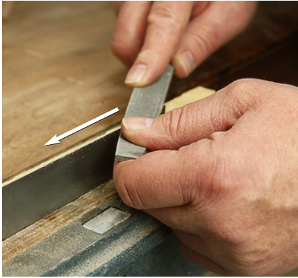
To drawfile a scraper edge, hold the file at an angle as shown and push it across the tool's edge. Cut only on the push stroke.
