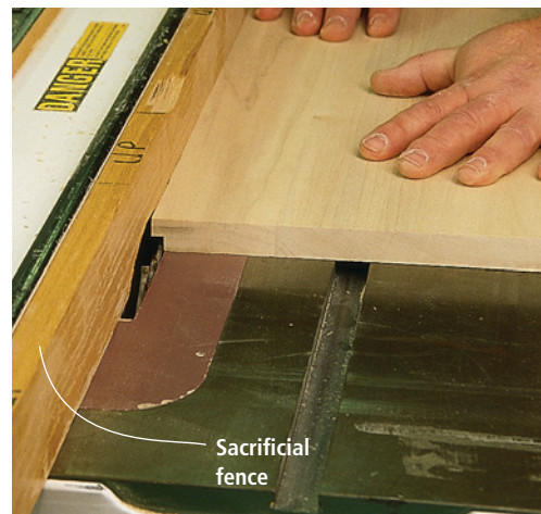
After resetting the dado height and adding a sacrificial fence to my rip fence, I was able to cut the rabbets for the back on each side.
