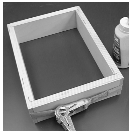
A band clamp helps hold things tight as the glue cures. Just make sure everything is square before you leave it to dry.
