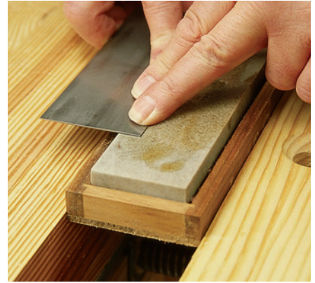
After the edges are polished, you can hone the faces of the scraper, as shown.
