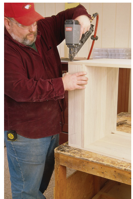
Nail the other two braces in place below the bottom. The braces help square up the cabinet as you attach them – assuming they're cut square.
