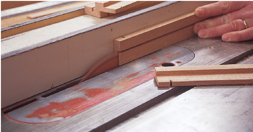
Cut the rabbet on the lower rails in two passes on your table saw. Define the shoulder, then set the fence to \frac{1}{4} " and raise the blade to remove the \frac{7}{8} " waste. This produces an L-shaped profile.
