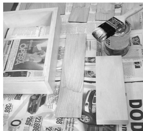
Use contact cement to adhere the laminate to the plywood. I prefer the water-soluble variety because it's easy to brush on, and it cleans up with soap and water.
