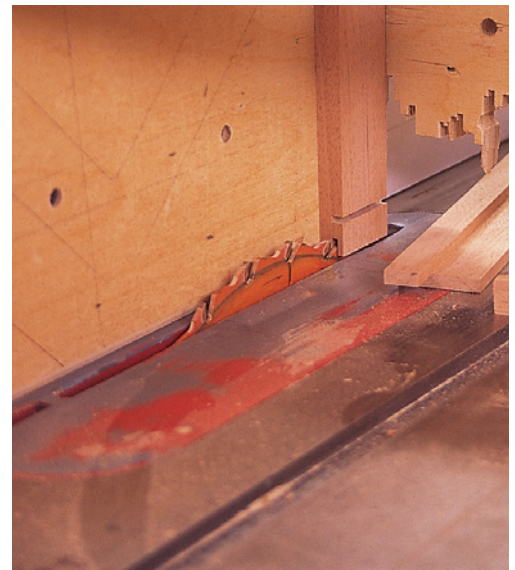
Next, make the cheek cut that leaves the necessary \frac{1}{4} "-thick x \frac{3}{4} "-long tenon on the ends of the lower rails.
