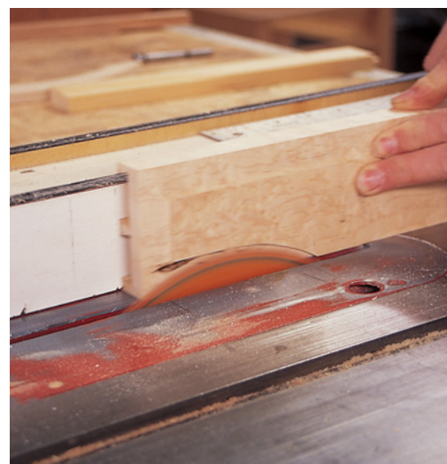
With the drawer apart, set the saw blade's height to \frac{3}{4} " and cut a rabbet in the front on all sides, creating the shoulder for the crossbanding.
