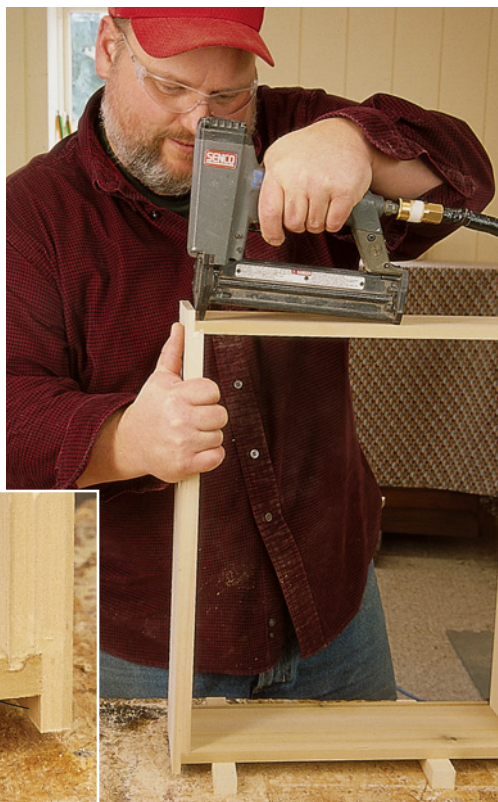
Large rabbet cut before drawer-lock joint
