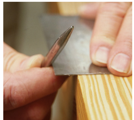
Finally, to turn the hook, tilt the burnisher 8° to 10° and rub the edge with light pressure.
