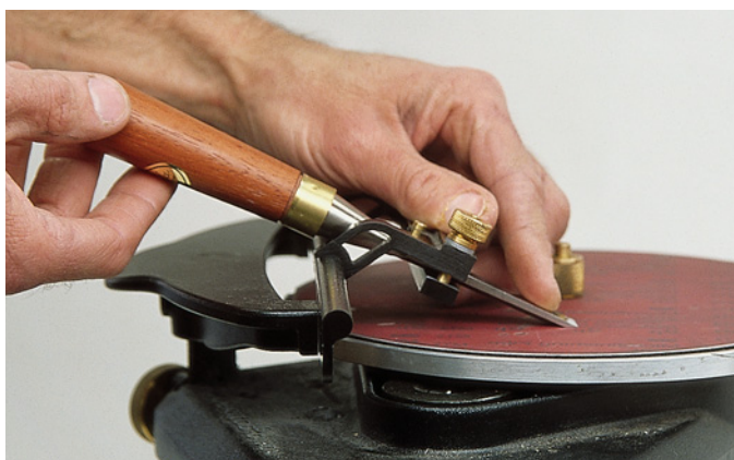
Light finger pressure is all it takes to hone a polished edge quickly and easily on the Veritas machine.
