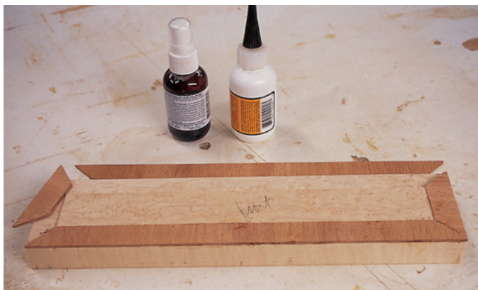
Cut the crossbanding on the band saw, noticing the grain direction, and fit to the drawer front with mitered corners. Use cyanoacrylate glue to bond the banding to the drawer face.
