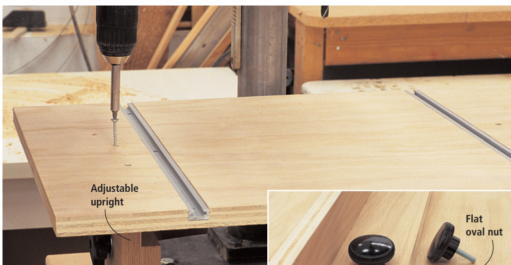
Attach the plywood table, with the tracks already installed, to the adjustable uprights with screws. Secure the fence to the T-tracks using knobs with a threaded shaft and flat oval nuts (right).
