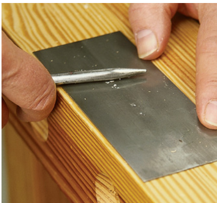
The first step in burnishing is to consolidate the edge by running the burnisher flat on the face.
