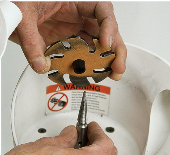
The 3M Trizact sandpaper is attached to plastic discs (called Ninja Disc Backpads) that screw onto the machine's spindle. Swapping discs is fast and easy.
