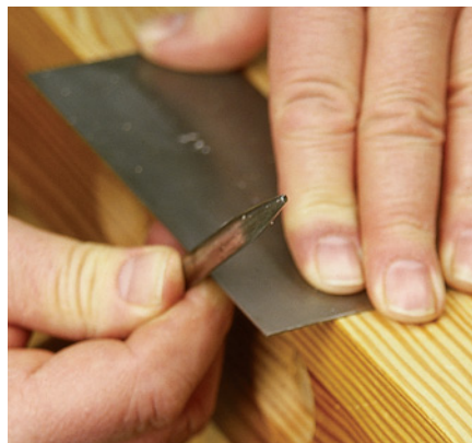
Next hold the burnisher square – perpendicular to the face – and rub the edge.
