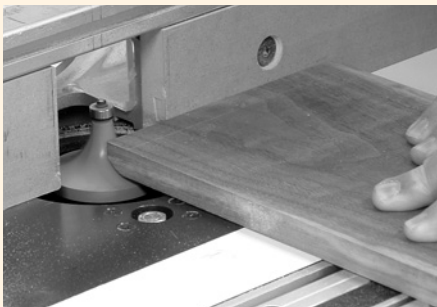
When you're ready to shape your workpiece, first cut the end grain along the ends ...
