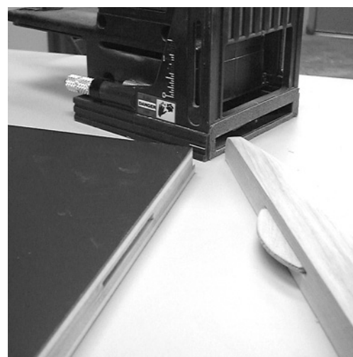
Before installing the handle, cut slots for a single biscuit in the center for added strength.
