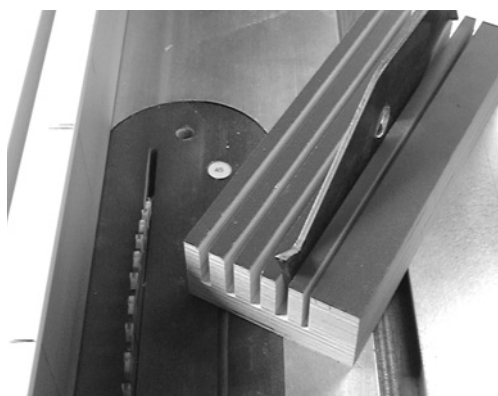
The chipper block simply is two pieces of 3/4" plywood face-glued together, with a series of evenly spaced 1"-deep slots for the chippers.
