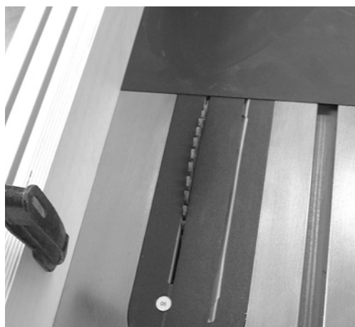
To cut the laminate, I used my table saw with a long board clamped to the fence. This board prevents the thin material from slipping underneath.
