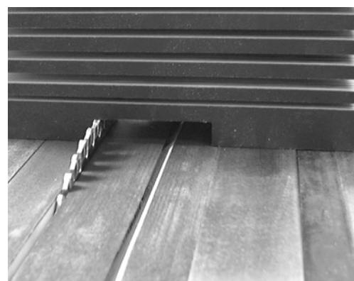
Nibble away a pocket for your collection of blade shims using your table saw.
