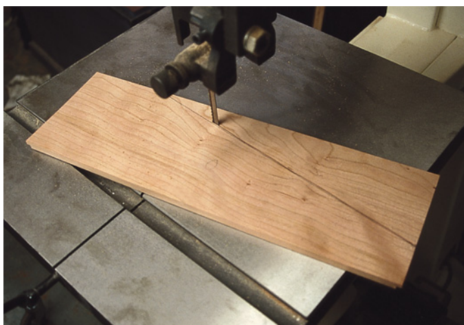
After carefully laying out the angle locations on both sides, use the band saw and cut about \frac{1}{16} "-wide of the line to allow for accurate trimming.
