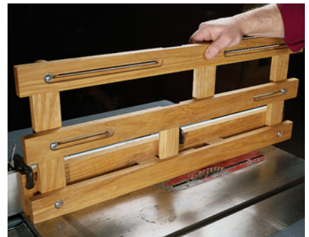
With all parts extended and the screws retightened, the fence is now 12" tall.
