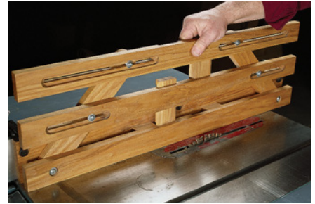
Just loosen the machine screws and the fence can be adjusted to any height.
