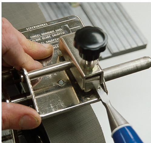
On the JET JBGS-82, set the angle of your tool's bevel by lining up its front edge with marks on the jig. Three common angles (25°, 35° and 40°) are called out.
