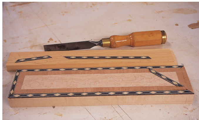
Repeat the process to install the decorative banding.
