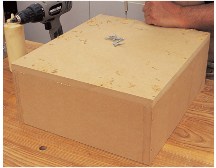
A bottom that's cut square will help keep the drawer parts aligned.
