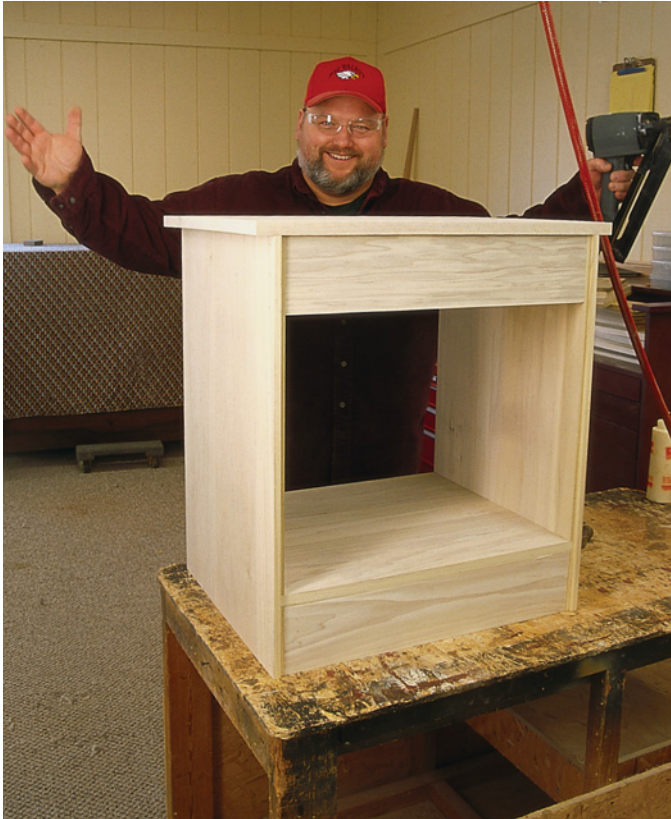
The carcass is essentially complete. All that's missing is the back, which I leave off until after I paint it and install the drawers.
