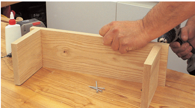
Build the adjustable table's support with hardwood and screws.
