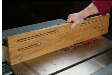
The fence is 6" tall when contracted and can be used with any machine that has a fence.
