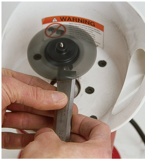
The plastic discs' shape allow you to see the tool's edge as you grind and hone it. Shaping unusual tools is remarkably easy.
