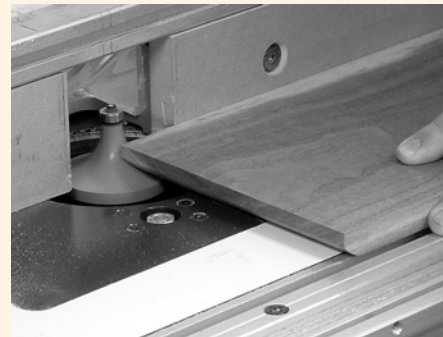
... then cut the long grain along the edges.
