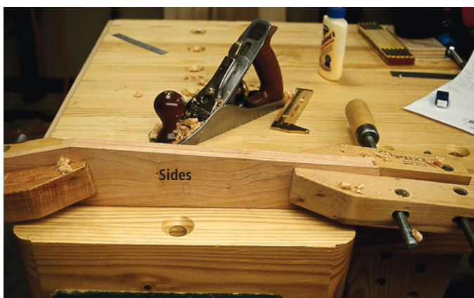
To clean up the band saw cuts and ensure they're identical, clamp the two sides together and use a bench plane to clean them up simultaneously.
