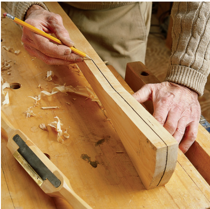
Using your pencil held as shown, trace a centerline on all edges.
