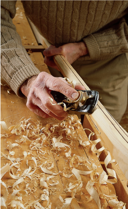
The block plane will quickly smooth all the edges into a 1 1/16" x 1 1/4" oval, as I'm doing here.
