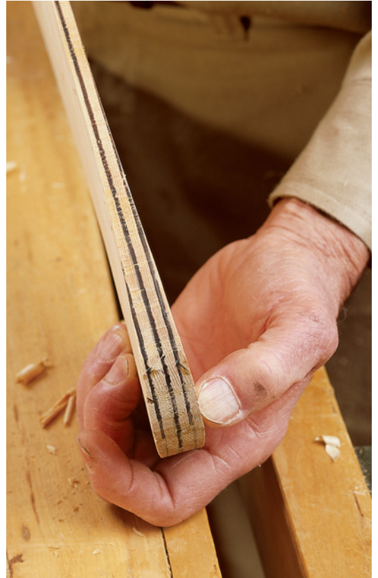
The point of the blade is left thicker ( \frac{5}{8} " ) to reinforce the point where splits are possible.
