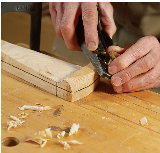
A block plane will round over a comfortable end. The profile shows well here.
