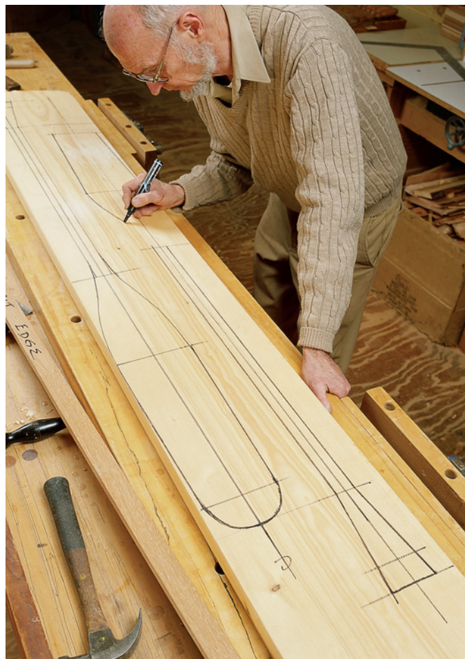
Layout involves transferring the dimensions from the plans. The centerline with cross lines indicate the major points. Connect the straight lines, then sketch in the curved transitions.
