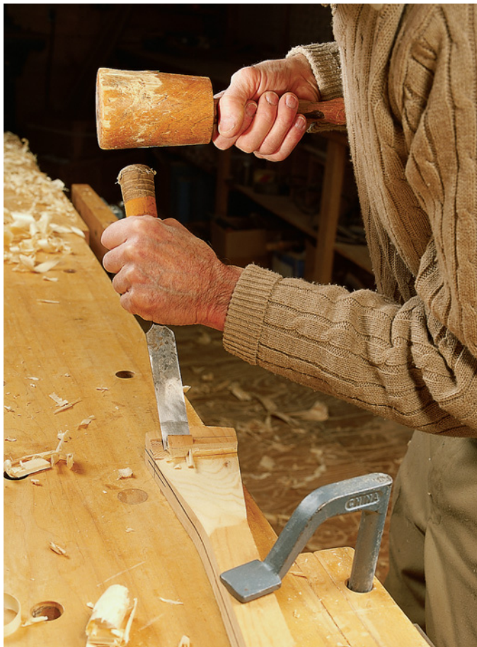
Chisel a hollow approaching the saw kerf. Beware that two cut lines like this can be difficult to blend smoothly. Before cutting too far, expect to clean it up with a rasp and sandpaper.
