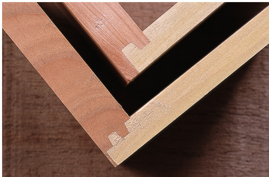
Two ways to cut a drawer-lock joint: The joint at top was made using a drawer-lock bit; the one at bottom was made using a miniature glue-joint bit. Both are strong and quick to make.
