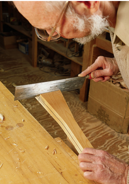
Saw down to a point on the handle, leaving \frac{3}{8} " for the grip.
