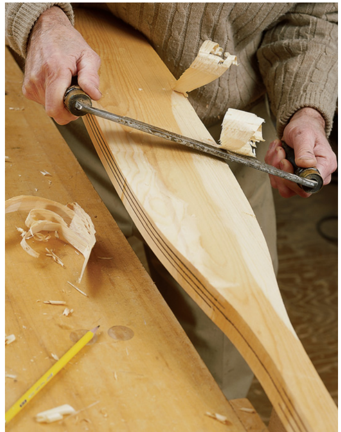
Use a drawknife to rough the blade to thickness. Bevel the edges first as shown, then take down the center. It may be tough using this tool, so try to hold it the way the photo shows. This should ease the struggle a bit.
