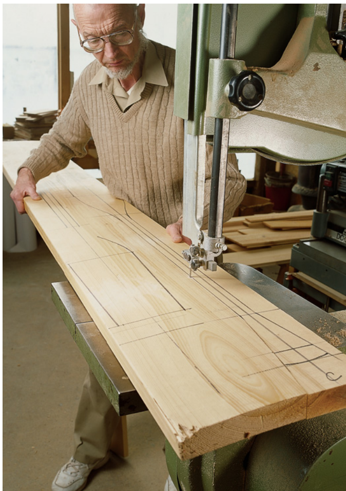
After planing the plank to 1¼" thick, band saw the paddle blank to shape.
