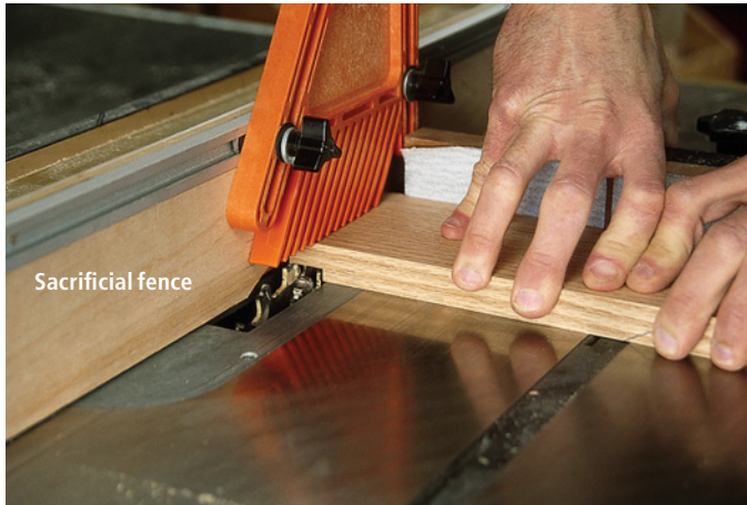
With the sacrificial fence in place, this setup will allow you to cut the rabbet in one pass. This eliminates the need for multiple saw setups and you don't need to stand your work on edge to make the cut.
