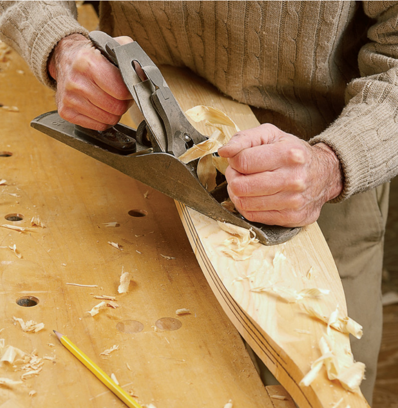
Use the bench plane to smooth the blade to its final \frac{3}{8} " thickness. The pencil lines on the edge should give you guidance in this step.
