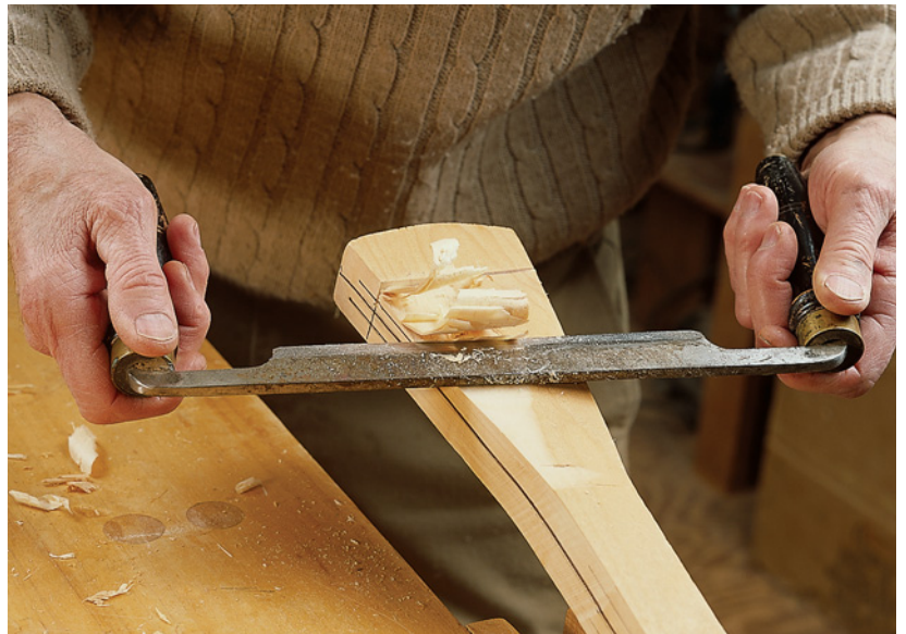
The drawknife removes waste as you approach the saw kerf at the handle.
