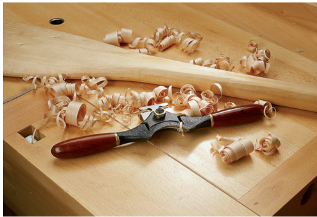
A spokeshave with a concave sole, such as this one from Veritas, excels at rounding the shaft of the paddle.
