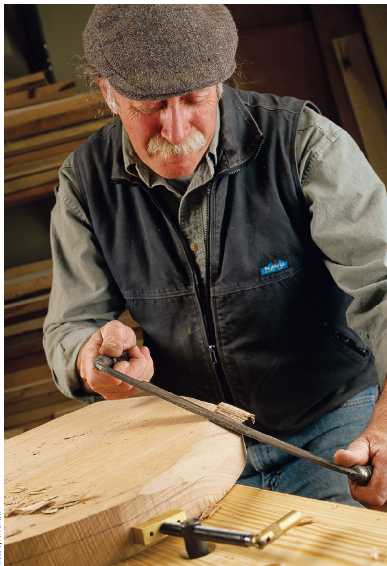
Chairmaker Don Weber works on an American elm seat blank with a drawknife. Elm commonly is used in chairs because of its inherent strength.
