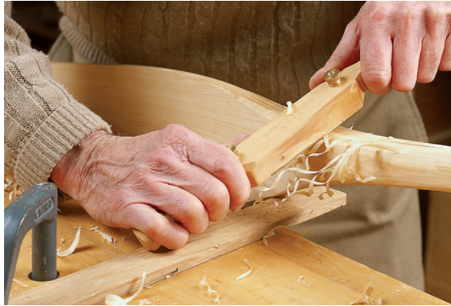
The spokeshave (I'm using a wooden one here) is used to smooth the transition between blade, shaft and handle. It works pulling or pushing to follow the direction of the grain.
