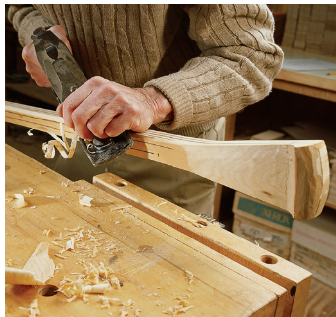
The shaft is planed into an octagon following guide lines.
