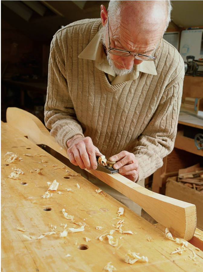
Smooth all the paddle's edges with a block plane. If any lines don't look fair to you, planing can make them so.
