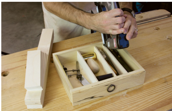
Install the dividers in the drawers so they can be easily removed in the future. A 23-gauge pinner is an excellent tool for this job.
