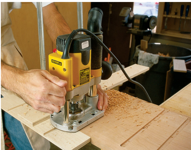
The shop-made T-square jig and a plunge router make quick work of the dados.
