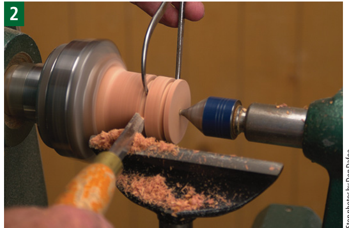
2 If a chuck is used, turn part of the block to round, then use a parting tool and calipers to establish a rough diameter dimension, which is the finished dimension plus 1/16", in this case about 1 11/16".
