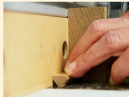
The wood to be milled should slide easily through the notch. Hand pressure on each side ensures an accurate cut.
