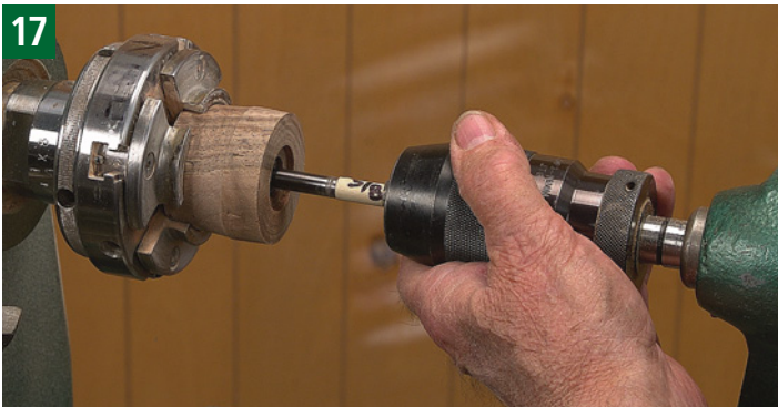
17 Select a block of wood for the roof. The procedure for roughing out the block and turning it to the required dimension is the same as shown in steps one through five for turning the body of the ornament. The only difference is the dimensions needed, and they are given on the drawing of the roof. For a basic roof, the block needs to be 1\frac{5}{8} " long and 1\frac{7}{8} " in diameter. Drill a 1" hole that's \frac{1}{8} " deep to provide a counterbore area for the top of the body to fit into. Now drill a \frac{5}{8} " hole that's \frac{1}{2} " deep to allow the top to fit on the wooden mandrel. This also removes some of the wood in the top, making it lighter. Sand and finish the underside of the top.
