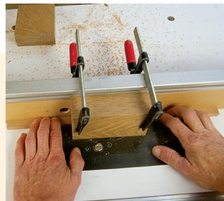
A block of wood surrounding the router bit lets you apply pressure to the table and fence close to the action, while protecting your hands.
