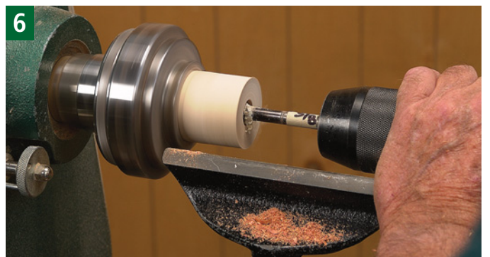
6 Insert a drill chuck into the tailstock and install a 5/8" Forstner or saw-tooth bit. Drill a hole 1½" deep. This will leave ¼" of wood in the base of the body. (Here I'm working on a different ornament. Remember how many I had to make? So I apologize for the species change throughout the article. But note that the steps are the same.)
