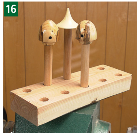
16 If any runs start to show, use the dowel to rotate the piece until the surface starts to set, then place the dowel in a holder until the finish is dry. Depending on humidity and temperature, the lacquer will be ready for a second coat in 15 minutes or so. When the finish is dry, the body is put back on the mandrel, the lathe turned on and the body is polished with #0000 steel wool and paste wax, then buffed with a flannel cloth.
