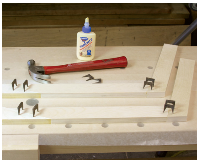
The first 3/4" layer of the legs is simply edge glued to form the shape. To gain some strength, I used pinch dogs. These large angled staples pull the two pieces tight across the joint with only a couple of taps of a hammer. Another good option is to use pocket screws – two at each joint should do the trick.
