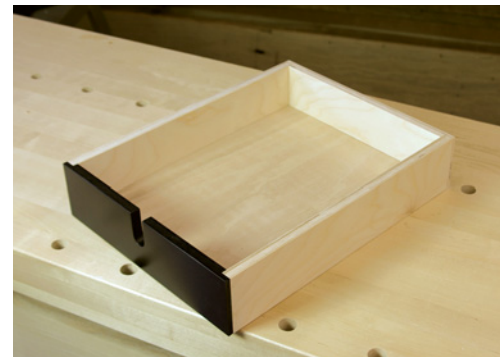
The drawers are the crowning detail. The simple rabbeted drawers are quick to make on the table saw. Taking advantage of a pneumatic pin nailer (firing a 23-gauge wire) I was able to paint the drawer fronts before assembling the drawers, providing a clean look.
