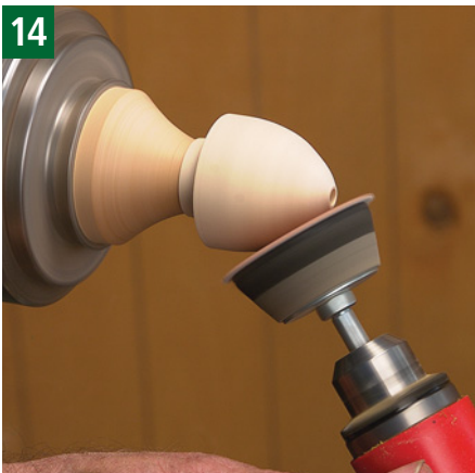
14 Sand the body with Velcro discs using #100, #150, #220, #320, and, if necessary, #400. Don't sand too much and get the walls too thin. Look through the entrance hole and the perch hole to check the wall thickness.
