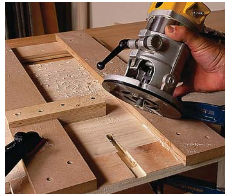
If you have two routers with the same base diameter, you can use one for the "wasting" cut with a straight bit (as shown at top), and the other with the dovetail bit (above left and right).
