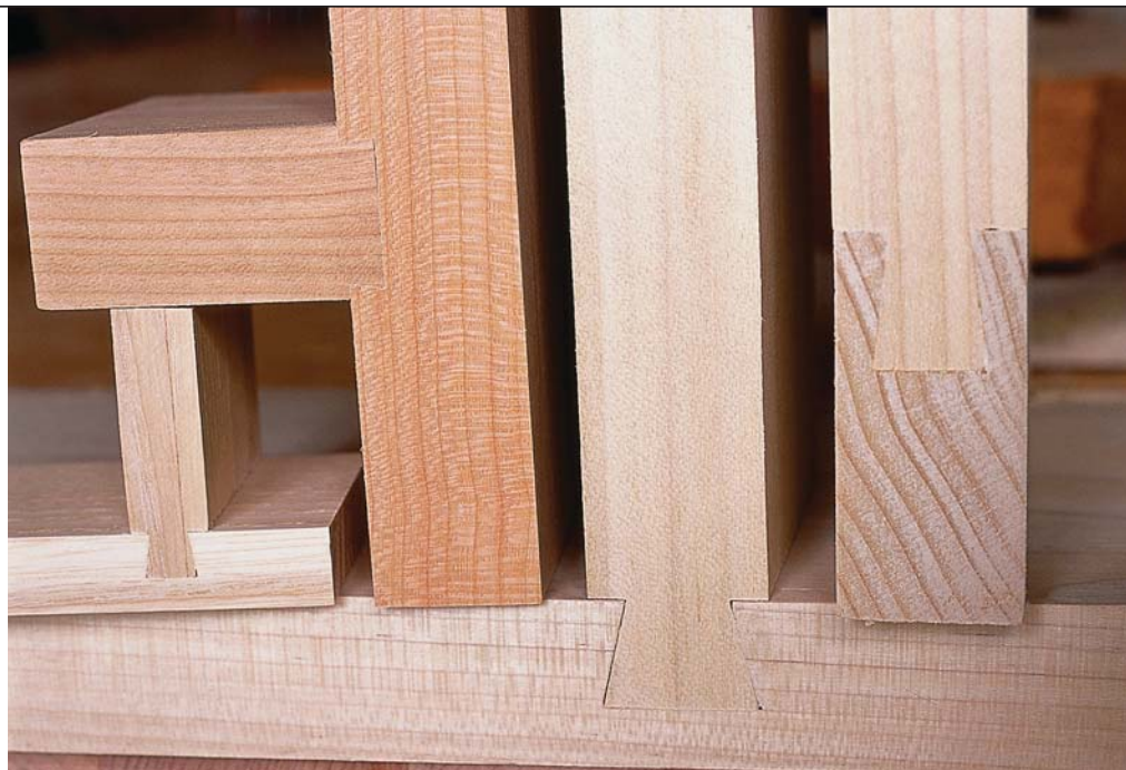
Router-cut sliding dovetails link parts together, with or without glue, and they have a multitude of uses.
