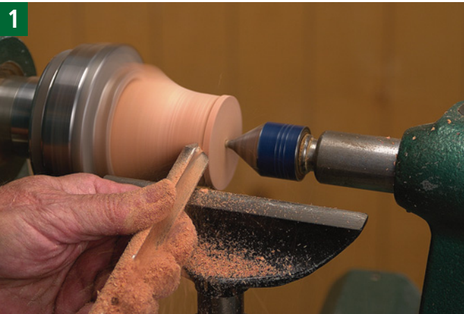
1 Select a block of wood approximately 2" square and about 2½" long. This can be put in a chuck or turned into a cylinder between centers with the grain running lengthwise.
