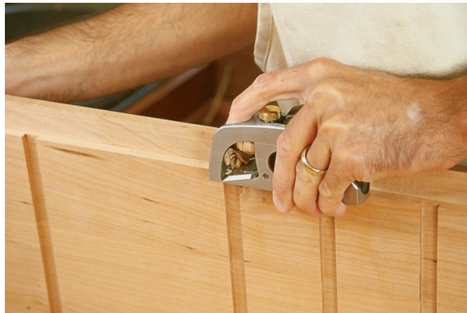
If your rabbets for the back are perfectly square, your case is much more likely to end up square, too. Clean up any imperfections with a rabbeting plane, such as this bullnose rabbet plane.
