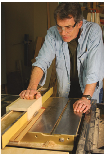
A push block that rides on the rip fence keeps your hands at a safe distance from the blade.
