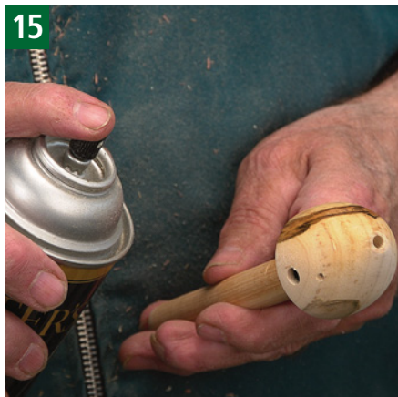
15 Finish the body. I prefer a lacquer finish. Insert a \frac{5}{8} " dowel 6" to 8" long into the body. This will make it easy to hold the body while spraying. I spray a full wet coat of Masters Magic high solids gloss lacquer. I prefer the gloss, as I want a shiny finish. After all, this is a Christmas ornament.
