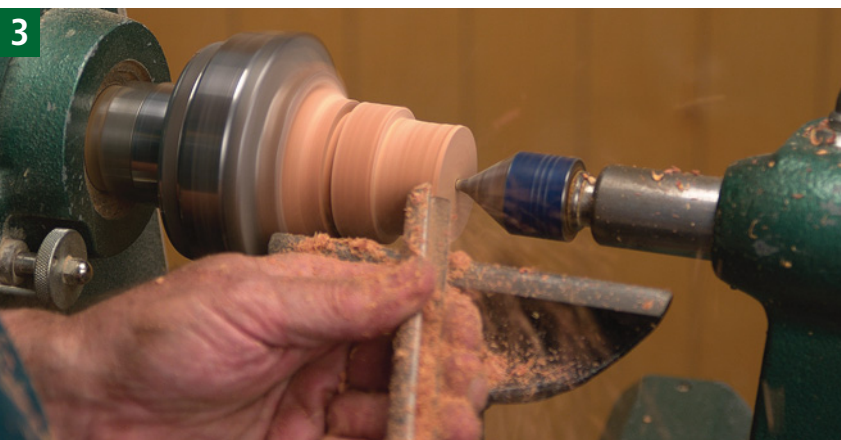
3 Turn the cylinder down to the calipered dimension using a gouge, removing stock up to two-thirds of the length, but not getting too close to the chuck. Cut the end of the cylinder clean and smooth.
