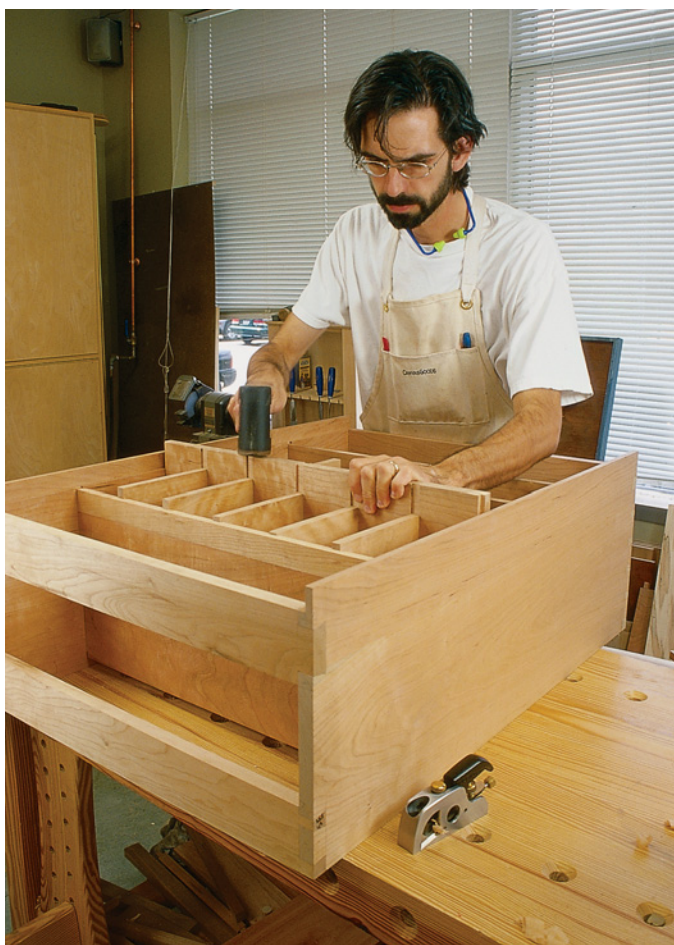
Fitting the dividers is easy with a hand plane. I merely make sure the dividers are surfaced a few thousandths of an inch thicker than where I want them to be. Then I thin them down with a smoothing plane until they slide in with just a little persuasion.
