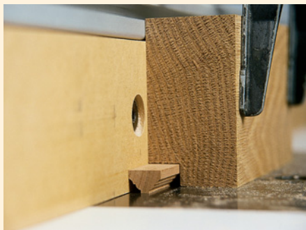
Because the piece is surrounded by the notched block, it can't twist or roll, even though very little wood remains on the table surface.
