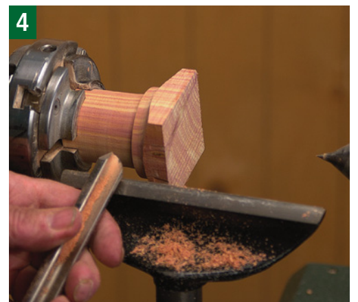
4 Reverse the stock in the chuck and turn off the square end. Turn the rest of the block to the correct rough dimension.
