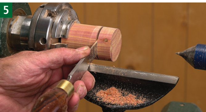
5 Measure and mark the cylinder to finished length. Part off the excess piece of wood. This should leave a cylinder 1¾" long. Examine the cylinder, checking for color or figure. The most interesting part of the work will be at the top of the body. It may be necessary to remove the cylinder from the chuck and reverse it to achieve this.
