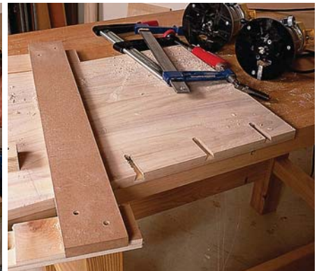
If you have two routers with the same base diameter, you can use one for the "wasting" cut with a straight bit (as shown at top), and the other with the dovetail bit (above left and right).
