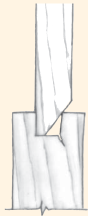
Bevel too steep Panel splits frame
