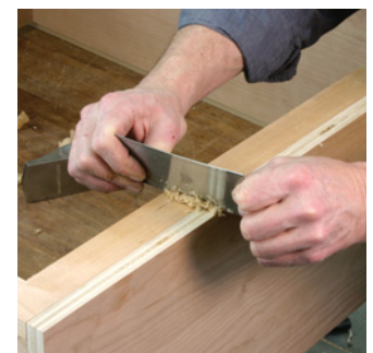
A card scraper brings the solid wood even with the plywood without raising a cloud of dust, or risking the damage that a belt sander or random-orbit sander could cause.
