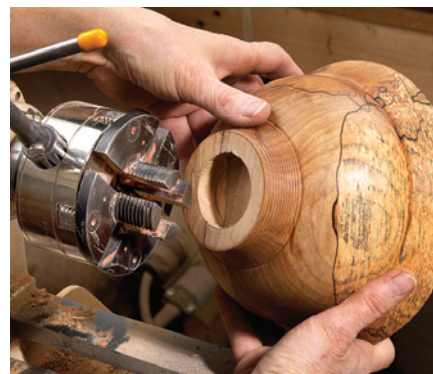
Mount the bowl on the chuck. Here the chuck jaws will expand in the cavity to hold the work.
