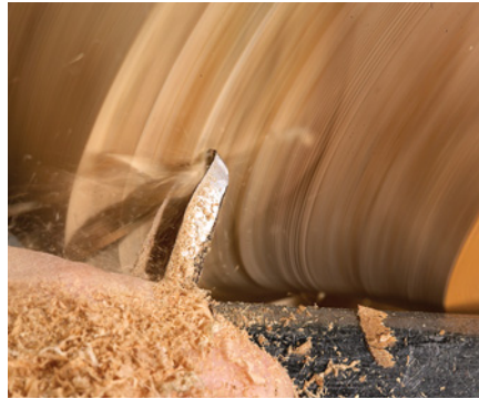
A higher-angle cut is good for removing a lot of material once the piece is round.
