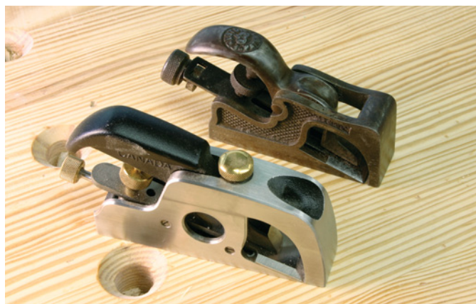
The Veritas bullnose plane shown with a vintage Preston version of the same tool. The Veritas plane has features and a shape that favors ergonomics and function over the classical form.
