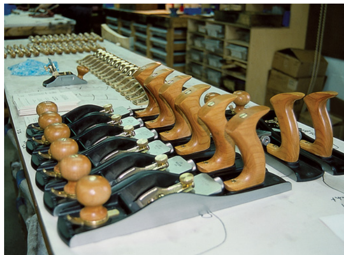
Lie-Nielsen low-angle jack planes being readied for shipment from the factory in Maine. Both companies hand-assemble each tool.
