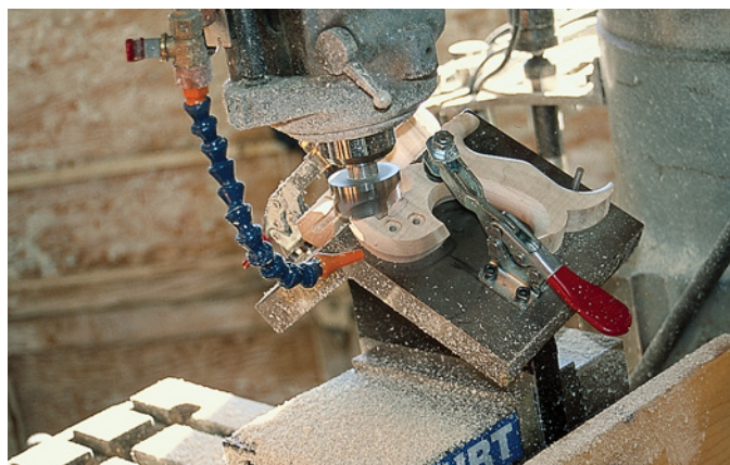
One of the big challenges for Lie-Nielsen and Lee Valley is to produce handles that are comfortable but that can be made with a minimum of hand work. Here a Lie-Nielsen saw handle is machined to shape.
