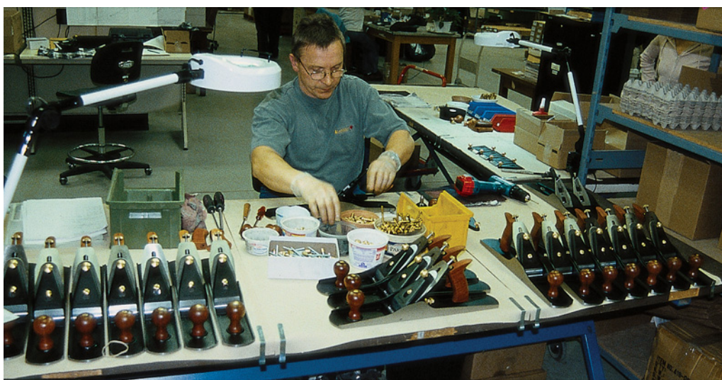
At Veritas, every tool has a checklist that must be followed at assembly-time. These checklists are continually fine-tuned for better results and faster work.
