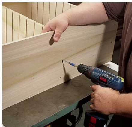
Some heavy-duty screws will ensure this cabinet will stay put, even when fully stocked.
