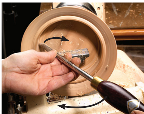
Note the position of the tool as I begin the cut. To keep the bevel rubbing while cutting the side of the bowl, the handle must be held far to the right and must swing around to the left as you cut to the bottom or center of the bowl.
