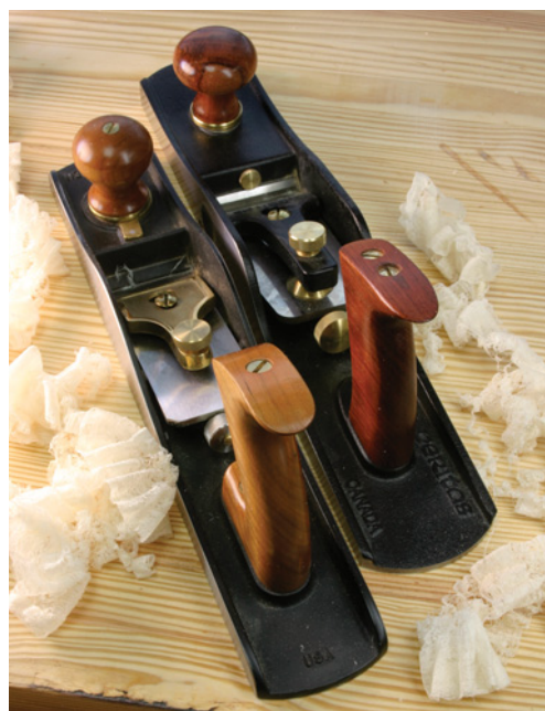
These two low-angle jack planes are quite different when you start comparing the details. They both work quite well, but different woodworkers will prefer one over the other.
