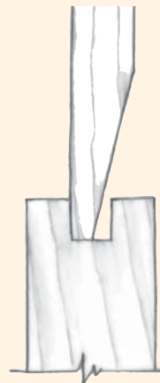
Bevel too shallow Panel loose in frame
