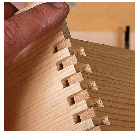
Cutting the full layout across both pieces isn't necessary to test the fit. If the setup is significantly off, fitting three or four pins will expose it. If those pins mesh nicely, cut more of them and refit the joint.
