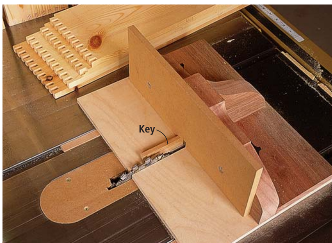
The jig I use on the table saw rides in both miter-gauge slots. The adjustable facing, into which the key is glued, is cut from a scrap of 1/2" MDF.
