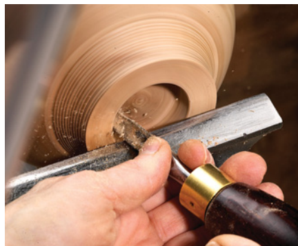
Cut a recess in the foot for remounting the workpiece on the chuck.
