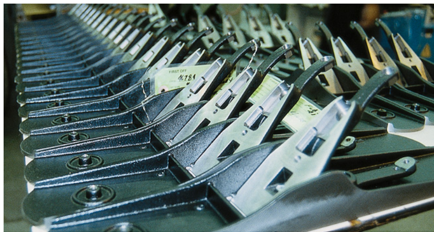
Veritas No. 6 fore planes after the frogs have been machined. Unlike a traditional No. 6, the Veritas has its mouth located further back than the Stanley versions.
