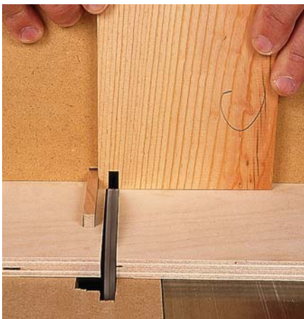
Stand the work on end, tight against the key. Push the jig across the cutter and make the first slot.
