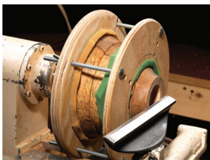
Here you can see the nearly completed bowl mounted in the doughnut jig.
