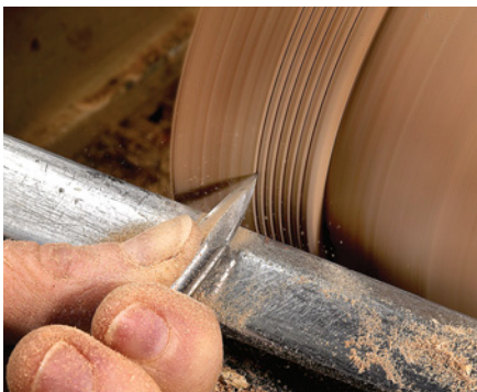
The fingernail-grind spindle gouge is perfect for detail work on the outside, foot and rim.
