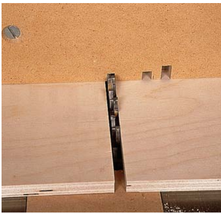
Kerfing the adjustable fence for the key is the first step in setting up your box-joint jig. Note the two kerfs from a previous job to the right of the blade. It's best, I think, to set up fresh for each new job.
