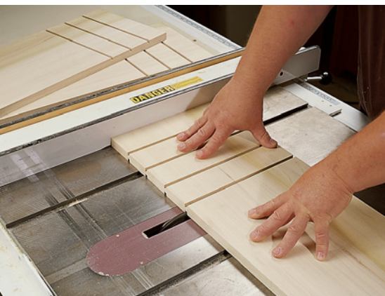
Cutting the dados is simple work with a dado set installed in your table saw. Cut four dados (one on each side piece and two on the divider), move the fence, then cut four more and so on.
