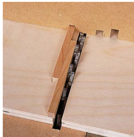
Make a key strip, hand-planing it to achieve a tight press-fit in the kerf. Cut the strip into two pieces: one is the key, the second is a setup gauge.
