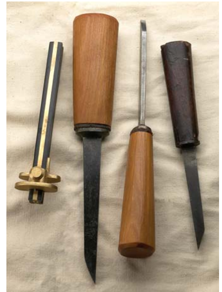
Here you can see cabinetmaker's or joiner's mortise chisels.
