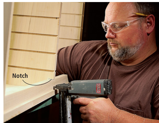
Two screw strips, one on the top and one on the bottom, allow you to screw your cabinet to your shop wall. Notice the notch cut into the divider to allow the screw strip to fit.
