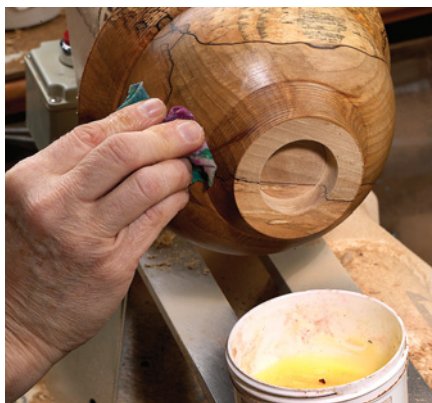
Apply finish to the completed exterior.
