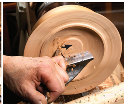
Note the position of the tool as I begin the cut. To keep the bevel rubbing while cutting the side of the bowl, the handle must be held far to the right and must swing around to the left as you cut to the bottom or center of the bowl.
