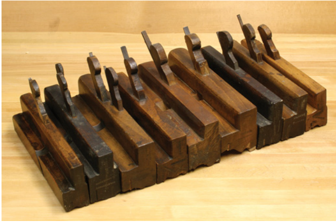
Complex moulders produce shapes with complex curves or multiple features; simple moulders produce a single, fillet-less, convex or concave arc.
