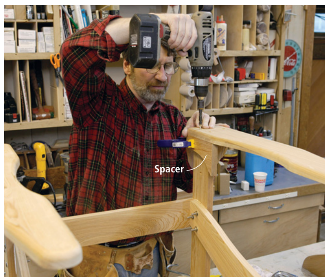
Use three screws to attach the arm to the leg and arm bracket. Carefully position the arm for a \frac{3}{4} " overhang of the leg. Use a spacer to help position it. The arm overhangs the front edge of the leg 1\frac{1}{8} ".
