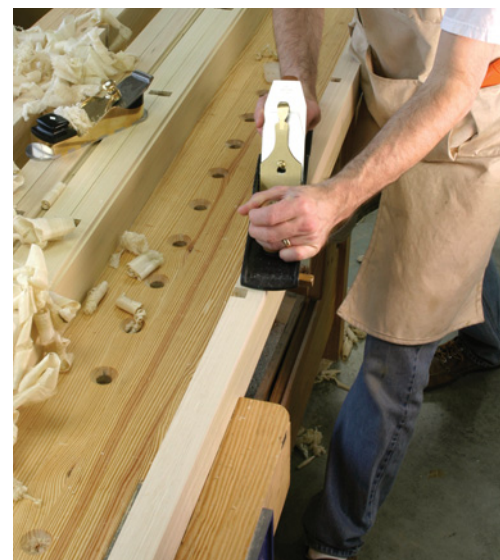
I used poplar for my uprights, which is easy to plane. After removing any bow with my jointer plane, a pass or two with a smoothing plane is all this forgiving wood needs to be ready to finish.
