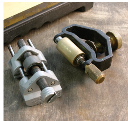
The Eclipse-type side-clamp honing guide (left) has a narrow roller that allows you to more readily rock the guide when forming a curved edge.
