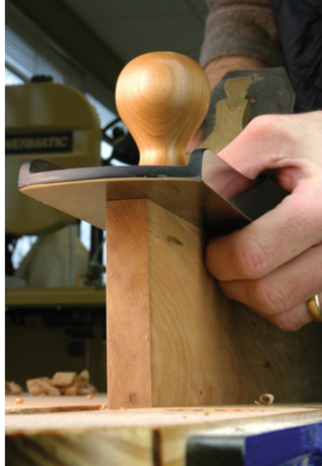
Use your fingernails as a fence to help maintain the plane body square to the edge of the board.
