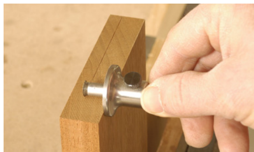
Using a marking gauge, scribe a line across the end grain of the drawer front. It should be about one-third of the board's thickness in from the face.
