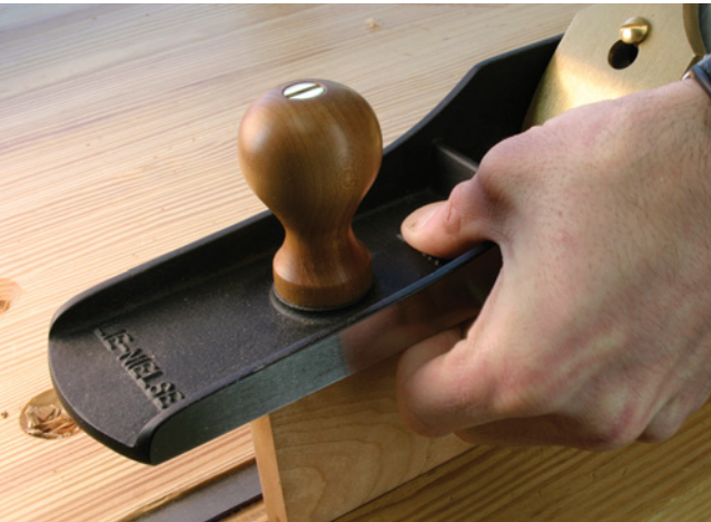
To accurately plane a board's edge, position your thumb and fingers as shown.
