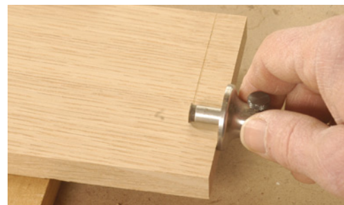
Without changing the setting on the gauge, scribe a line on both inside and outside faces of the drawer sides. These are the base lines for cutting the tails.
