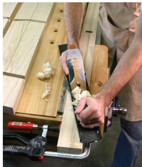
With the angle cut, clamp two mating uprights together and plane down to your line. The longer the plane the straighter your surface will be.
