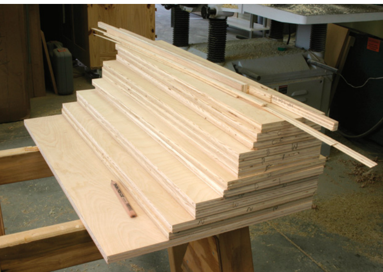
Take care when cutting your plywood because every kerf counts. Shown is my stack of finished shelves. That little pile on top of the shelves is the waste that was left from an entire sheet of plywood.
