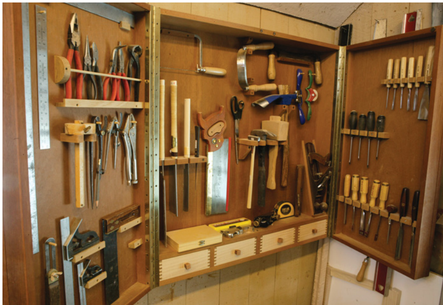
Norm Abram's shop does have a decent collection of hand tools. Abram "hides" his chisels in this wall-mounted tool chest, which was a project on the show. Lately, he's become fond of Japanese hand saws. Also note his measuring and marking tools. Abram says these are the most important tools he owns.
