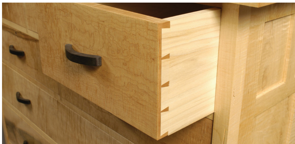
Half-blind dovetails cut using this method look exactly like those cut entirely by hand.
