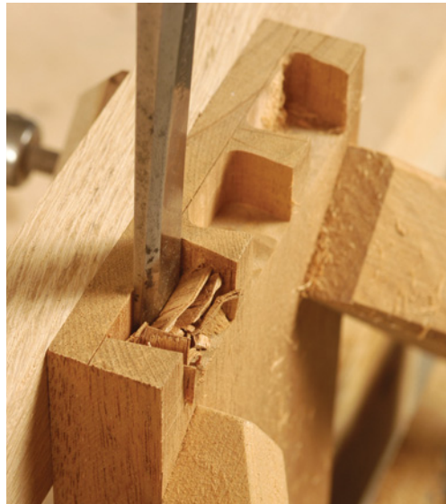
When the sides of the pins have been pared to the line, work on the front of the joint. Make sure the front edge and the sides of the pins are square, not sloped, so the joint will go together without splinting the drawer front.
