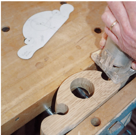
Round the edges with a trim router. The template for the layout of the body is on the bench.
