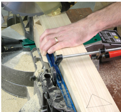
Cutting 85"-long pieces all to the same size is impossible on most table saws. So I gang-cut the pieces on my miter saw. Clamp your mating uprights together and cross-cut them simultaneously. This way if they're a little off, they'll still match.
