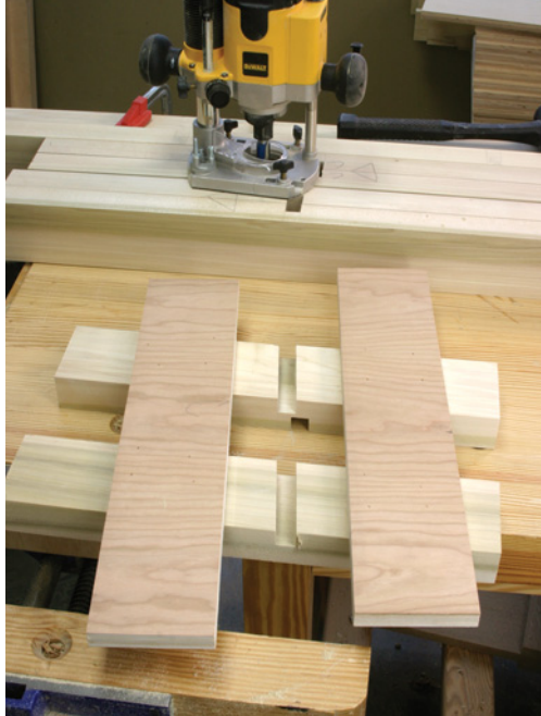
To build a dado jig, draw a 7° angle on your scrap and then build the jig around that line and your router's baseplate using scraps, glue and nails.
