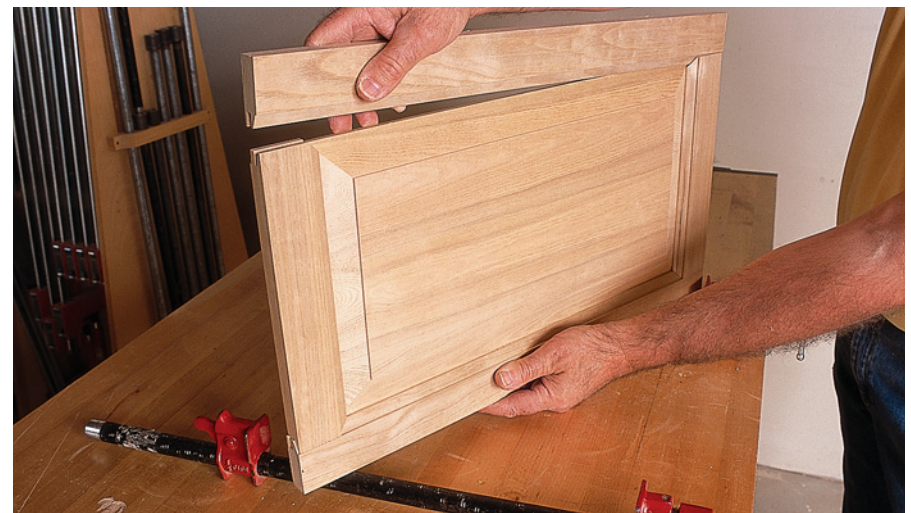
Cope-and-stick joinery is an efficient method for assembling doors and other panels.
