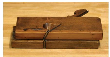
A skew rabbet plane (top) can work across the grain or with it. The square rabbet plane (bottom) is easier to freehand.
