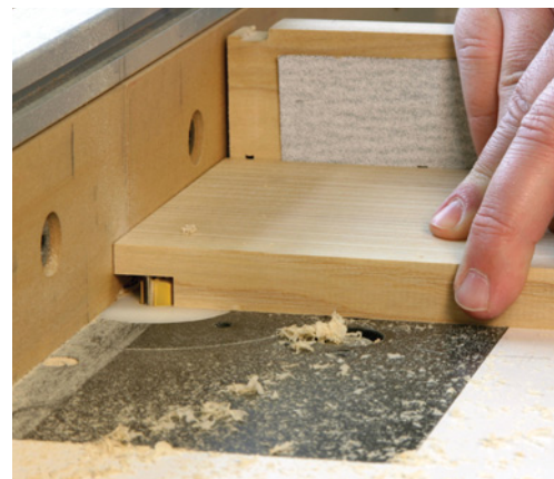
The second and final pass is made to complete the rabbet. Repeat both steps on each mating piece. Note the sandpaper on the miter gauge fence to keep the piece from moving during the cuts.
