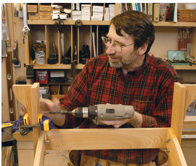
Position and clamp the arm bracket then drill and countersink for two screws. The top edge of the support should be flush with the top of the leg and centered in the width dimension of the leg.
