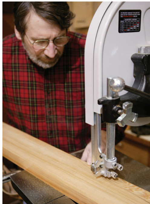
Cut both chair side pieces at the same time by nailing them together in a waste section of wood. Band saw to the template line then sand the edges smooth.
