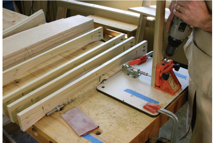
This project is where pocket screws really shine. Whenever you’re working at an odd angle or near edges like this, a pocket screw can be your best bet. The other reason I chose them is because I wanted to finish the parts separately and assemble the project on-site.
