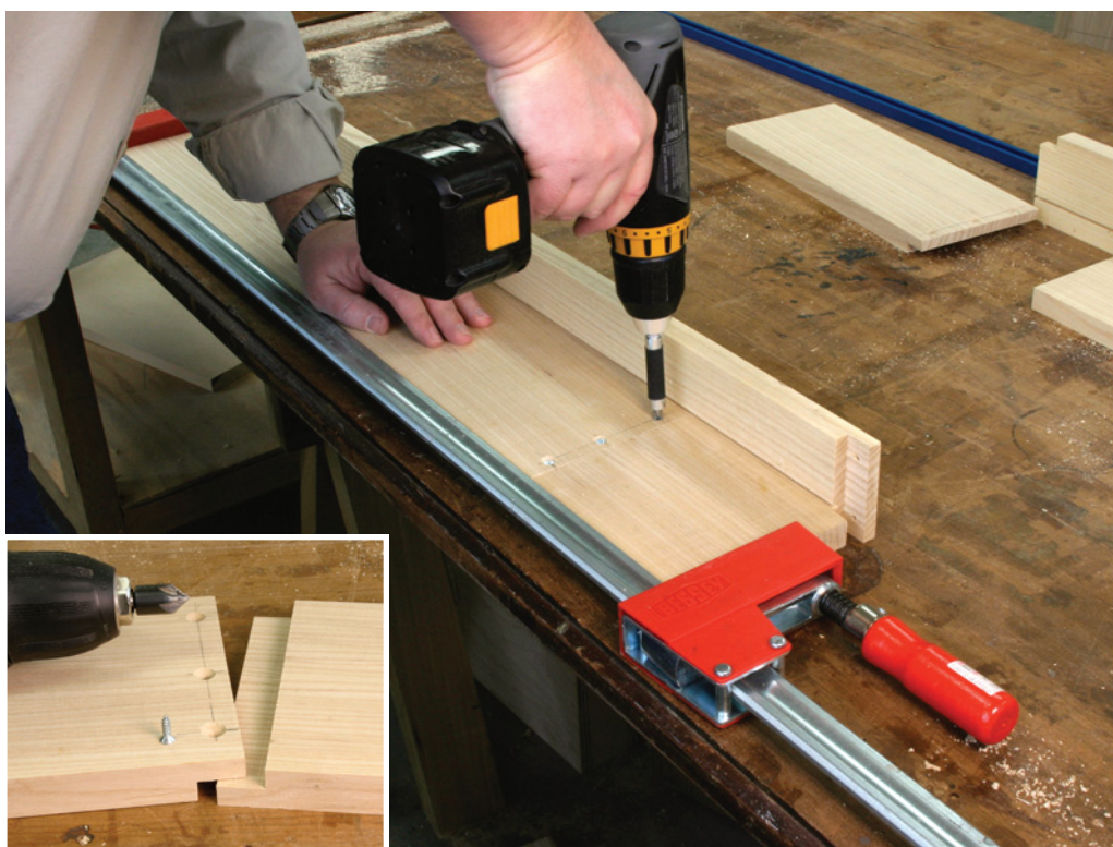
Accurately screwing the mating half-lap pieces together requires clamping the pieces together. Countersunk pilot holes and flathead screws complete the assembly.
