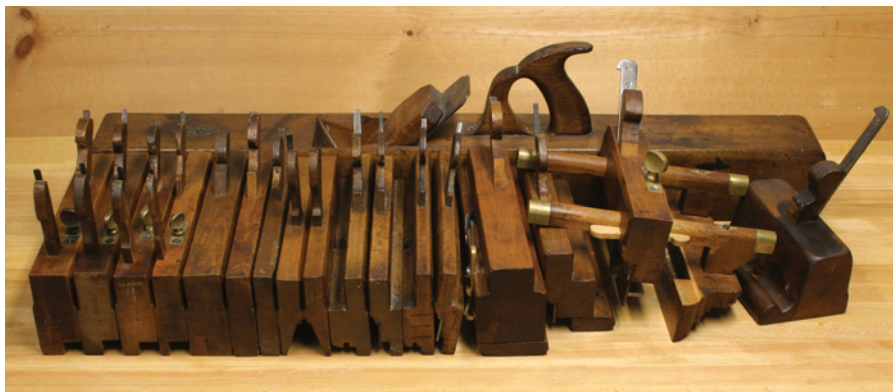
Shown from left are a set of four dado planes, three skew rabbets, a pair of side rabbets, two pairs of match planes for different size stock, moving fillester, specialty drawer bottom plow, wedged arm plow, old widow's tooth router (uses plow plane irons) and a 30" jointer plane behind them all.
