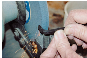
Grind the cutter to a 30^\circ angle. Grinding manufacturers don't recommend side grinding but I've always felt safe.
