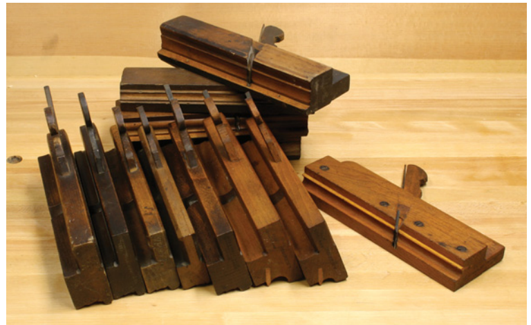
Technically, beads and sash planes (as shown here) are complex moulding planes, but they are rarely categorized as such.
