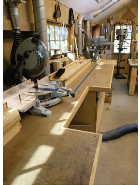
This massive miter saw stand and storage center was a project on the show. Directly underneath the miter saw is a roll-around scrap bin.
