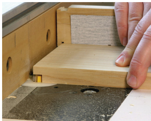
A simple 3/4"-wide rabbet is the secret to the mating half-lap joints. After determining the exact center of the board thickness, a 1/2" straight bit is set to cut to that height. The fence is set for the final width of the rabbet, but the first pass is made at the edge of the board.
