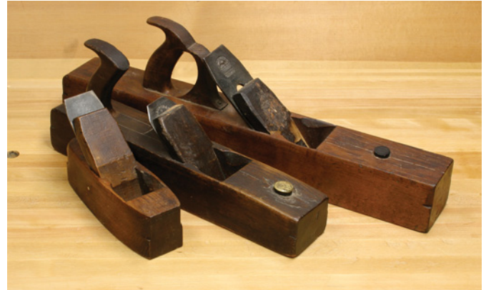
The degree of blade curvature varies: smoothers (left) have the least, fore planes (center) the most. As a side benefit, the curved blades eliminate the necessity for lateral-adjustment mechanisms. At right is a try plane.
