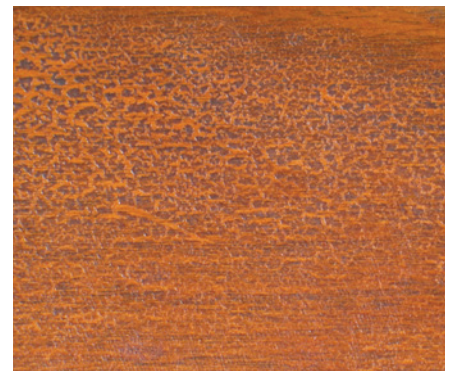
Finishes that have softened and become wrinkled (and also dirty) because of extended contact with acids contained in body oils and sweat (as shown above) usually have to be stripped and replaced with a new finish.
