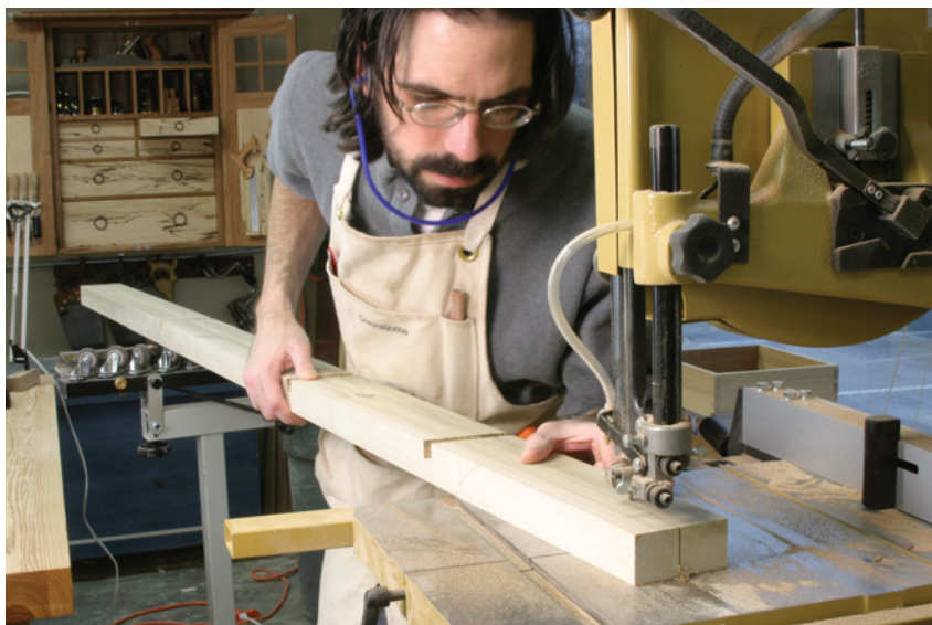
I'm sure that some of you will figure out a way to do this on the table saw, but the band saw is far quicker for me. A roller stand holds the bottom end up while I make the cut at the top end.
