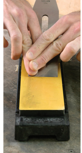
To smooth out the curved edge, remove the plastic from the stone and hone using finger-point pressure at five stations on the iron.
