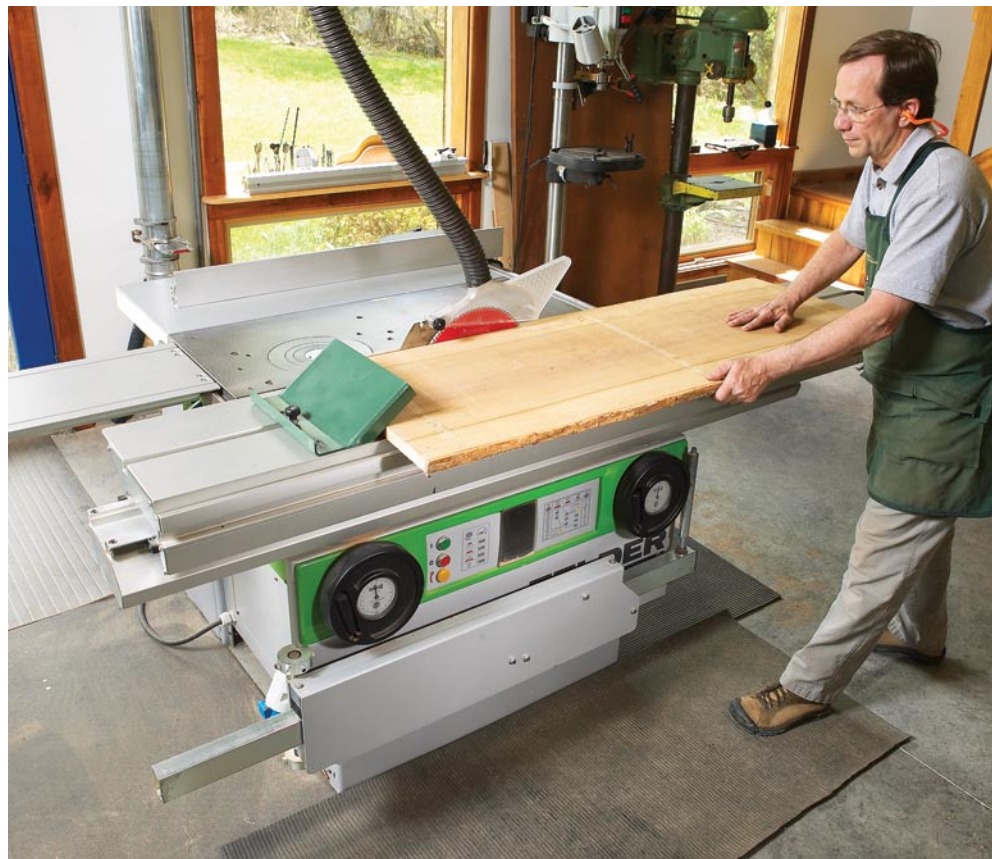
Difficult cuts made easy. Ripping the wane off a board or ripping a board with a crook can be a challenge. But with the European-style shoe attached to your sliding table, you can rip difficult woods with little effort or risk.
