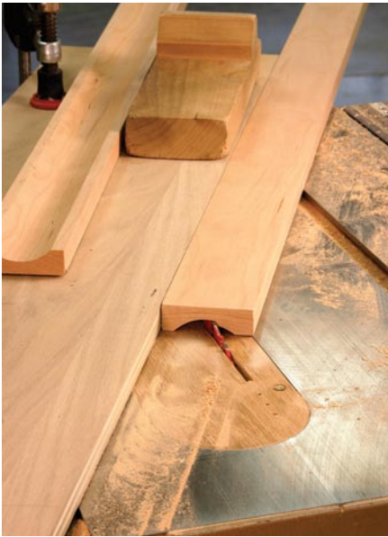
Sculpt the mouldings. Incremental steps in blade height are used when cutting the cove. Then cut the 45° bevels on the long edges.
