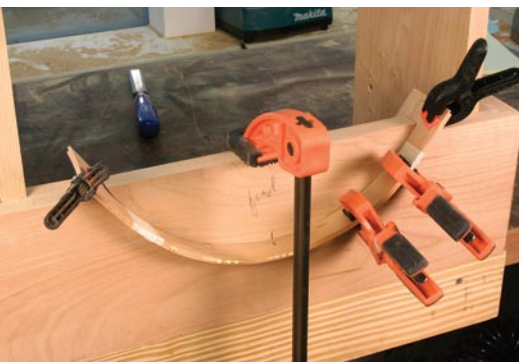
Two strips make one bead. The offcut from the gallery front is an excellent caul for clamping the laminated bead into the profile. Small spring clamps close any gaps between the pieces.
