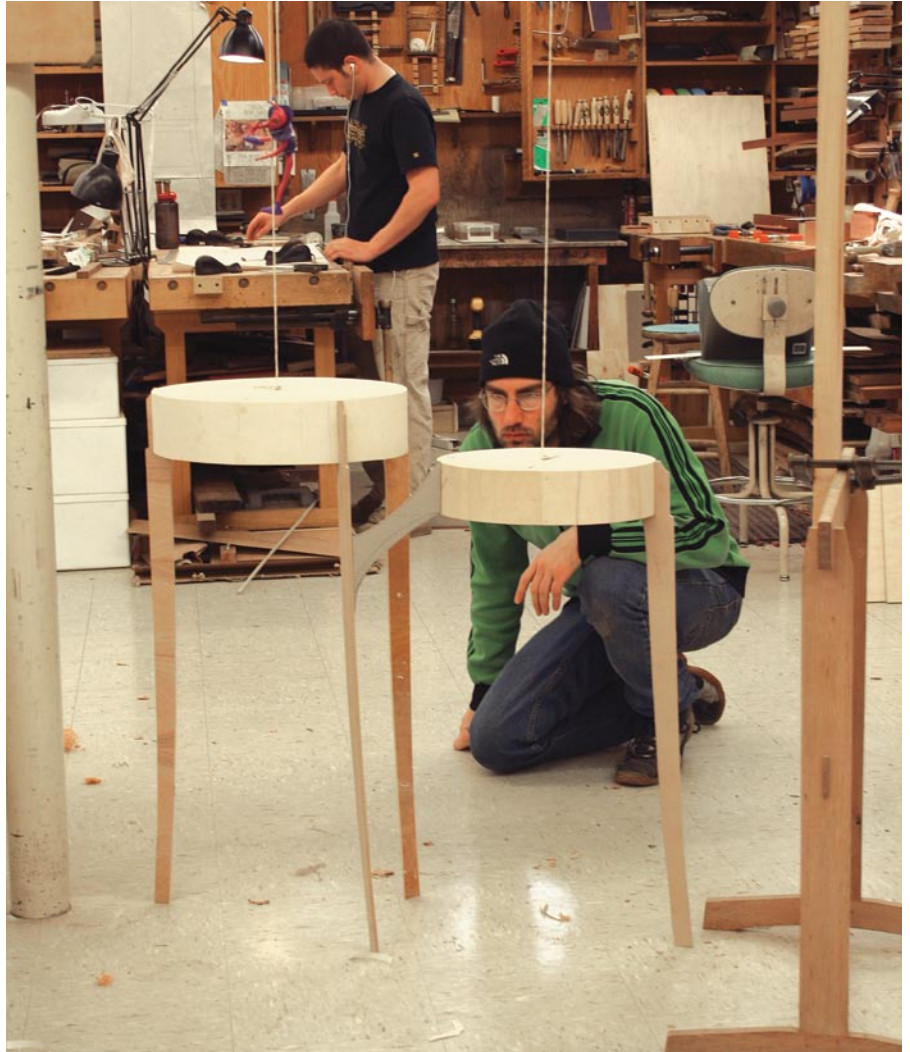
Design in three dimensions. The process of creating new designs follows that employed by James Krenov; full-size mockups like this one by Germán Plessi of Buenos Aires, Argentina, supplement drawings to better visualize details from all angles.
