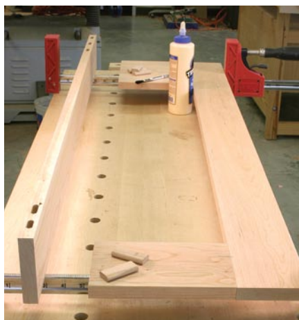
Loose-tenon construction. Cutting the mortises with the Domino is quick work. Select the best face for the waist frame of the clock.
