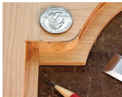
Ease the fit of the glass. Leaving this sharp corner square makes fitting the glass nearly impossible. Breakage is imminent. Rounding the area to the radius of a quarter keeps you from working with more than one piece of glass.
