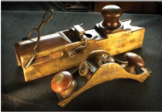
Not in any tool catalog. Some of the unusual planes that Sindelar acquired through a middleman. Little is known for sure about the planes, except that they look like nothing else. The bench planes (above) include a plane with a hefty fence integrated into its design. The other grouping (left) shows a fixed-sole compass plane and an unusual plane that was designed to plane boards to one specific thickness.
