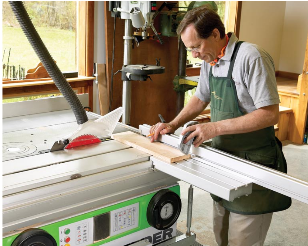
Crosscutting. European saws have an array of fences for the sliding tables in different lengths. These can be used for mitering, crosscutting and compound cutting.
