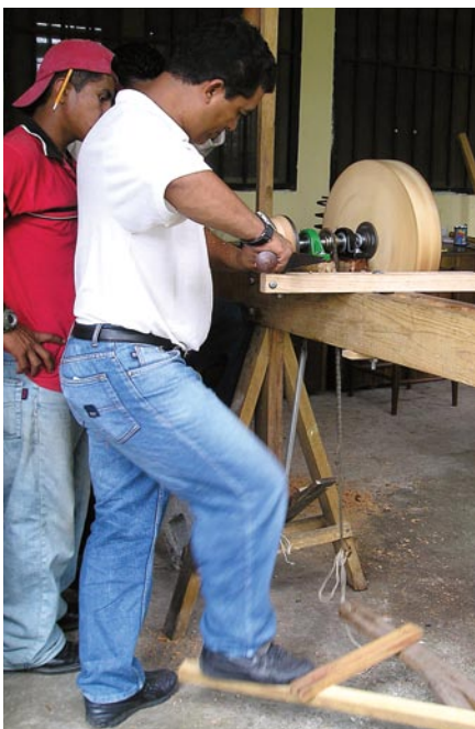
Trial run. One of the Honduran artisans takes the new lathe for a spin.
