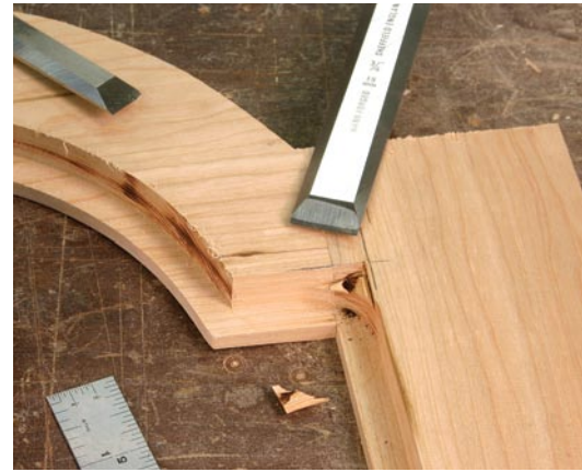
Prep the door for glass. The inside corners are left rounded by the rabbeting bit and need to be squared with chisels. Cut the end grain using the force provided from a mallet while cutting the side grain with only hand pressure. Too much force can crack the face of the door.
