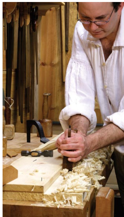
Two dados at once. To keep everything lined up, I prefer to dado both sides at once. The fronts are placed together so the plane exits at the back of the piece. A nailed-on piece of scrap wood serves as a fence.
