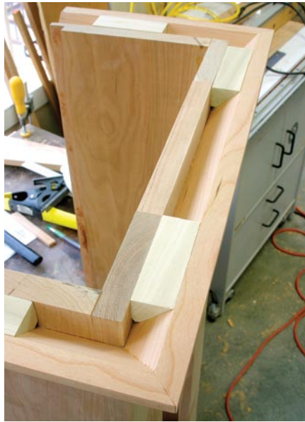
Fitted blocks support the hood. Scrap pieces cut with a 45° bevel, when glued in place, add support for the cove moulding and carry some of the load from the hood.
