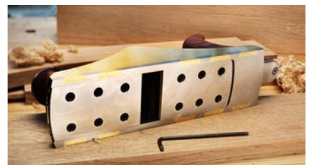
Sole of a new machine. The VP-60 has two sole plates to close up the mouth for any planing situation.
