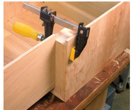
Make a level connection. Attaching the waist properly to the base is important to the standing of the clock. If the waist isn't square to the base the clock will lean back or pitch forward. Bring the waist level before adding the screws.
