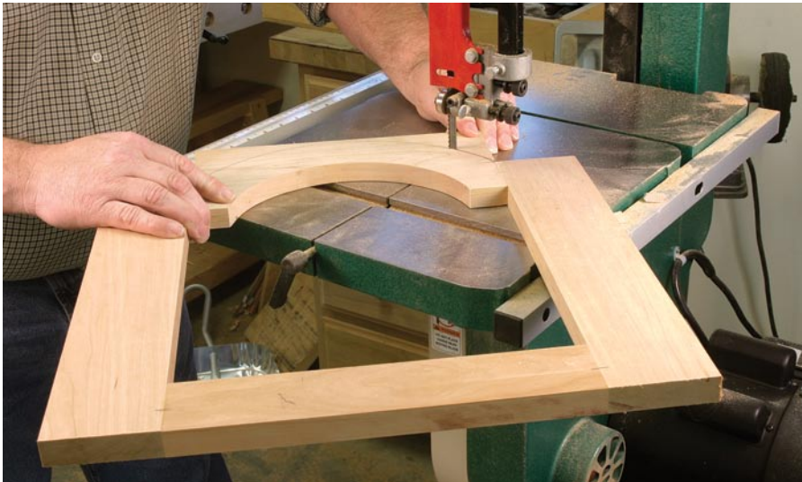
Fit the hood door. Once the outer arch is cut, the door is fit to the hood. Fit the door in position then fine-tune the fit to create an even reveal around the door.
