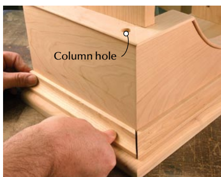
Small cove finishes the hood mouldings. This moulding is created at the router table with a 1/2" cove bit. The bit is slightly raised with each pass, creating the irregular profile.
