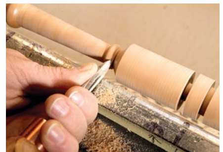
9 Finish cleaning up the taper, and turn the bead. As the narrowest part gets smaller, vibrations will increase. Take lighter cuts; push into the cut, not toward the workpiece.
