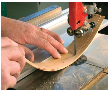
Handwork finishes the bent bead. Trim the bead to width at the band saw, but the majority of the work of matching to the flat bead is completed with chisels. Carefully angle the ends of the bead to fit those of the matching corner pieces.
