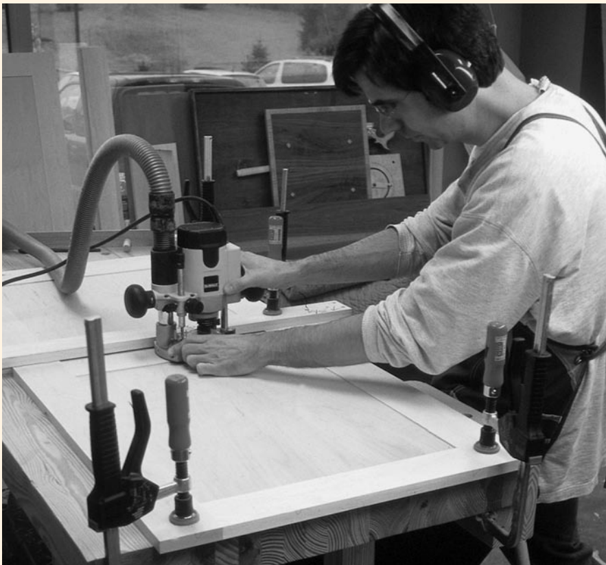
A router with a dust-collection port will keep shop air much cleaner. And without all those chips flying around, it's a lot easier to see what you're doing.
