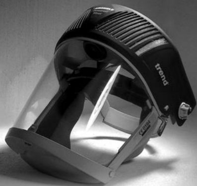
This Trend Airshield provides a steady flow of filtered air from a battery-powered motor that runs four hours between charges. Turners find this type of respirator especially useful because it combines a full-face shield with respiratory protection.
