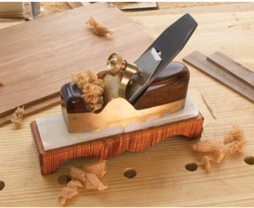
Slick storage. This plane wick is an excellent place to set your tool when it's not in use.
