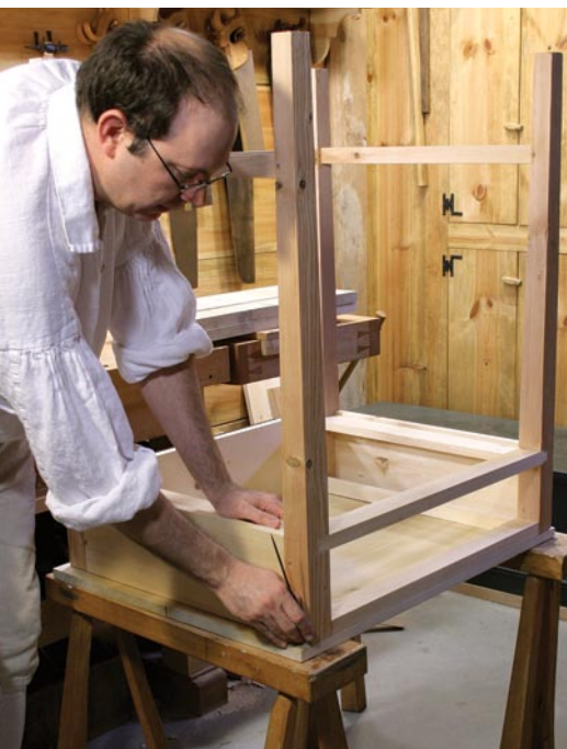
Matching sizes. I sawed the boards to shape, starting by matching the bottom board to the lower case. This allowed for a slightly irregular lower case (this lower case was surprisingly square, doubtless due in part to the match-planing of the legs). The sides and top were then matched to this board and to each other as required.
