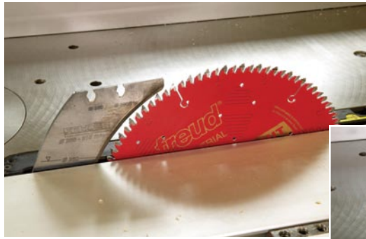
Follow the action. The riving knife behind the blade moves up and down with the blade. The knife prevents kickbacks and doesn't have to be removed for typical operations, such as cutting joints.
