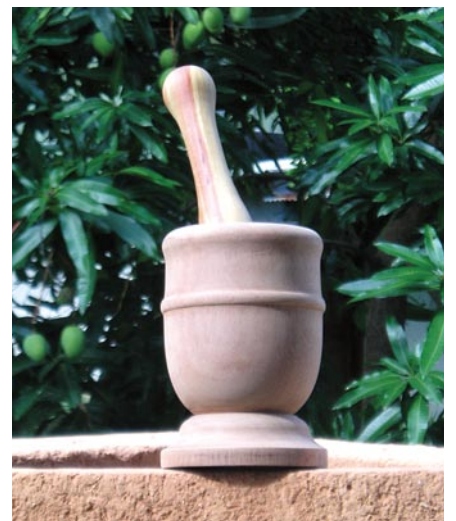
Results. A finished mortar and pestle, turned on a bicycle lathe in La Cieba, Honduras.
