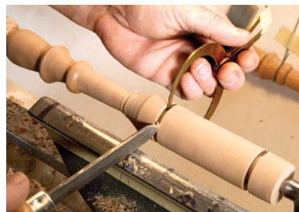
8 With the parting tool, cut to the diameter of the bead on the long taper. The parting cut on the right end of the handle is where the end of the handle will be.
