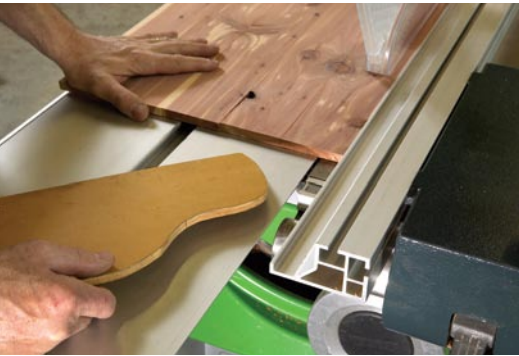
The advantage of a low fence. When ripping narrow stock, the low fence gives you lots of room to work safely.
