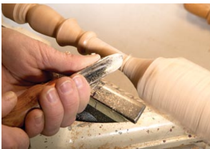
7 Clean up the taper, turning downhill (large to small diameter). Stop cutting just before you get to the waste remaining on the right; if you push the gouge uphill, it will catch badly.
