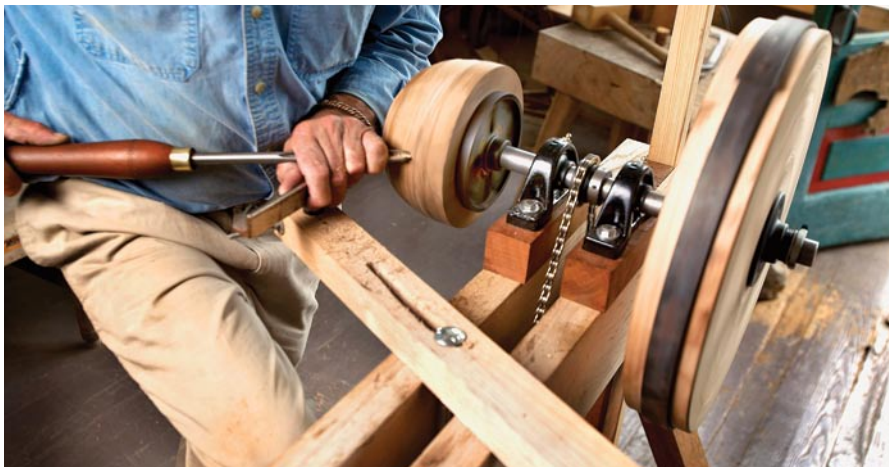
Power enough. And that gives me enough rpm to turn end grain on this bowl.
