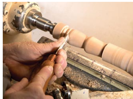
5 Round the end of the handle, but don't cut too far in yet. You'll need the support on this end when you rough in the other half of the handle.
