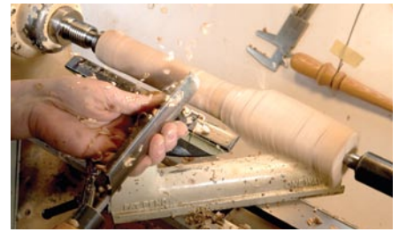
2 Begin by rounding off the workpiece. A large roughing (spindle) gouge is quick and effective. Cut on the low side of the gouge, and from larger to smaller diameter.
