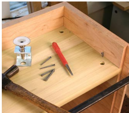
Plumb is peachy. The levelers hold the clock plumb when it sits on a non-level floor. Adjusting the levelers through the bottom requires drilling access holes in the bottom of the base.
