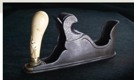
The scraping snake. An unusual European ivory-handled plane. The plane shows signs of use (lots of hammer taps on the wedge), and its construction suggests it is a scraping plane.
