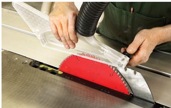
Quick-change artist. By twisting a knob and pulling upward, you can remove the blade cover in just a few seconds. Most U.S. saws have no such feature.
