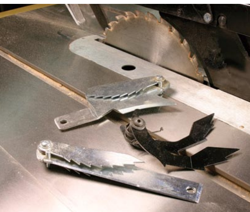
Anti-kickback pawls. These toothed, spring-loaded devices are supposed to stop work from flying back at the operator. However, most woodworkers remove them.
