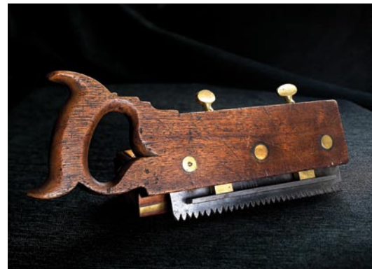
The ultimate stairsaw. An English stairsaw, used for cutting dados in stringers. Note the ingenious depth stop by the blade.
