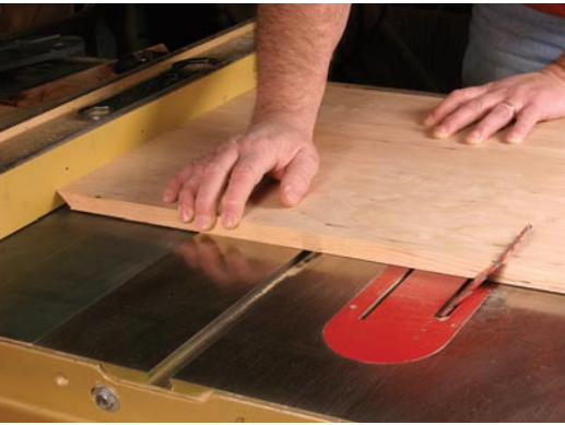
Last cut for the front panel. The left-tilt table saw is great for cutting the 45° miters for the base pieces. At a right-tilt saw, use a panel-cutting jig or sliding table attachment.
