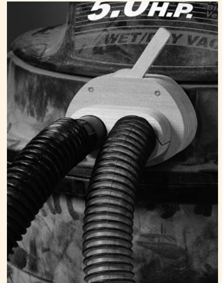
This shop-made blast gate for a shop vacuum allows two tools to be connected at the same time. A simple toggle switch opens one inlet port at a time.
