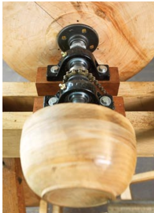
User's perspective. The chain runs around this bicycle-gear sprocket spinning it (the flywheel behind helps keep the momentum up) ...
