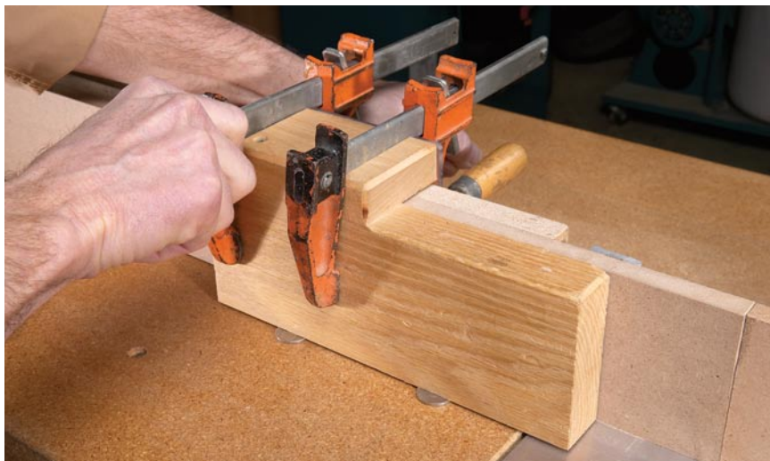
Clamp it twice. A loose stop block will spoil your accuracy and cause you to lose control of your cut. Whenever possible, use two clamps on your stop blocks, such as this stop on my miter saw's fence.
