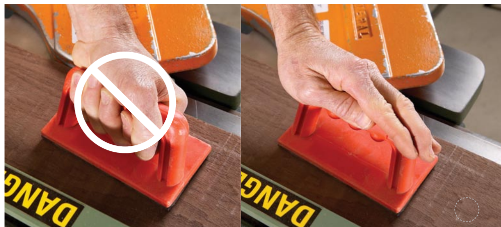
Wrong and right. The push blocks that came with your jointer are useful if you use them correctly. Don't grasp the handle as shown above left. This traps your hands. Instead, wrap your hand over the push block as shown at right. Don't forget to replace the pad's foam with a piece of sandpaper.
