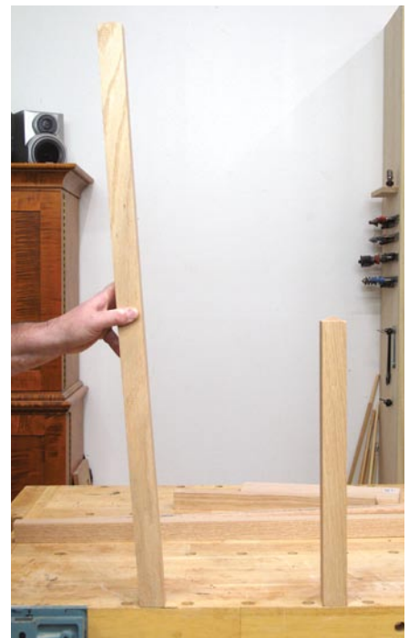
Angle adds comfort. The rear leg (left) needs only a slight (5°) angle cut on the bottom to add about 50 percent more comfort to your chair.
