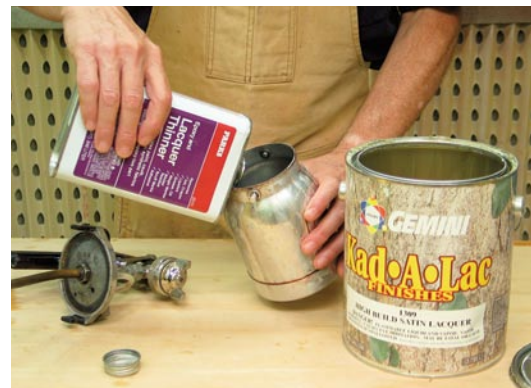
Thinning lacquer. Lacquer thinner is a blend of half-a-dozen or so solvents specially formulated for thinning lacquer. The blend allows for differing evaporation rates and for evaporation in steps to reduce runs on vertical surfaces.
