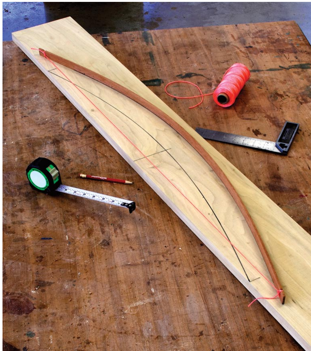
The important part. When drawing an arc, where it stops and starts, and the high point in between are more important than knowing the exact radius. Connect those points and you're ready to go.
