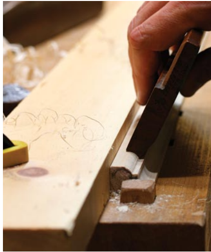
Hollow plane. I've flipped the moulding again and now I'm working the astragal portion with a hollow plane. I'll do one side at a time then finish the top surface.
