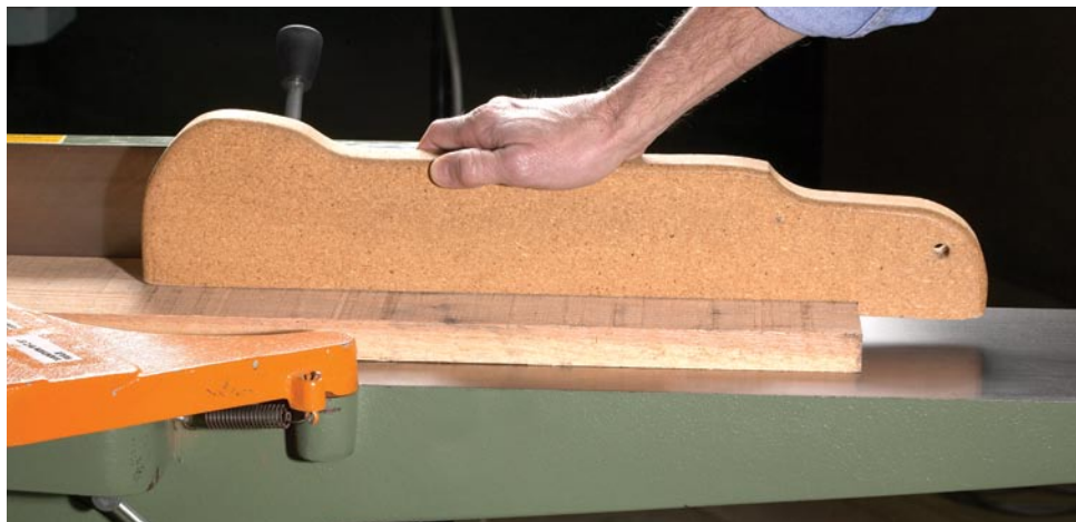
Hooks and protects. The hook at the end of this push stick protects your thumbs from a common injury on the jointer; plus, it changes the vector of the forces applied to the board to give you more control during the cut.
