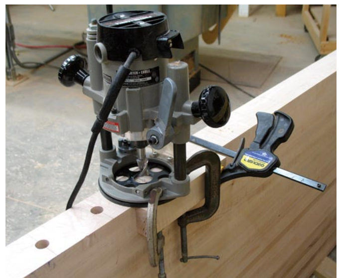
Hold-down holes. A second rigging is needed to drill the holes in the top's front edge. These holes are for accessories that hold wide panels in place.
