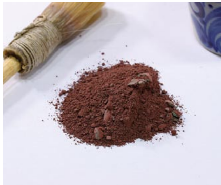
Just add water. Milk paint is available commercially as a powder. Just add water until it is the consistency of milk. Here I've mixed two parts of barn red with one part of Lexington green. The result will be a dark red. I mix single coats or less at a time, and don't measure my recipes too accurately. I'm looking for a little movement in the color.
