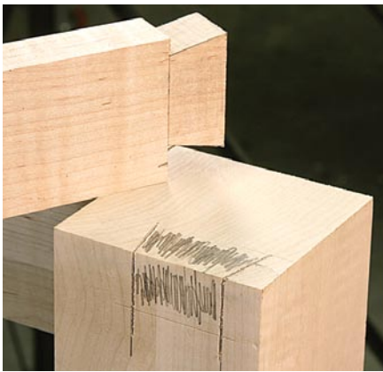
A furniture joint on the bench. Shaker craftsmen would employ the dovetail joint for the top rail. To maintain strength in the joint, set the socket back from the front edge.
