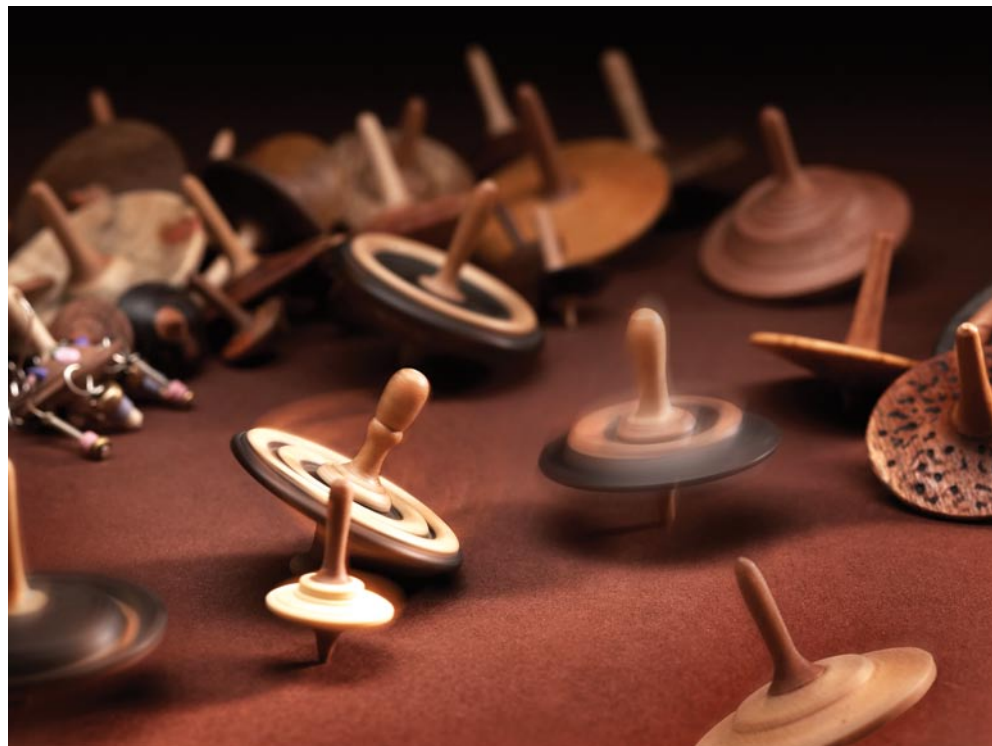
Spinning tops. There are a vast number of decorative and material possibilities when turning finger tops. Exotic woods, bone, antler, plastics and even countertop composites can be turned into these fun little gifts. To add an extra decorative touch, consider gluing up contrasting woods for blanks, adding beads around the edges, or burning a design the wood.
