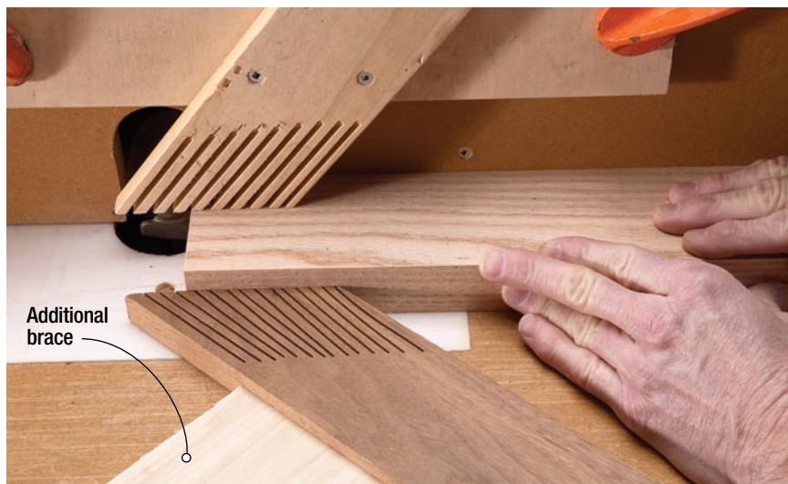
Helpful featherboards. Here I'm employing two featherboards to keep the work under control. Note the additional brace in front of the featherboard that's flat on the router table.
