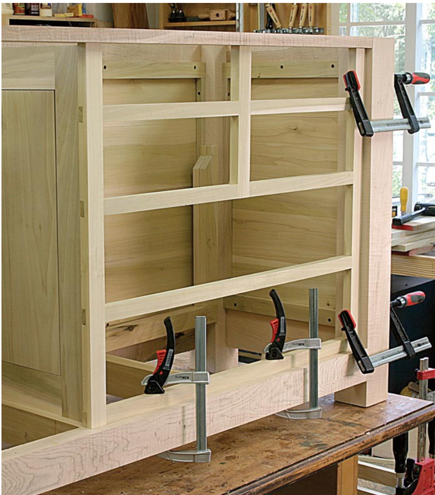
Well-placed clamps. Clamping the face frame to the bench base does not require scads of clamps. Strategic placement and having a square frame guarantee an accurate glue-up.
