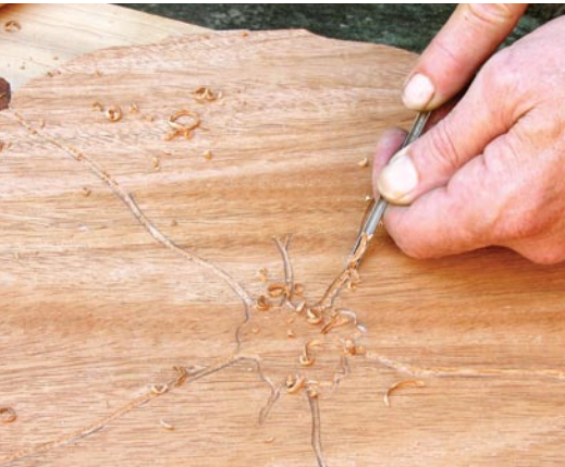
Shape from the tool. After starting the carving with a V-tool, a deep, narrow gouge cleans up the cuts and defines the profile of the lines.
