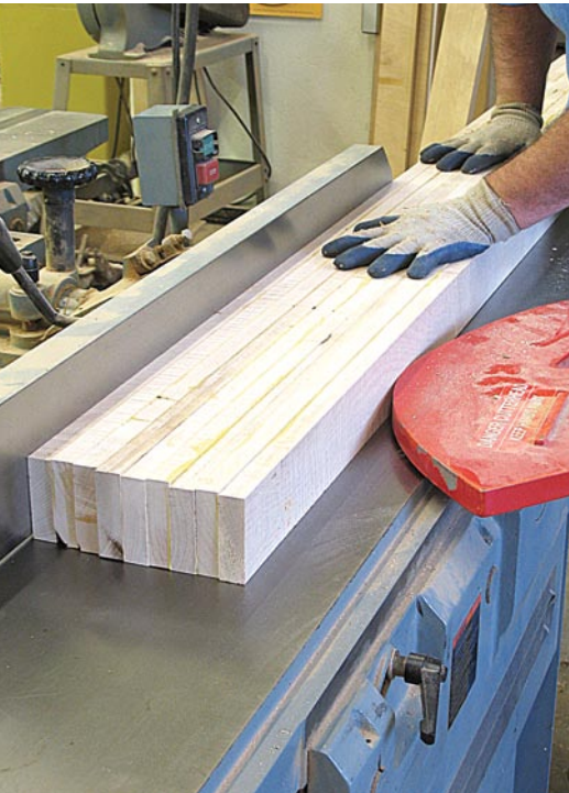
Jointing a flat surface. The stock for the top begins oversized to allow multiple trips to the jointer and planer. Having a level and true workbench top is paramount in bench making.
