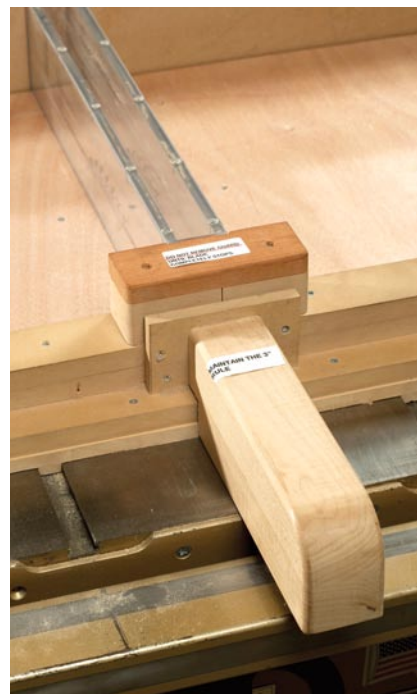
Two more layers of protection. The clear Lexan shield on this cut-off sled is durable and does not restrict your line of sight. The block of wood at the end of the shield covers the blade at the end of the cut, making this jig quite safe.
