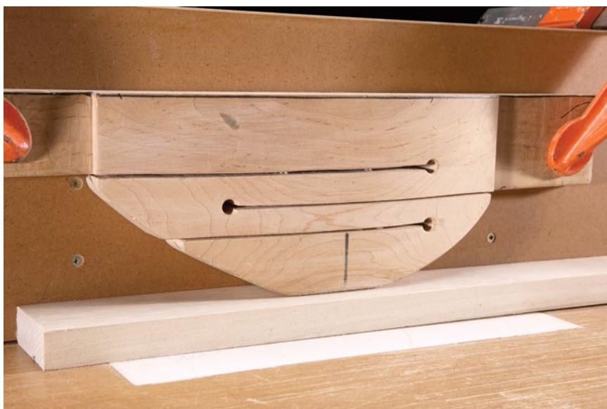
Spring-type guard. The beauty of this shop-made device is that it performs two essential functions on a router table: It holds the work down and denies your fingers access to the spinning cutters.
