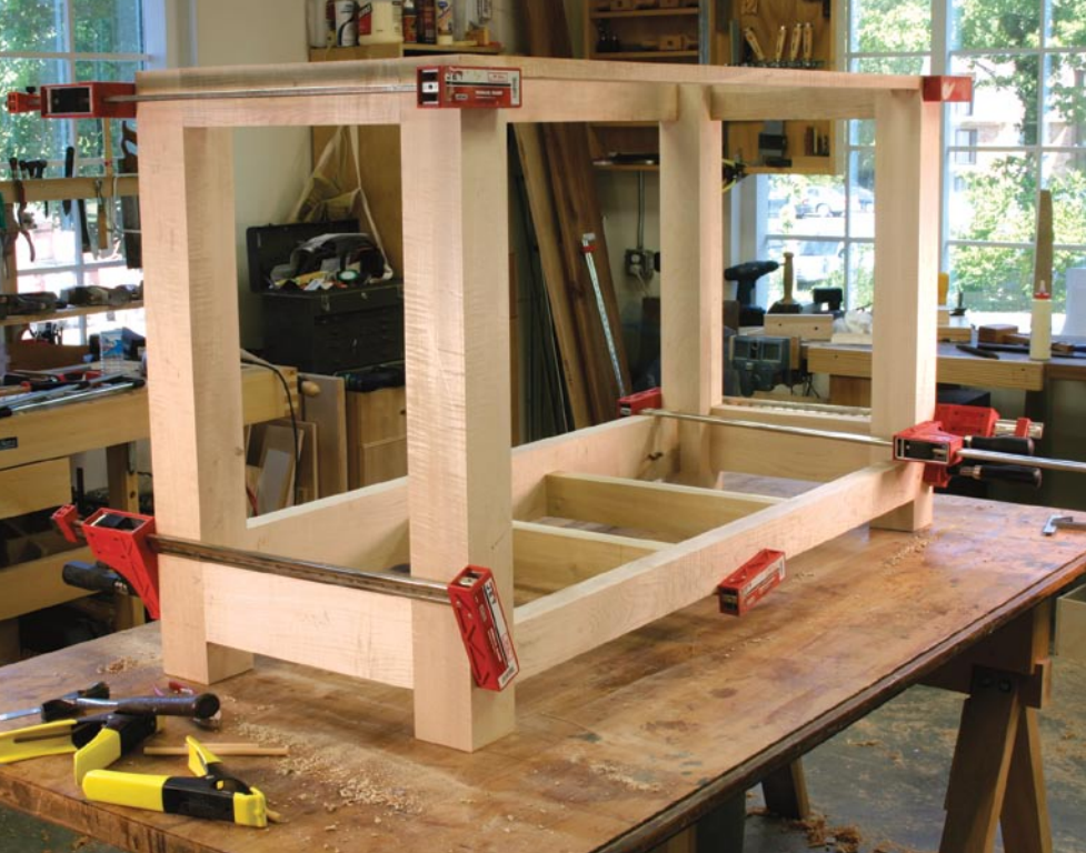
Standing strong and sturdy. All the rails are fit to the legs with mortise-and-tenon joinery. It's possible to simply add a benchtop at this point to have a well-built woodworking bench.
