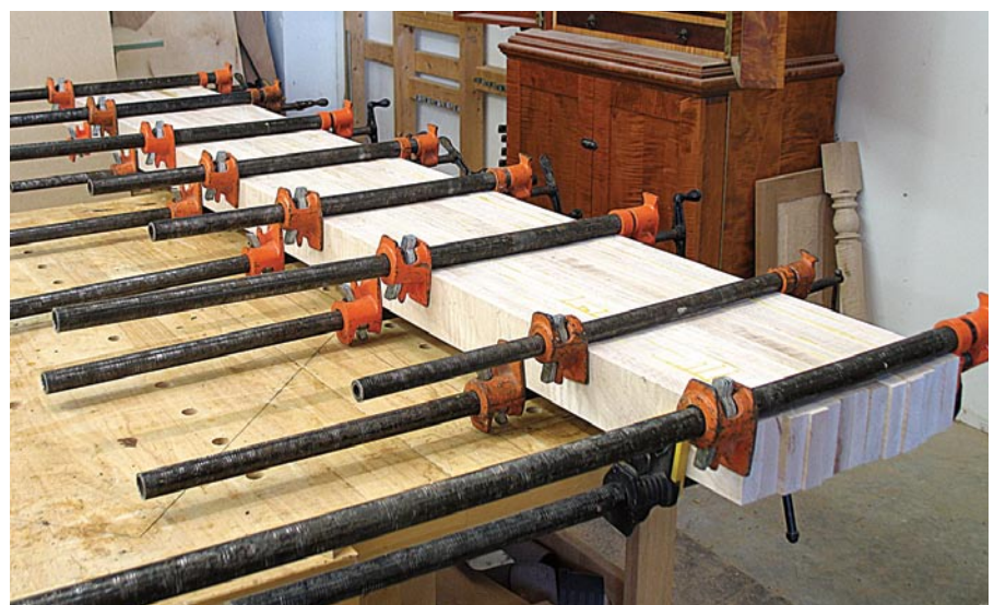
Counting pieces. The top was laminated from 32 pieces of lumber. Work in stages, please. Trying to laminate all the pieces at once will be a glue-filled mess.
