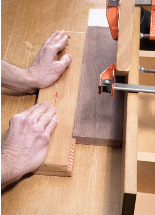
Twice as pushy. Good push sticks for the router table can be used vertically or horizontally on the table. Note how the hook helps push the work through the cut with no danger to your fingers.
