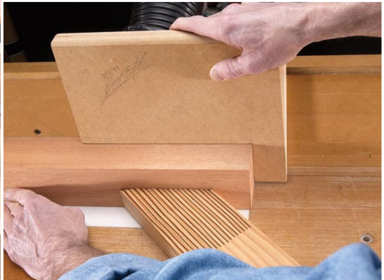
Twice as pushy. Good push sticks for the router table can be used vertically or horizontally on the table. Note how the hook helps push the work through the cut with no danger to your fingers.
