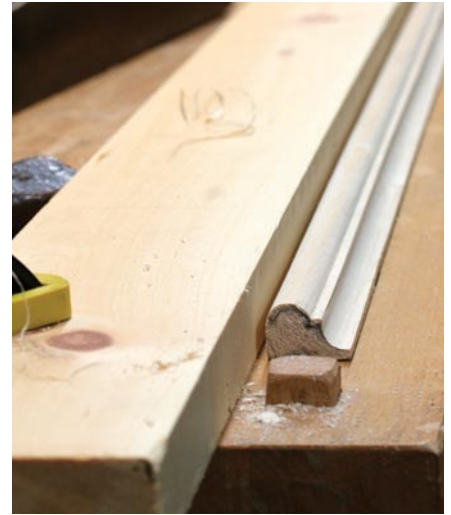
Uniformity is overrated. The finished moulding is not perfectly uniform from end to end. But it won't matter as long as I cut it into pieces and wrap them around the desk in order.
