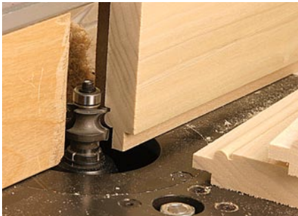
Routing a bead detail. The bead detail is placed on the tongue portion of the joint. Cutting the profile on the groove would weaken the joint considerably.
