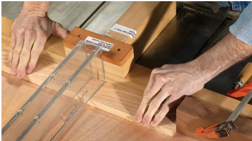
Proper crosscutting. Don't use the rip fence as a stop block for crosscutting. The better way to make repetitive crosscuts on a table saw is with a sled and a double-clamped stop block.
