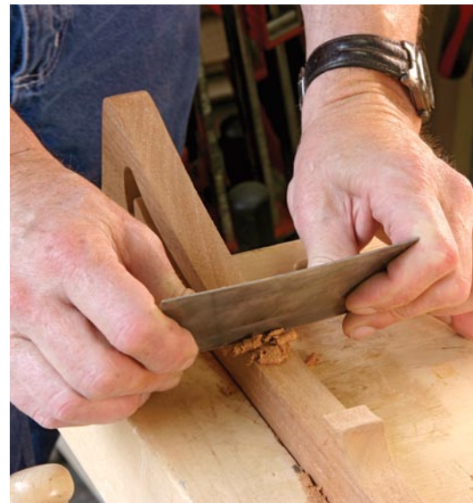
A close scrape. The hand-stitched rasp will leave shallow, narrow grooves. A cabinet scraper follows the rasp to remove the high spots between the grooves and leaves a fine surface.
