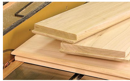
Drawer work begins. The table saw allows you to fine-tune the fit of the drawer. Measurements for other drawer parts are based off the inside face of the drawer fronts.
