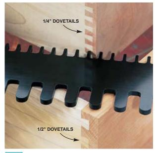
Make two sizes of dovetails with a double-sided template. All the jigs offer a smaller template as an accessory, but it's standard equipment on the Craftsman shown here.
