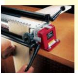
Quick-action board clamps let you move lumber through this jig at a rapid rate. The clamps are as stout as the rest of the jig, which looks like it can take years of hard use.
