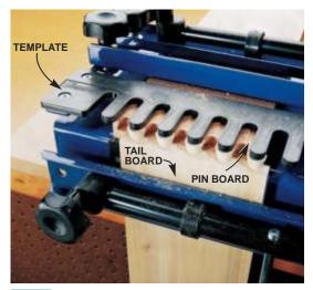
Cut both pins and tails in one pass on a half-blind dovetail jig, such as the Woodstock, shown here. Guided by the template, your router makes equally spaced dovetails.
