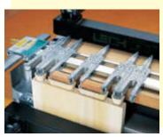
Customize the spacing of half-blind dovetails. That option is unique to the Leigh jig.
