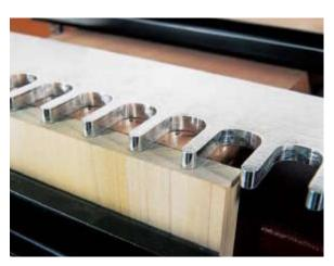
A rigid template makes it easier to align the pin and tail boards. You're more likely to get consistently accurate results with a rigid template (such as the Hart, shown here) than with one that bends slightly.
