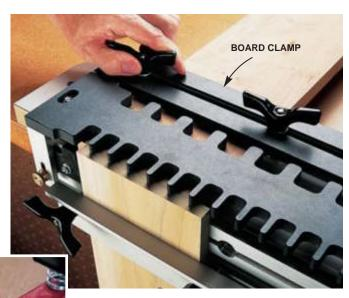
Adjustable stops allow you to fine-tune the width of the half-pin at the bottom of a dovetail joint. The stops on the Porter-Cable jig shown here are easily accessible.
