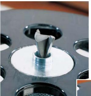
You'll need a specific-diameter guide to follow the template of a half-blind dovetail jig (see Chart, page 70). Woodworking catalogs offer template guides for most fixed-base routers, but you may have to special-order yours from a dealer.
